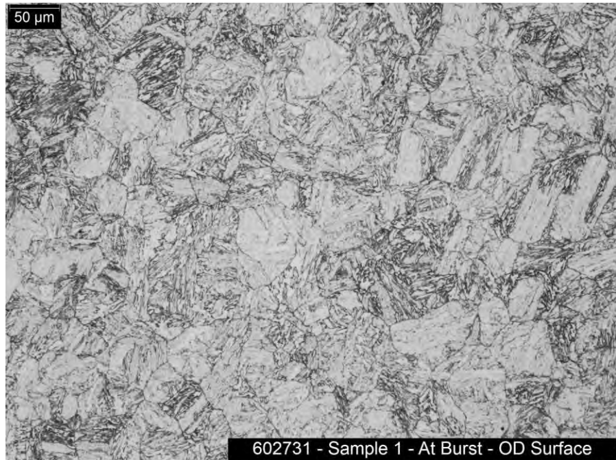
Figure 26: Sample 1 – Micro photograph of OD Surface cross-section at Burst, Grain Size No. 6
