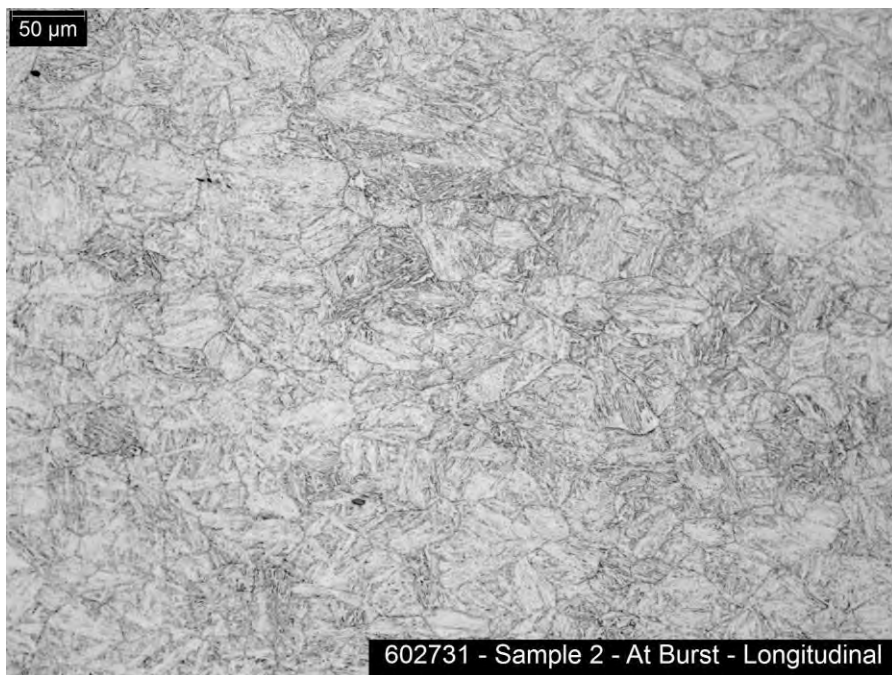
Figure 42: Sample 2 – Micro photograph of Longitudinal cross-section at Burst, Grain Size No. 7
