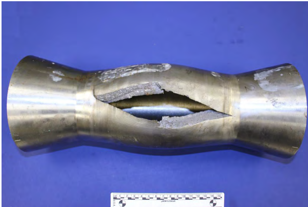
Figure 1: As Received Photograph – Sample 1 - Top View of Reduced Case at Burst (scale in mm)
