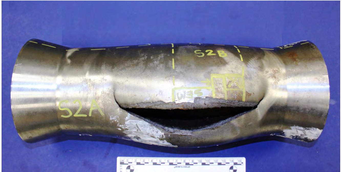
Figure 10: Layout Photograph – Sample 2 – Top View of Base Case at Burst (scale in mm)
