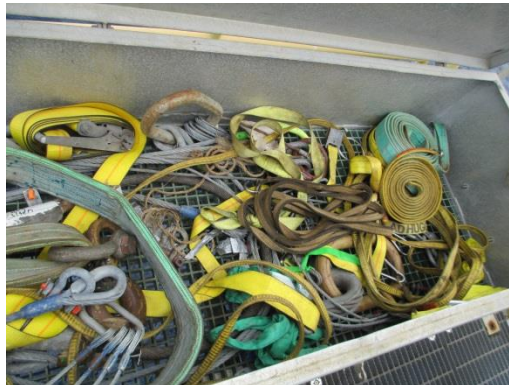
Abrasive wires contacting nylon straps in storage container
