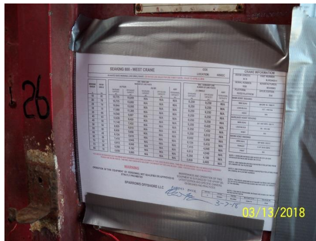
Load chart showing de-rating of crane 6 days prior to inspection
