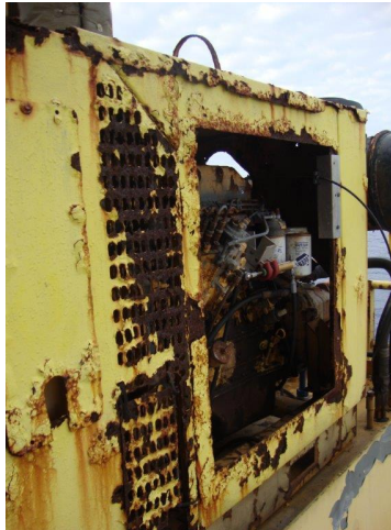
Severe corrosion on the engine covering
