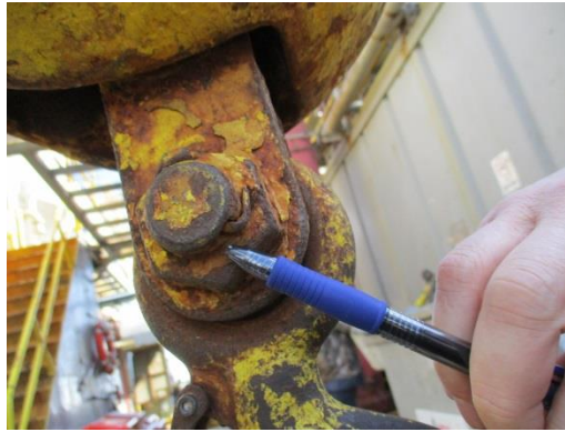
Failed cotter retaining pins on the auxiliary line overhaul balls of both gantry cranes
