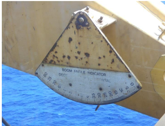
Numbers are faded on angle indicator
