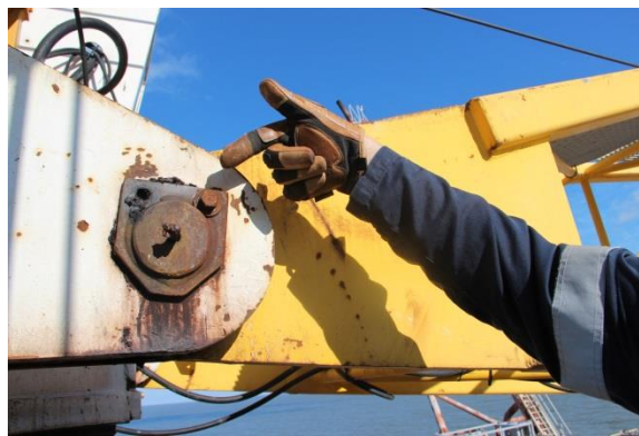
Bolt was missing from the boom heel section on platform crane
