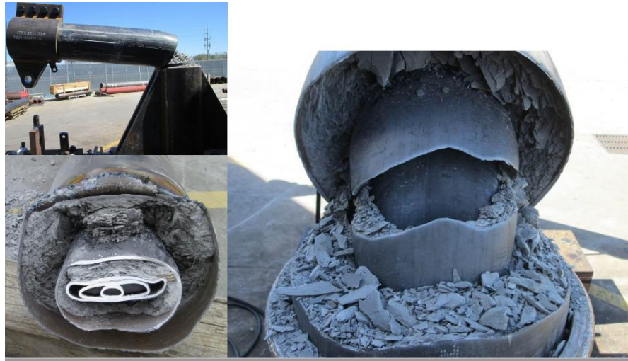
Figure 33. TEC Controlled 90 Degree Bend Test of Tubular
