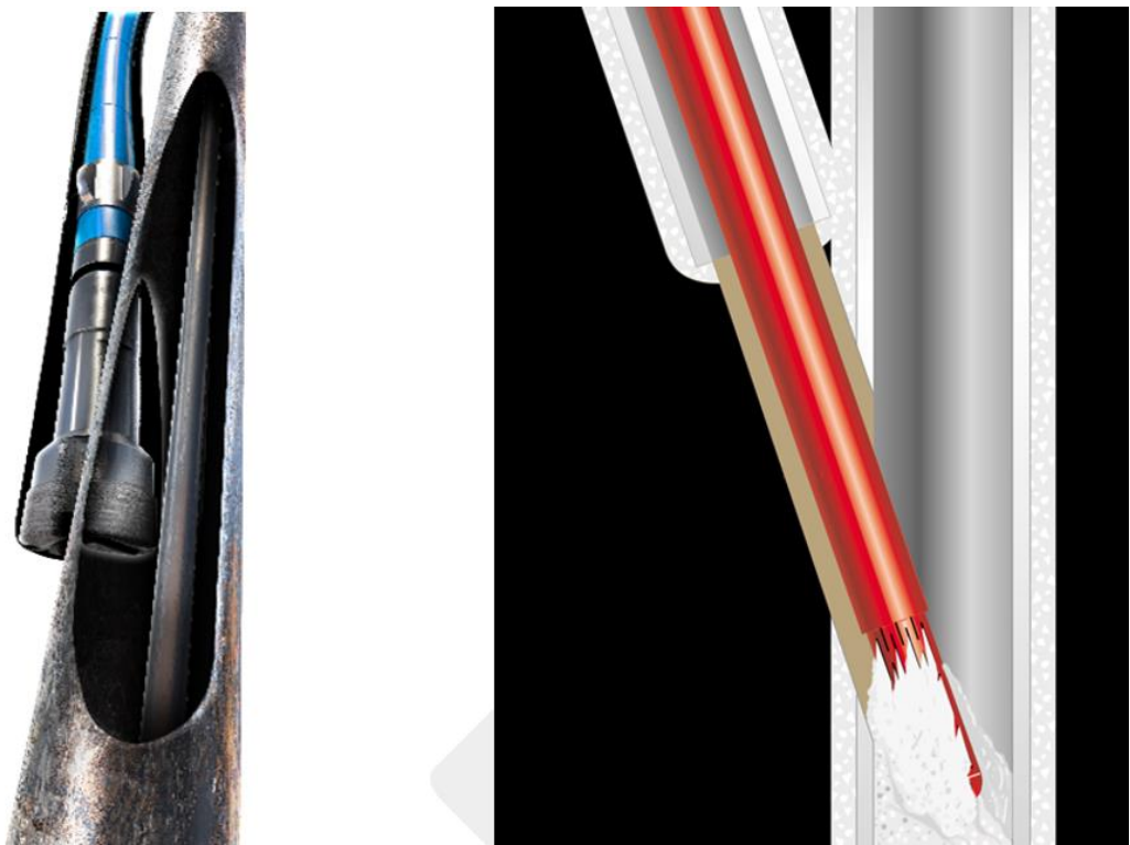
Figure 73. (Left) Milling into Target Well. (Right) Pumping Cement into the well to create an isolation plug
