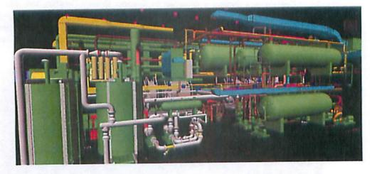
The recovered oil is either offloaded for recovery or sent to a flare system for burning. The recovered gas is burned in the flare system. Recovered sea water is purified and returned to the sea.
