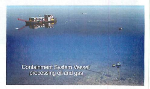
The Containment System starts with a specially designed containment dome that captures and directs the well leak fluids through separate oil and gas recovery hoses to the processing module equipment that is stationed on the barge.
