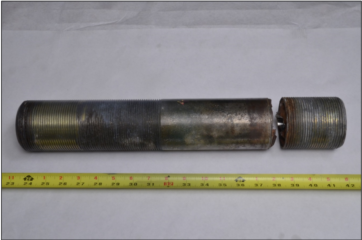
Figure 3: Hydraulic connector sheared fastener
