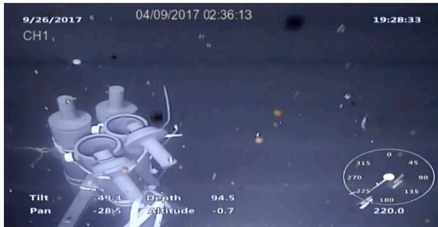
Fig. 26 Oil samples collection using Niskin bottle and robotic arms to release the lock-in mechanism.
