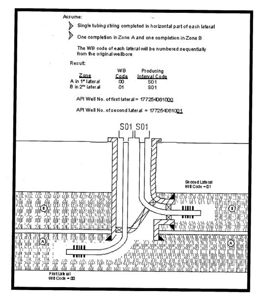
Note: Both laterals are open to production. The producing interval codes of S01 are unique to each wellbore segment.
