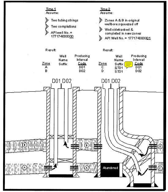
Note: Since a sidetrack creates a unique API Well No. all completions are assigned new producing interval codes independent of original wellbore.
