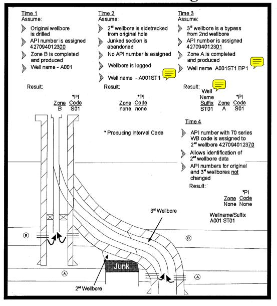
Note: Historical sidetracks, bypasses, well deepenings, etc., that were not initially assigned an API number can be assigned an API number with a 70 series WB code at a later time, so that any wellbore data can be identified. API numbers already assigned will not be changed.
