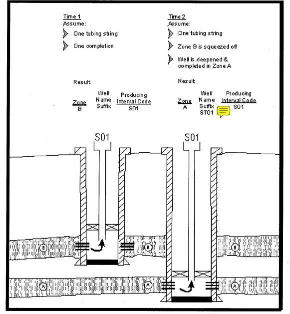
Note: In this example, the well is initially completed and later deepened and recompleted in another zone. The API number WB code is incremented to 01. The producing interval code remains S01.
