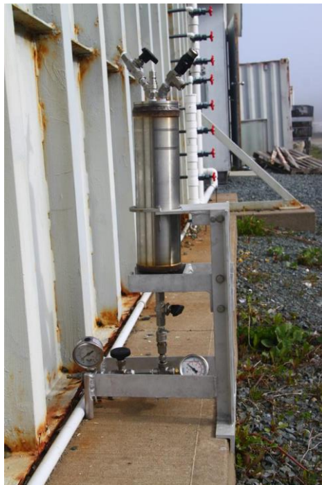
Figure 4A. Photo of the pressurized oil vessel used to hold the oil for the subsurface release.
