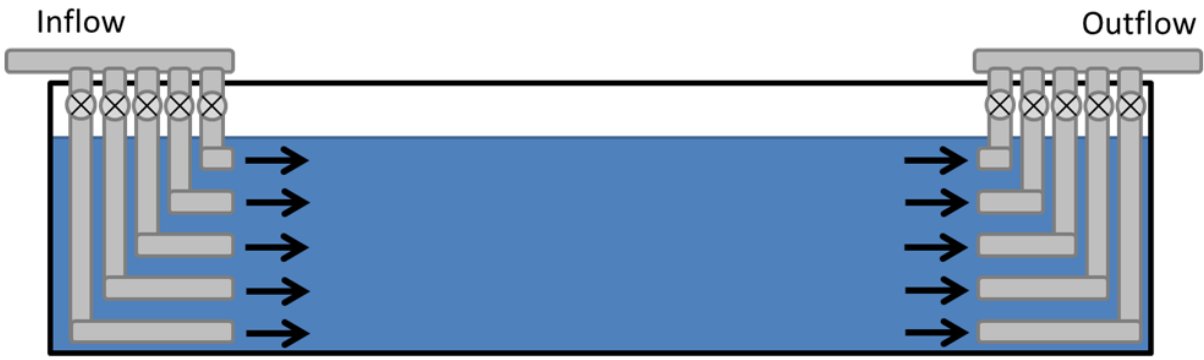
Figure 2. Photo of the DFO BIO flume tank (top) and cross-section of the tank showing the high-flow manifolds used to generate horizontal water currents (not to scale).
