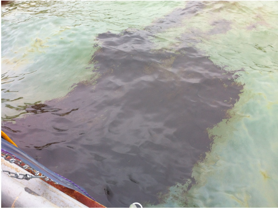
Figure 31. SLC oil being released in Ohmsett wave tank.
