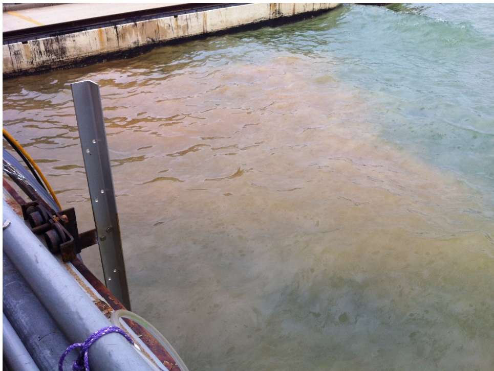
Figure 32. SLC oil being dispersed in Ohmsett wave tank.
