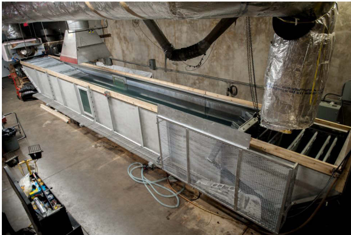
Figure 7-1 SL Ross Wave Tank
