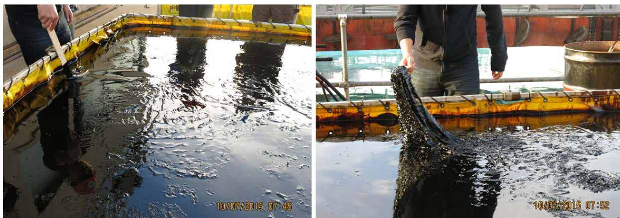
Figure 11. (a) The sheet-like ANS oil/i-Petrogel (3/1) adduct, (b) recovery of ANS oil/i-Petrogel sheet by a simple stick.
