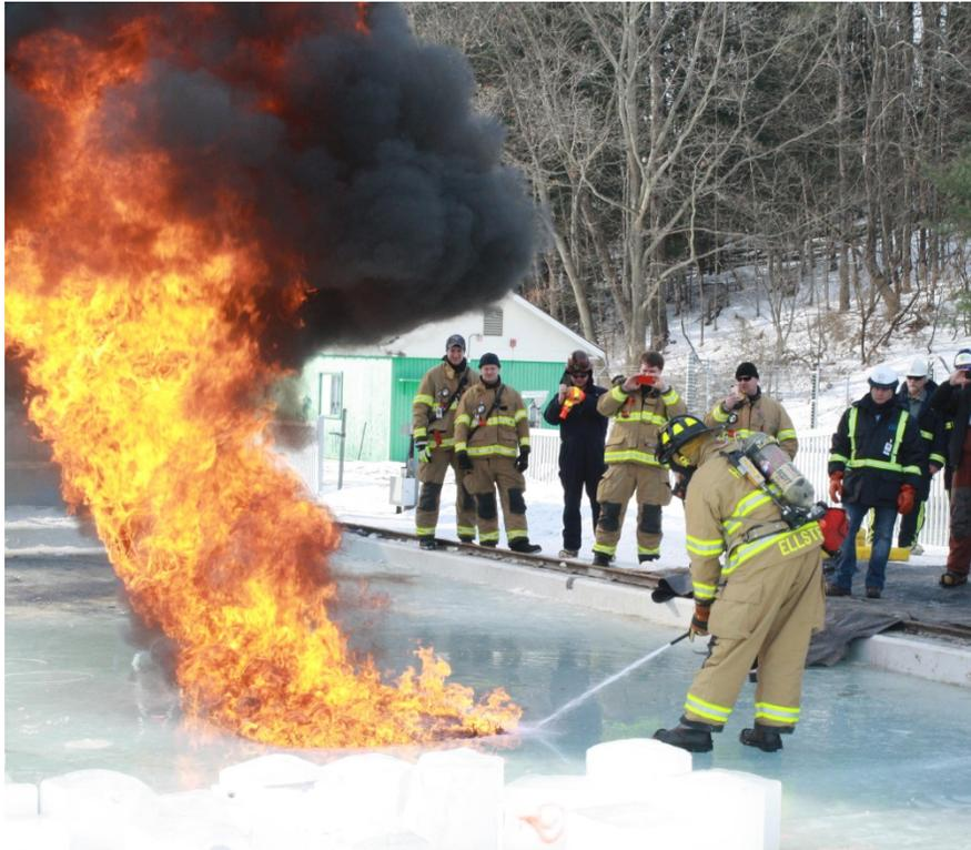
Figure 18. In-situ burning in ice at CRREL.
