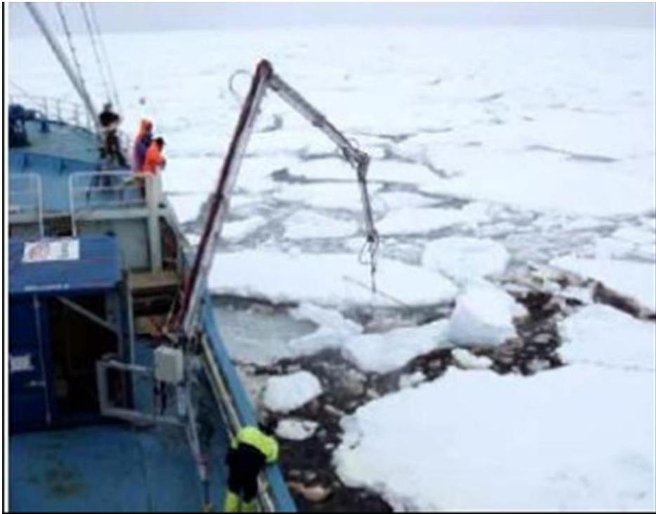
Figure 6 Dispersant application in dense pack ice: Barents Sea tests
