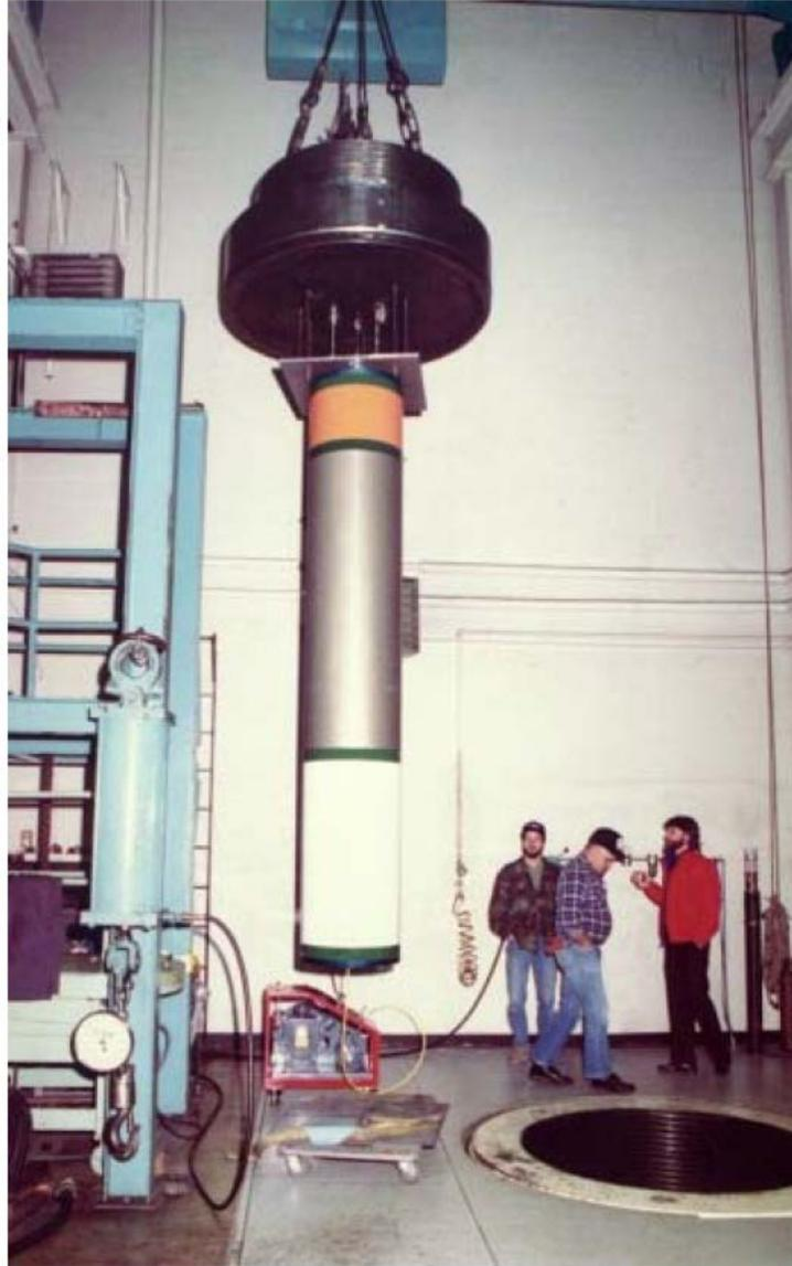
Figure 27. A vertical high pressure chamber at the Deep Ocean Test Facility.
