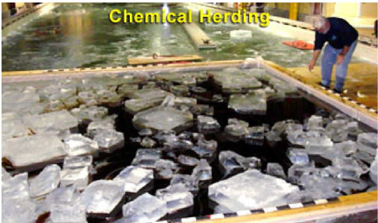
Figure 17. Testing of chemical herding agents at CRREL.
