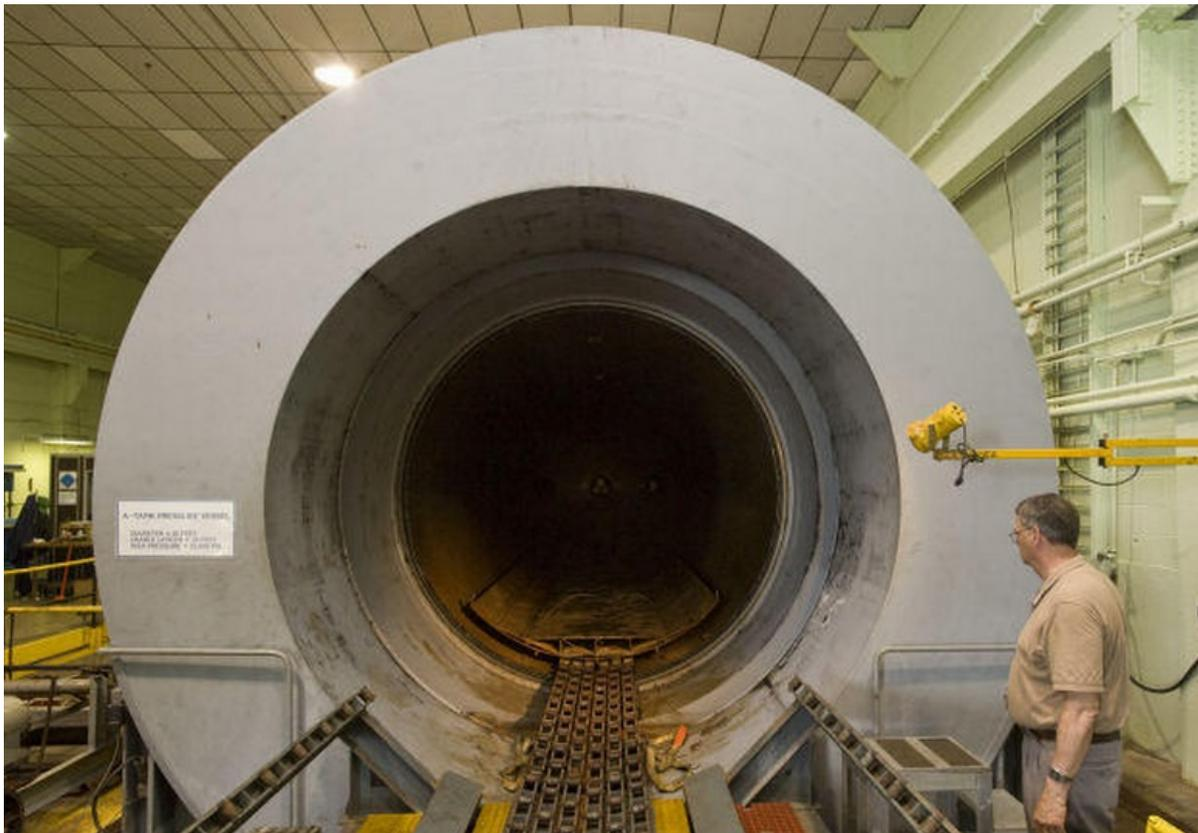
Figure 26. A horizontal high pressure chamber at the Deep Ocean Test Facility.
