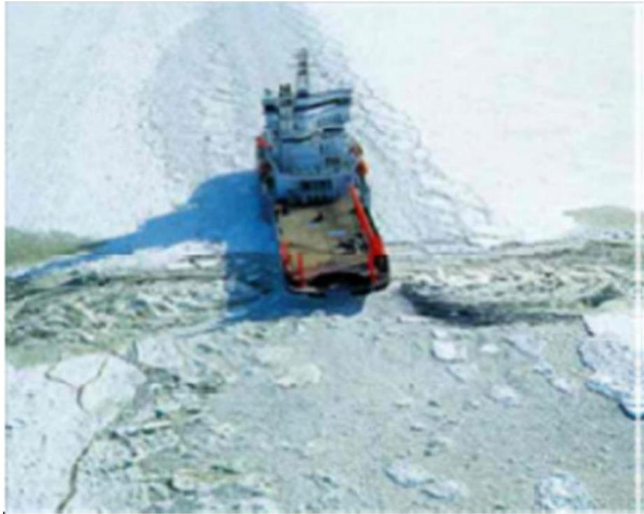
Figure 7 Use of ship's propeller wash to mix oil that has been treated with dispersant
