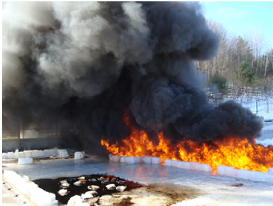
Figure 19. Burning of oil in a recovery trench in ice at CRREL.
