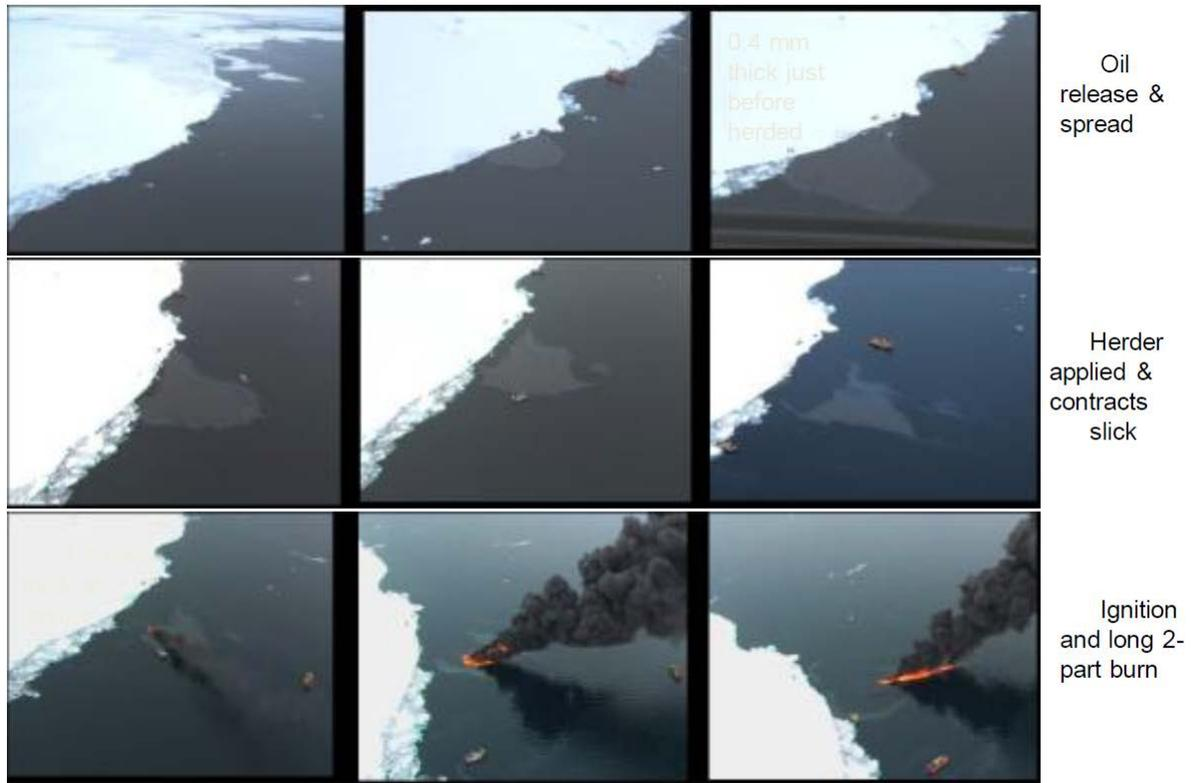
Figure 11. Full-scale field test of herding agents in drift ice in the Barents Sea
