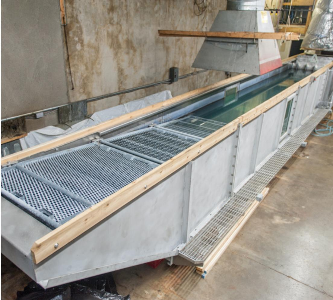
Figure 34. The wave tank at SL Ross.
