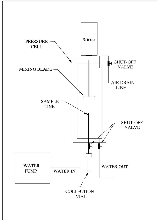
**Figure 9. Experimental design for the determination of dispersant effectiveness in water at elevated pressures.**
