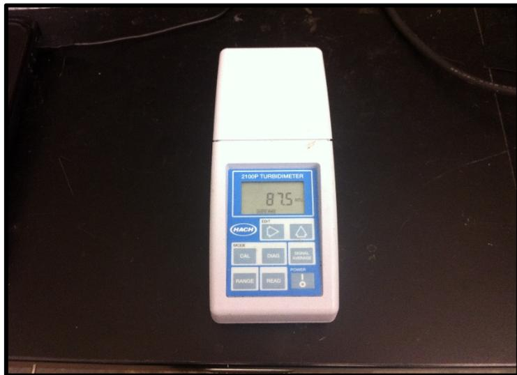
**Figure 1. Photographs of Aqualog spectrofluorometer (top), Turner Designs Cyclops-7 probe (mid), and Hach portable turbidimeter (bottom).**
