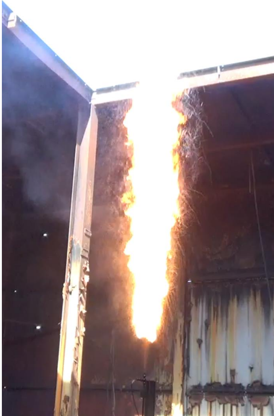
Fig. 50-Photograph of the burning spray plume operating with 3.0 g/s of 80:5:15% of CH 4 , C 2 H 6 , and C 3 H 8 and a blend of crude oils flowing at 16 g/s.
