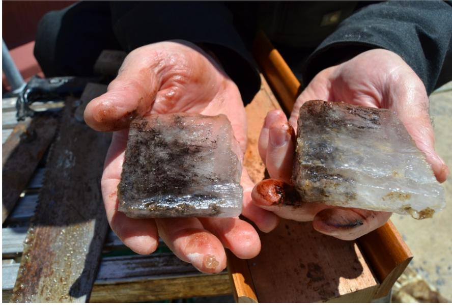
**Figure 4.15. Cross section of large ice core from 3B after 40 days of weathering.**
