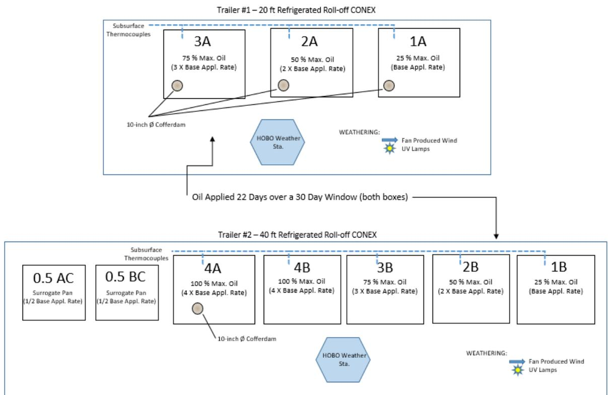
Figure 3.1. Layout of the ice samples and instrumentation in the refrigerated CONEX boxes.
