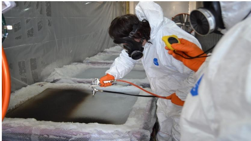
**Figure 4.2. Loading metered and timed application of oil to a target ice block.**
