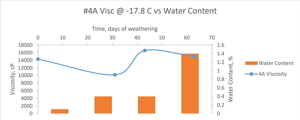
Figure 5.6 Block 4A Viscosity vs Water Content at -17.8°C
