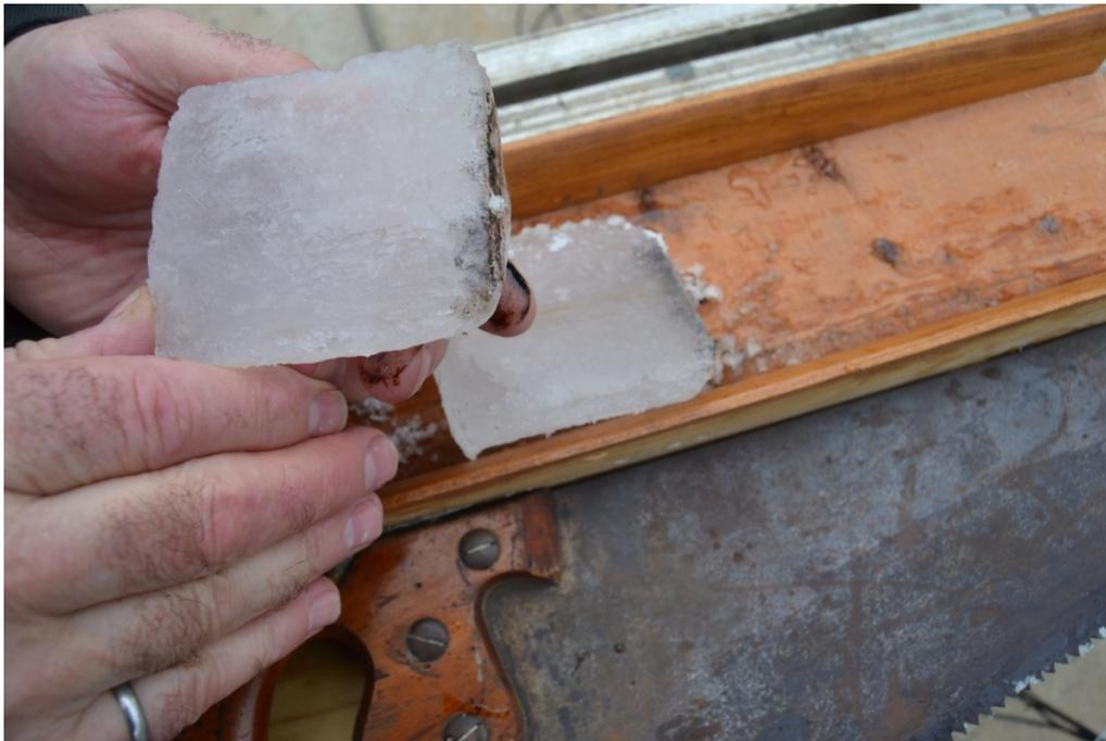
**Figure 4.6.** Cross section of large ice core from 2A following the application phase.
