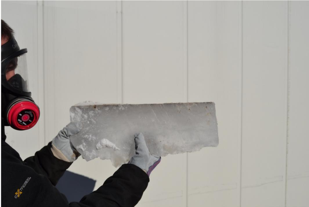
Figure 4.11. Upper layer of ice from 3A with slight oil migration following 33 days of weathering.
