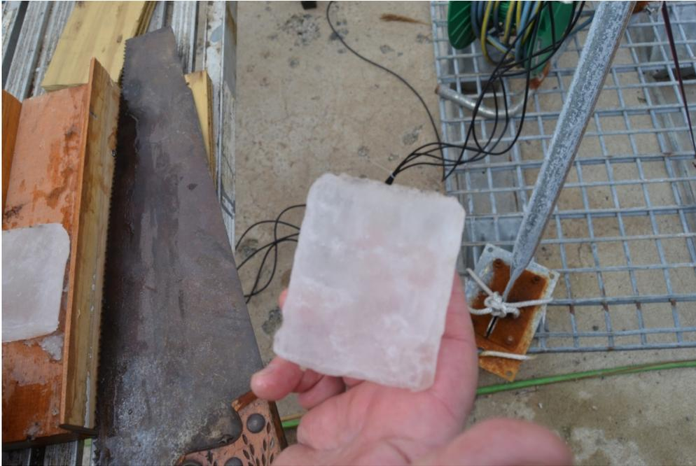
**Figure 4.7. Cross section of large ice core from 3A following the application phase.**
