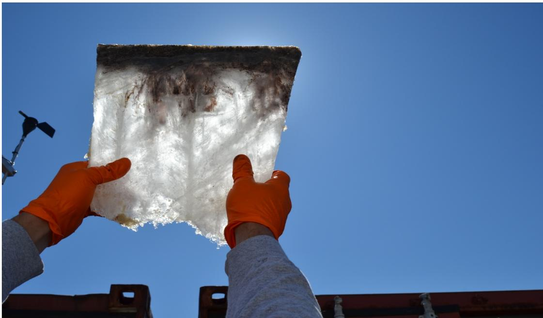
**Figure 4.18. Cross section slab of 4B with oil migration following 60 days of weathering.**
