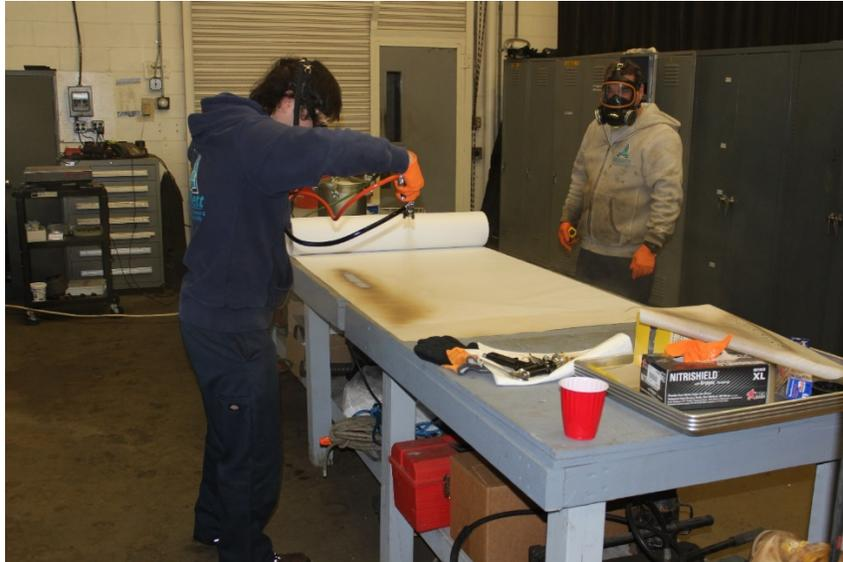
**Figure 4.1. Paper spray application test to establish operational parameters and technique for reproducible loading.**
