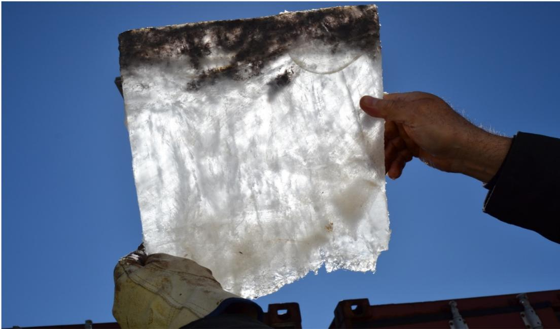
**Figure 4.17. Cross section slab of 3B with oil migration following 60 days of weathering.**
