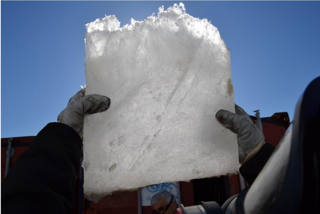
**Figure 4.9.** Cross section slab of ice from 1A with the skeleton layer at the top of the photo and the ice surface on the bottom. There is no evidence of oil migration after 33 days of weathering.
