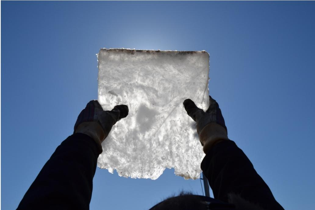
**Figure 4.13. Cross section slab of ice from 1B with the ice surface at the top of the photo with slight oil migration.**
