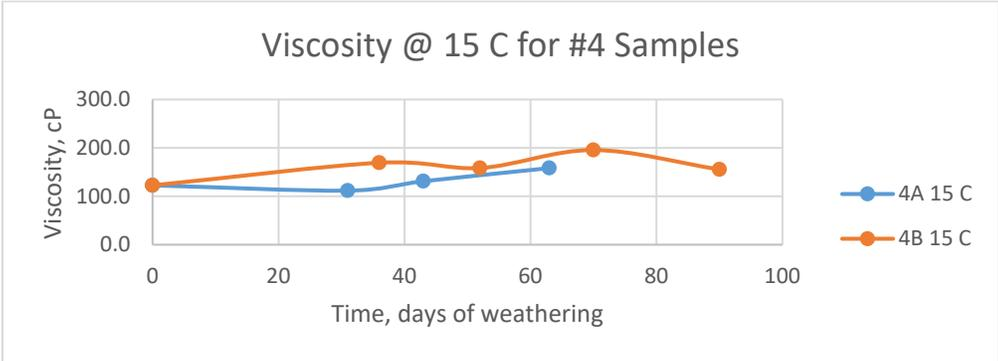
Figure 5.4 Replicates 4 Viscosity Change of Time at 15 °C
