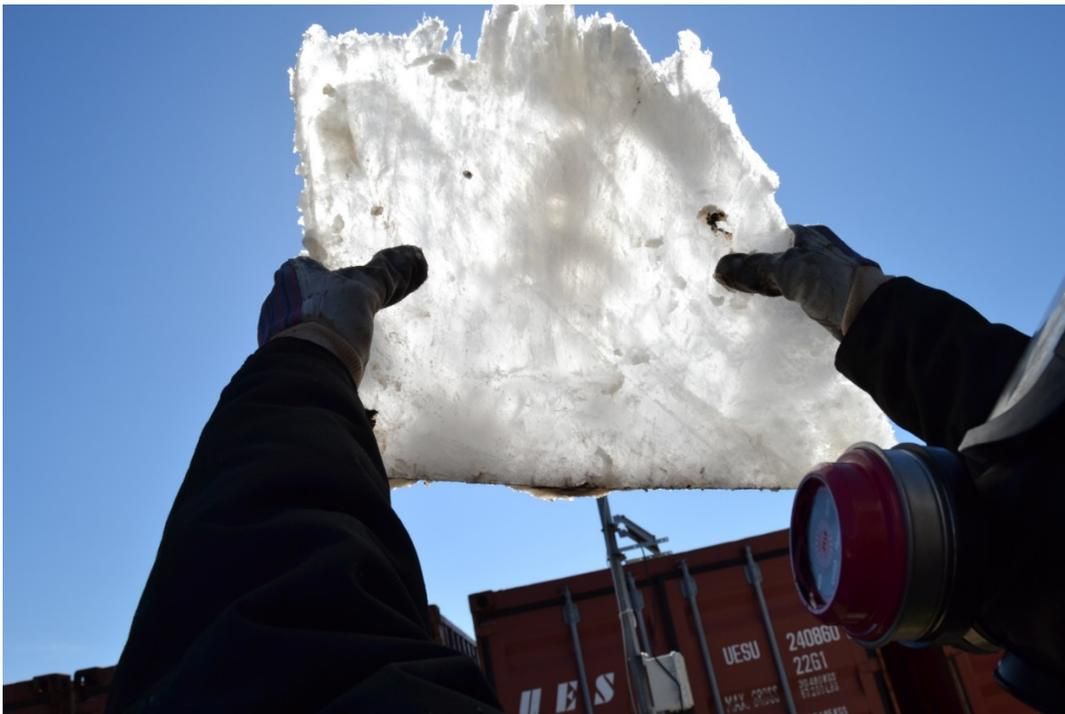
Figure 4.12. Cross section slab of ice from 4A with the ice surface on the bottom of the photo showing slight oil penetration following 33 days of weathering.
