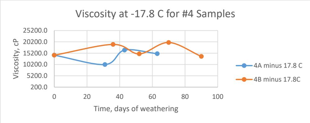
Figure 5.5 Replicates 4 Viscosity Change of Time at -17.8 °C
