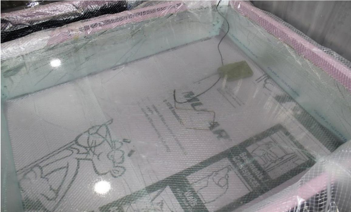
**Figure 3.2. Insulated box with plastic liner used as an ice form with a thermocouple to monitor the interior temperature of the ice.**
