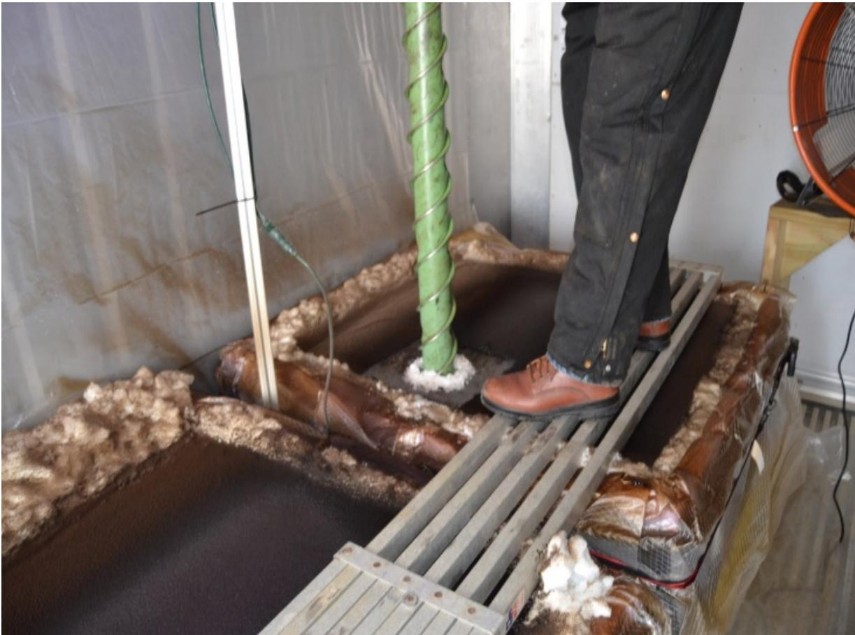
**Figure 4.4. Obtaining a 7.5 cm large core from sample 1A. Table 4.1. Oil Application, Ice Coring and Daylight Schedule**
