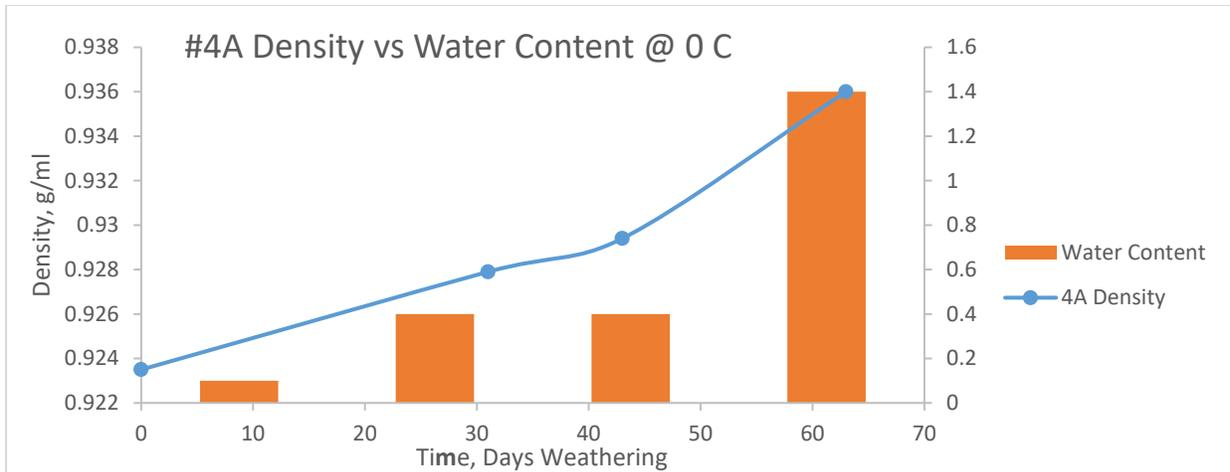
Figure 5.2 Block 4A Change in Density in Relation to Water Content
