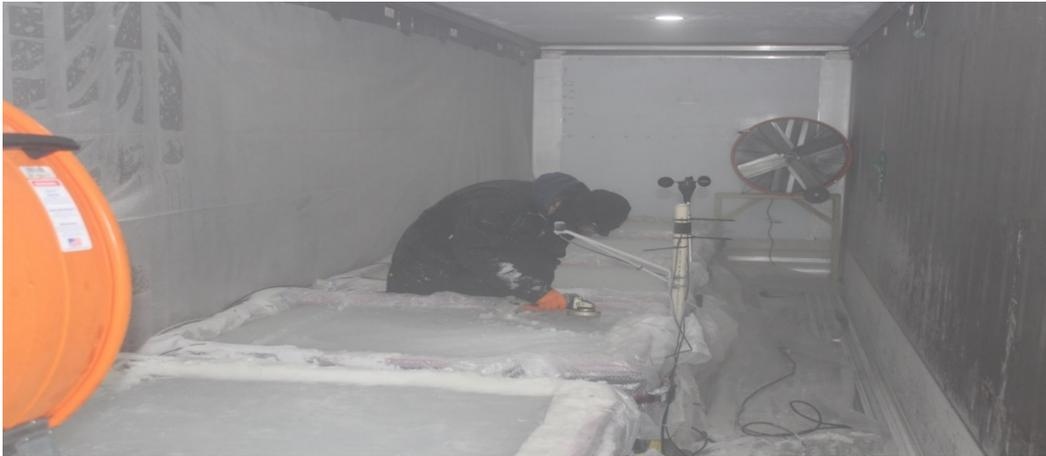
**Figure 3.3. Machining the 1m x1m test area in the 40-foot CONEX box with circulation fans and sensors.**
