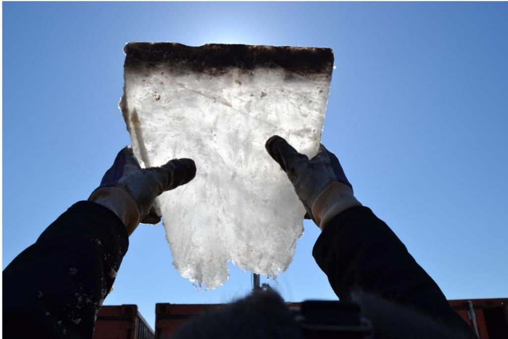
**Figure 4.14. Cross section slab of 2B with oil migration following 30 days of weathering.**
