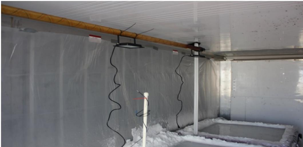
**Figure 3.4. Positioning of UV light sources for provide solar irradiation of the ice targets.**
