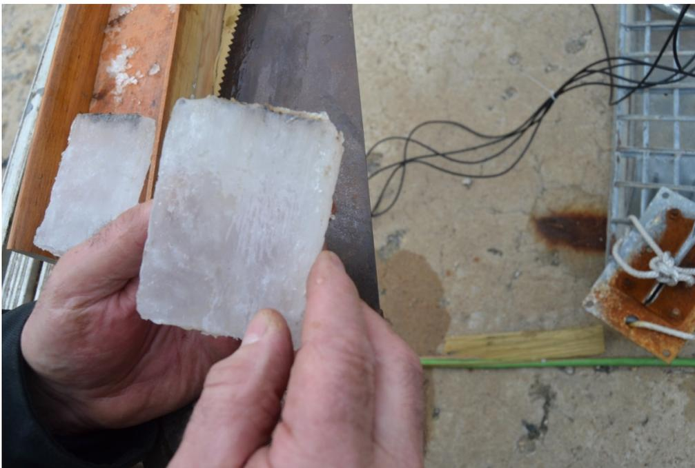
**Figure 4.8. Cross section of large ice core from 4A following the application phase.**
