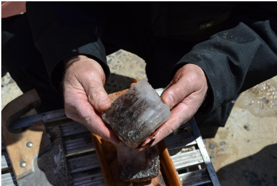
**Figure 4.16. Cross section of large ice core from 4B after 40 days of weathering.**
