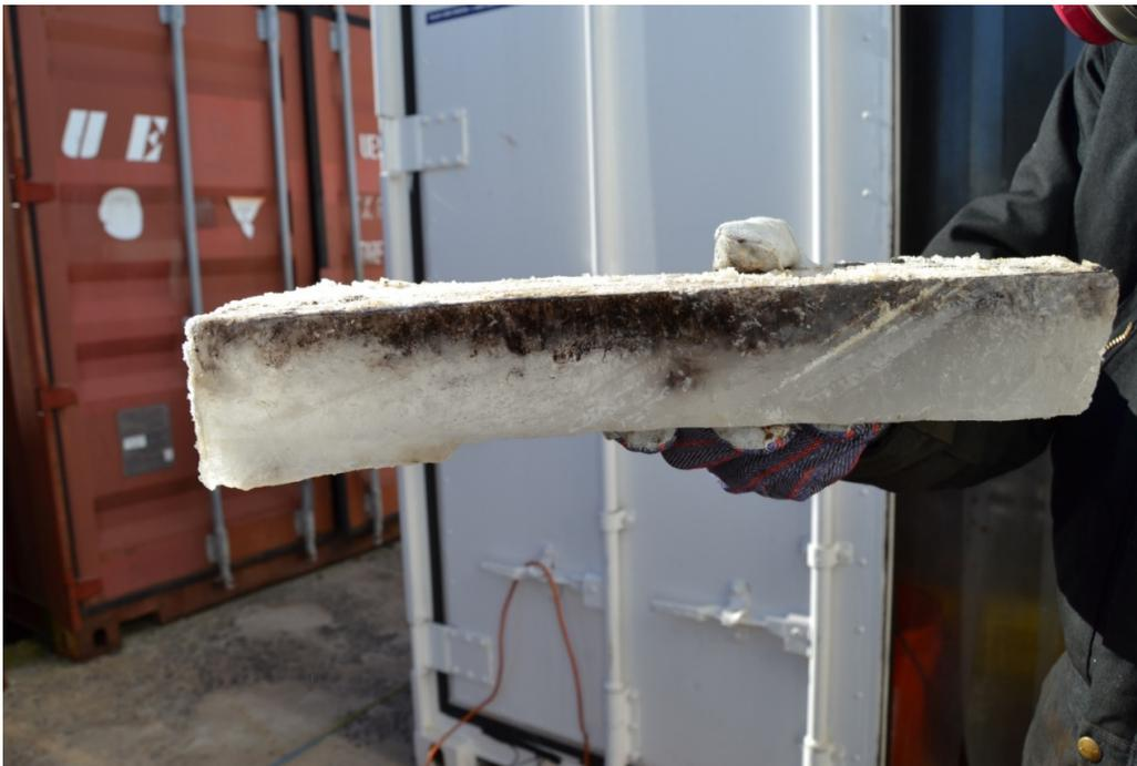
**Figure 4.10.** Upper layer of ice from 2A showing oil migration following 33 days of weathering.
