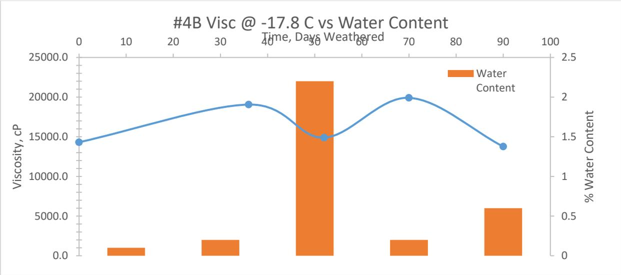
Figure 5.7 Block 4B Viscosity vs Water Content at -17.8 °C
