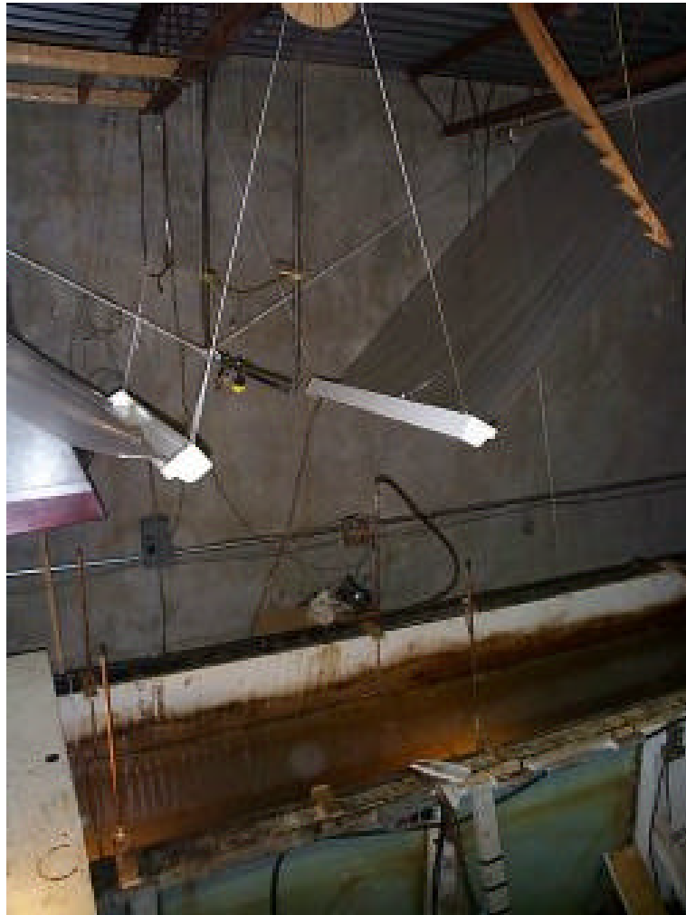
Figure 3 : Dispersant Spray Boom
