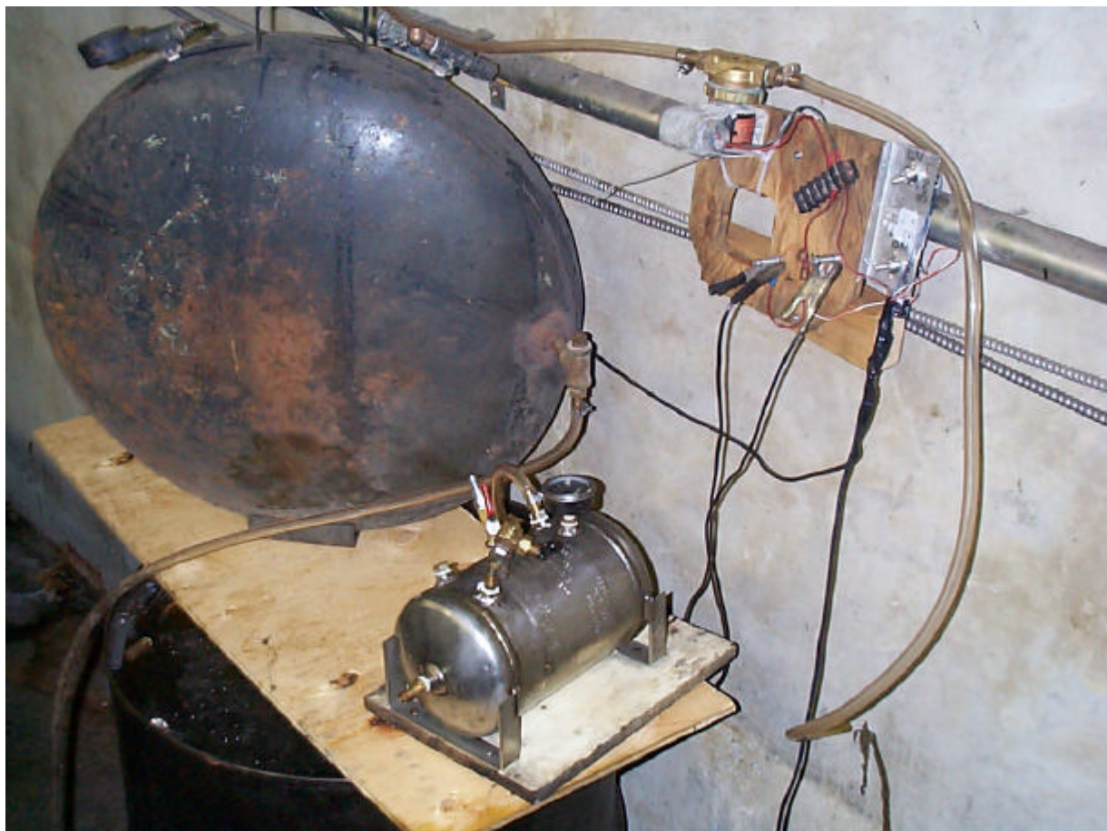
Figure 4: Dispersant Spray Pressure Tanks & Valve
