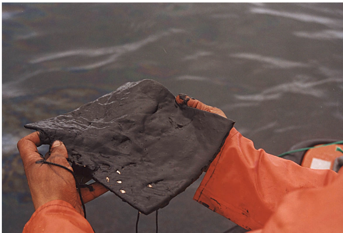
Fig. 8.2.4 Oil film thickness measurements using PP pad (on thicker emulsion). Crude oil experiment June 29.
