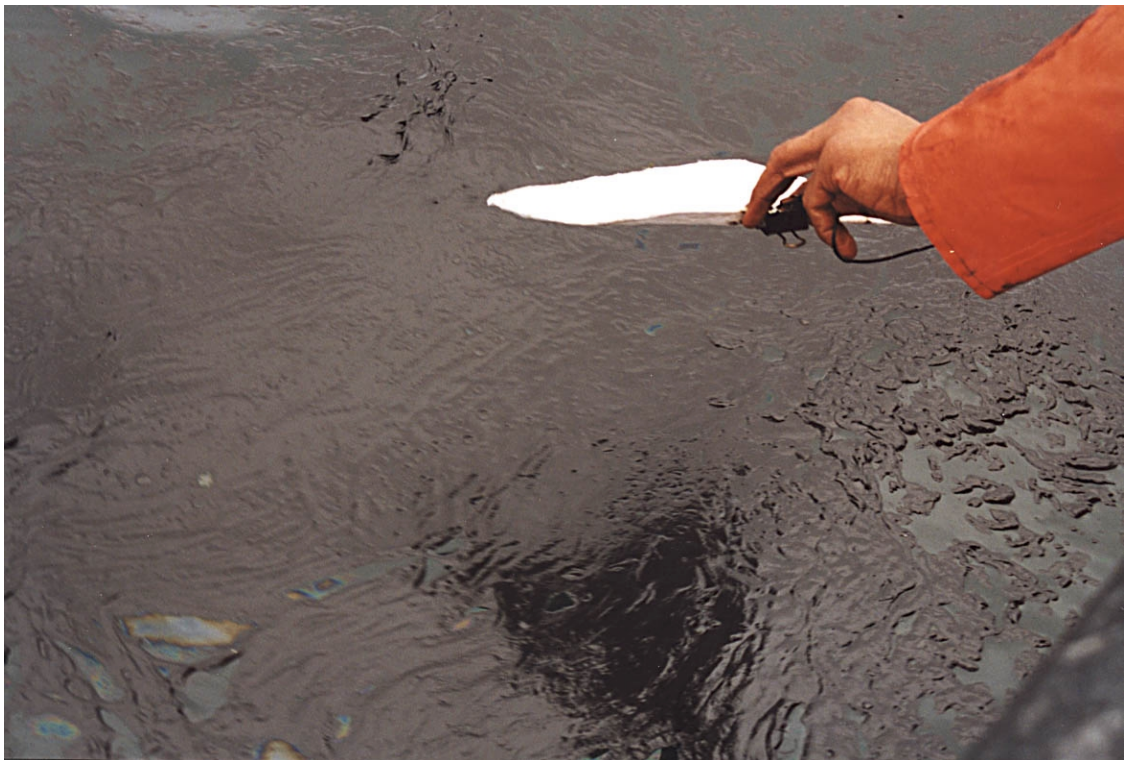
Fig. 8.2.2 Oil film thickness measurements using PP pad (on thicker emulsion). Crude oil experiment June 29.
