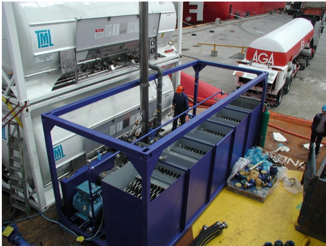
Figure 4.8 Far Grip in Tananger. Sea fastening of LIN and LNG tanks with pump unit and evaporator.
