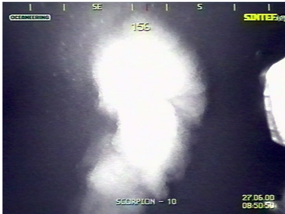
Figure 7.1.6. Further development of the diesel and methane plume. Undulating or meandering plume.
