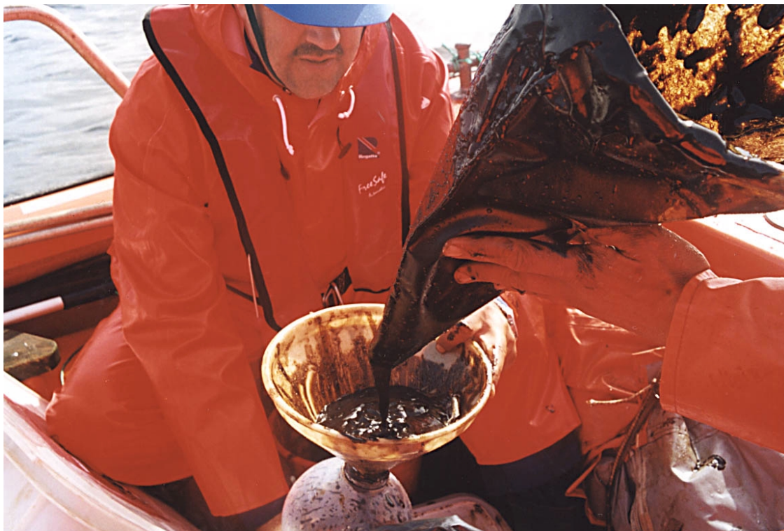
Fig. 8.2.7 Drainage of free water in emulsion sample by settling in separation funnels, June 29.
