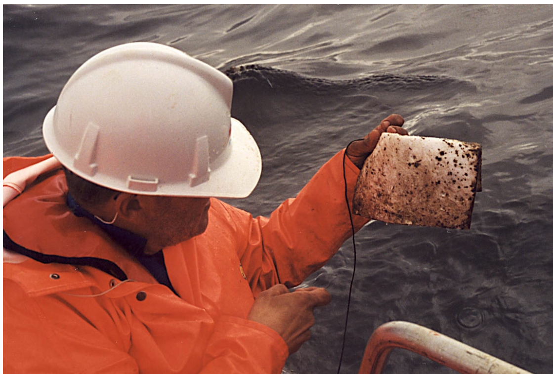
Fig. 8.2.5 Oil film thickness measurements using PP pad, on thinner oil film (metallic / discontinuous true oil colour)
