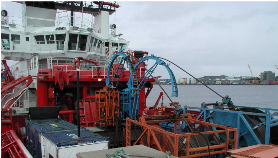
Figure 4.9 View of main deck on supply vessel Far Grip during mobilization at the ASCO base in Tananger. Reels with coiled steel tubing, goose necks and injector heads seen from the rear of the vessel.
