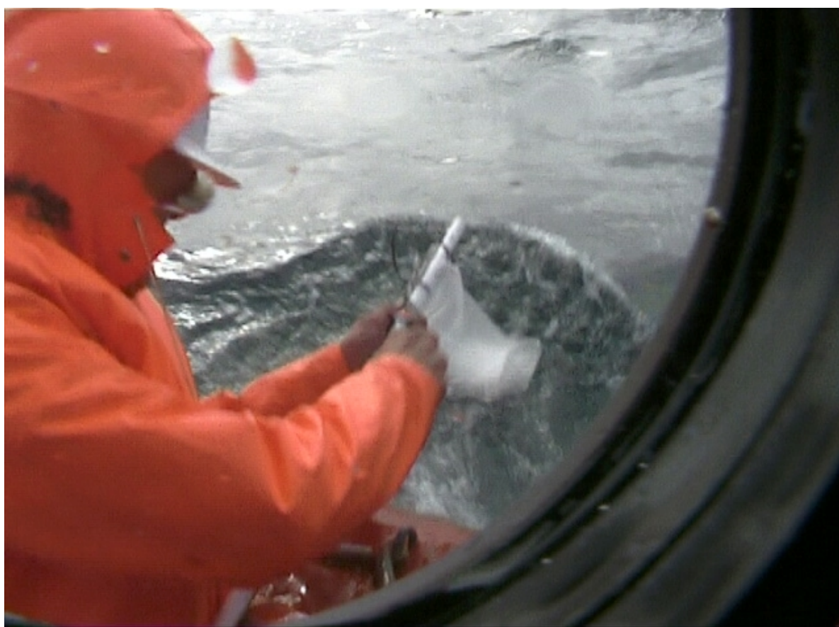
Figure 8.2.1 Teflon Net for thin oil film thickness measurements, of diesel film under “bad weather conditions
