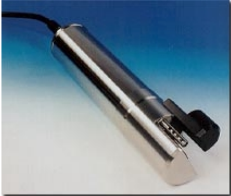
Figure 5.2. The UVAQUAtracka fluorimeter
