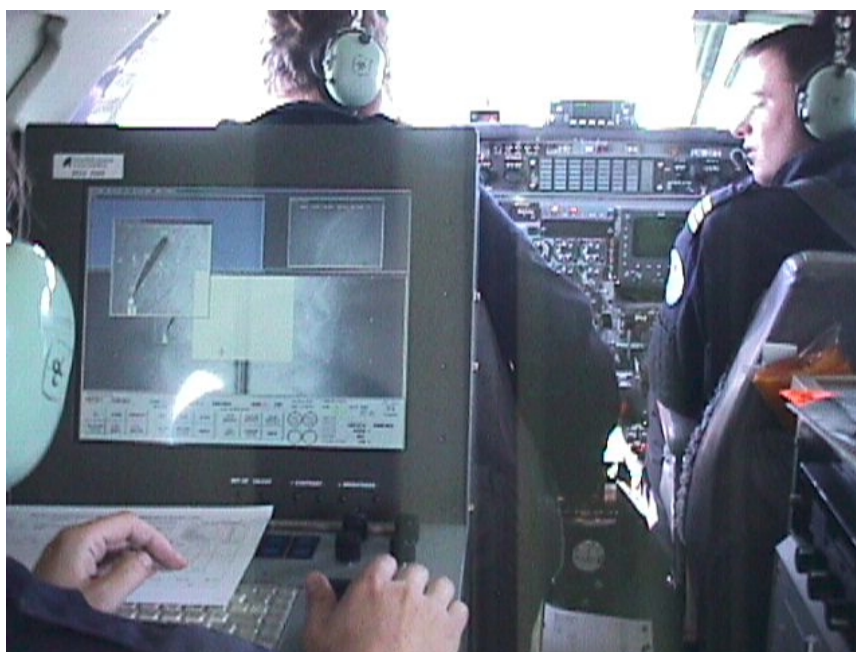
Figure 8.3.1 Inside SFT's surveillance aircraft. View of the SLAR radar image of the crude oil slick.
