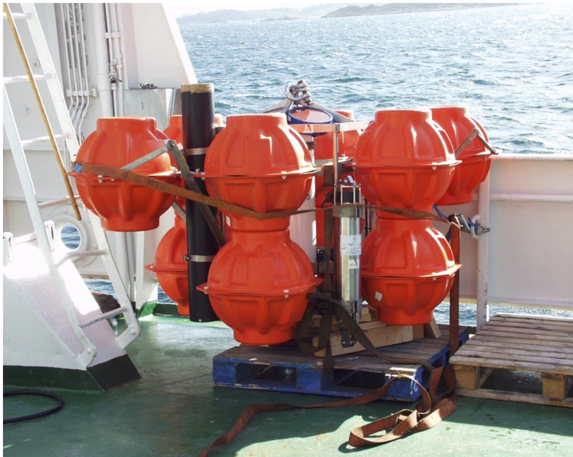
Figure 5.6 Picture of bottom mounted ADCP with buoyancy and acoustic release mechanism.
