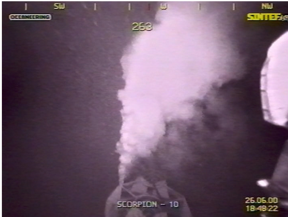
Figure 7.1.3. Well developed nitrogen plume.
