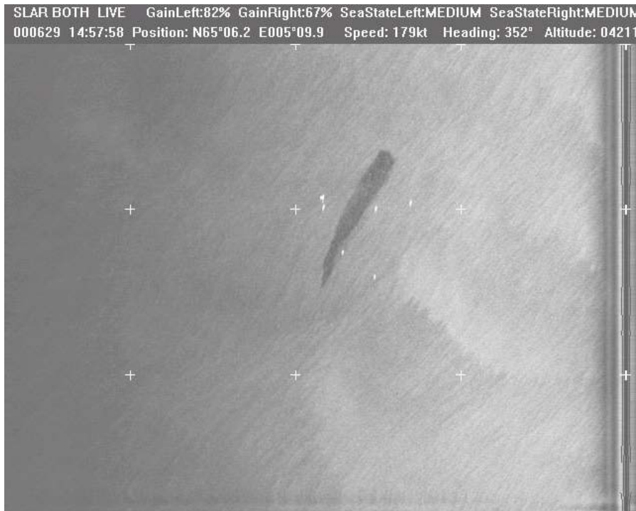
Figure 8.3.5 SLAR image from the Norwegian aircraft taken at June 29, 1358 UTC (note that the time stamp on the picture is Norwegian Standard Time – summer saving hour neglected). 10 km distance between markers. The text also contains the heading of the aircraft and a position – with reference to the marker at the top of the bar to the right in the image.
