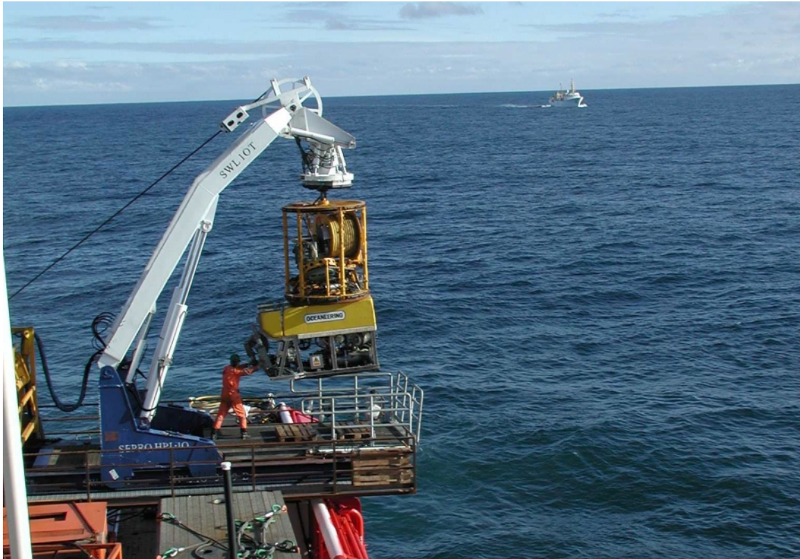
Figure 5.5 Work ROV launched from Far Grip in preparation for deployment operation. Research vessel Håkon Mosby seen in the background.
