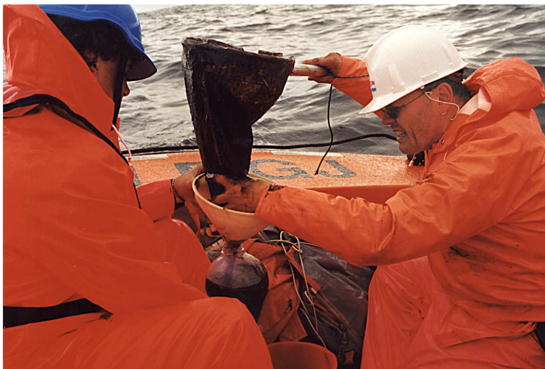
Fig. 8.2.6 Sampling of emulsions and drainage of free water by settling in separation funnels, June 29.
