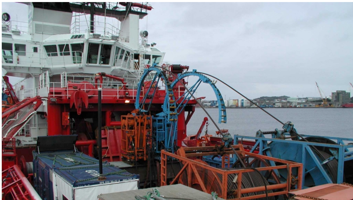
View of main deck on supply vessel Far Grip during mobilization at the ASCO base in Tananger. Reels with coiled steel tubing, goose necks and injector heads seen from the rear of the vessel.
