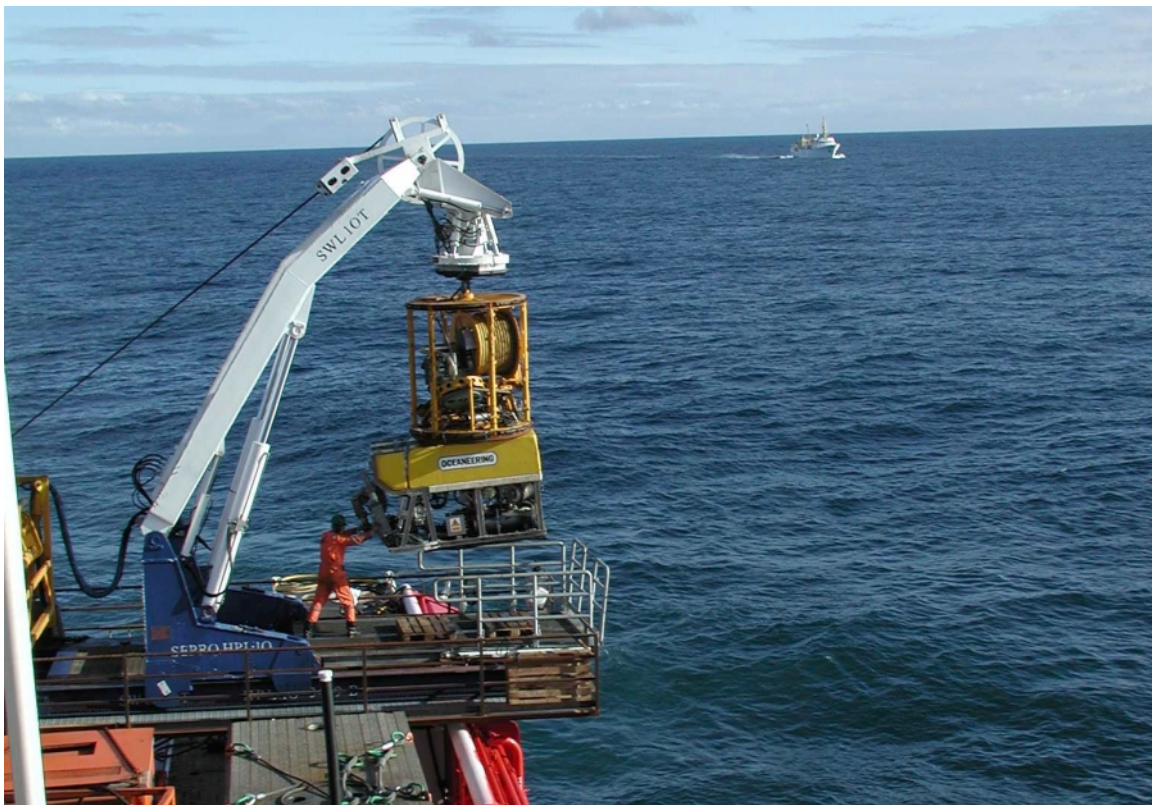
ROV launched from Far Grip in preparation for deployment operation. Research vessel Håkon Mosby seen in the background.
