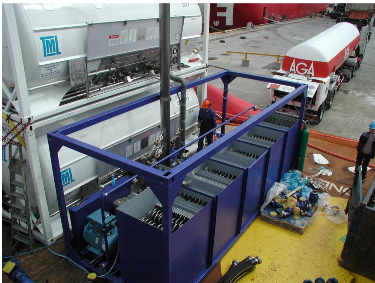
Far Grip in Tananger. Sea fastening of LIN and LNG tanks with pump unit and evaporator.
