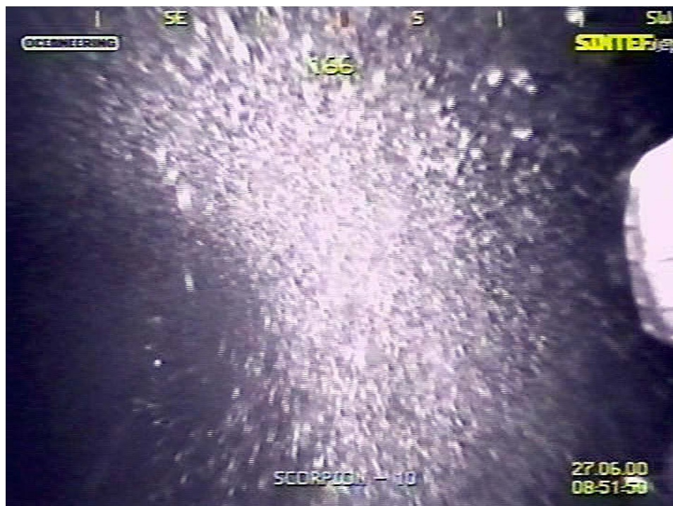
Figure 12.2. Picture identity 08-51-49. Methane and diesel release. Appearance of a gas and diesel cloud when entering into the plume. The separation between diesel droplets and gas bubbles is unclear.
