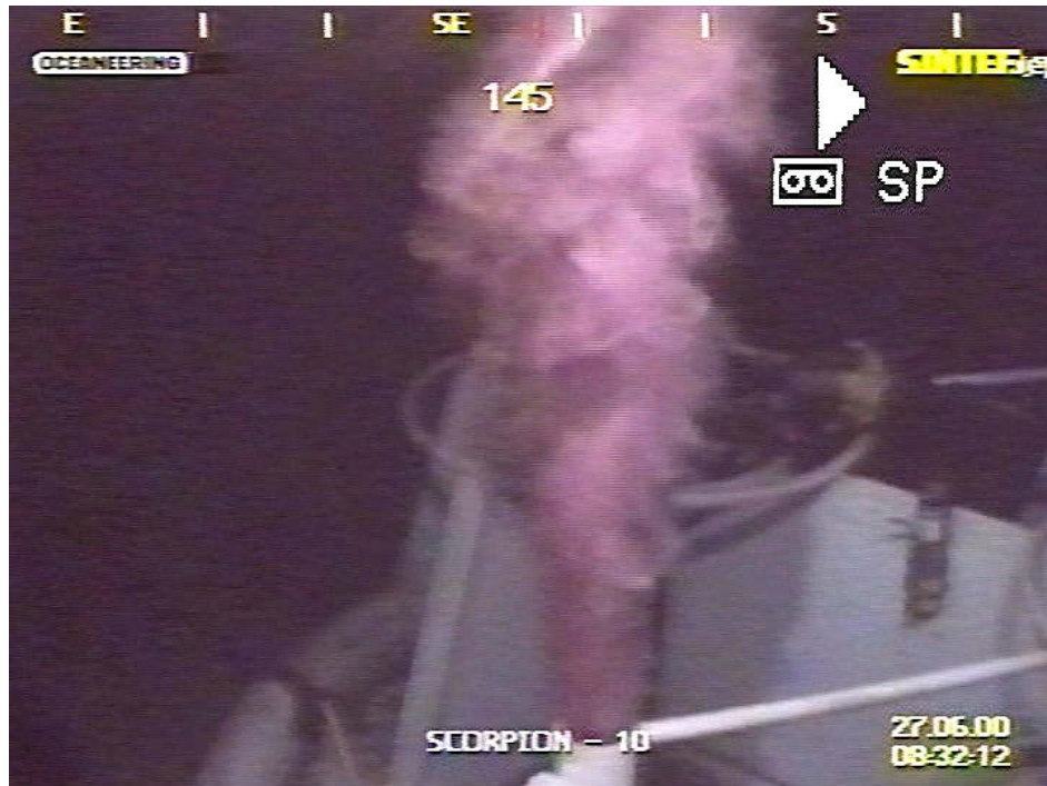
Figure 11.1. Picture identity 08-32-12. Release of water and nitrogen just prior to the diesel release.
