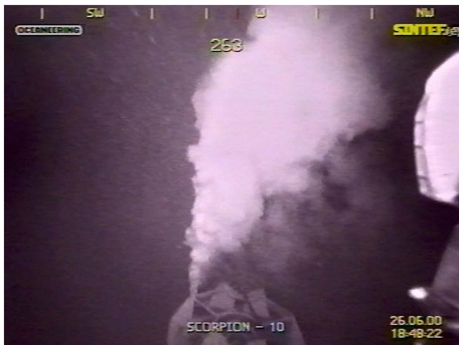
Figure 10.2. Picture identity 18-48-22. Well developed nitrogen plume. Some ambient currents are present directed to the right. Although not apparent in this picture, the video shows in this particular case a tendency for a separation of the plume, where the gas bubbles are moving upwards (to the left), and the water tends to move more slowly in the horizontal direction to the right (in the downstream direction).
