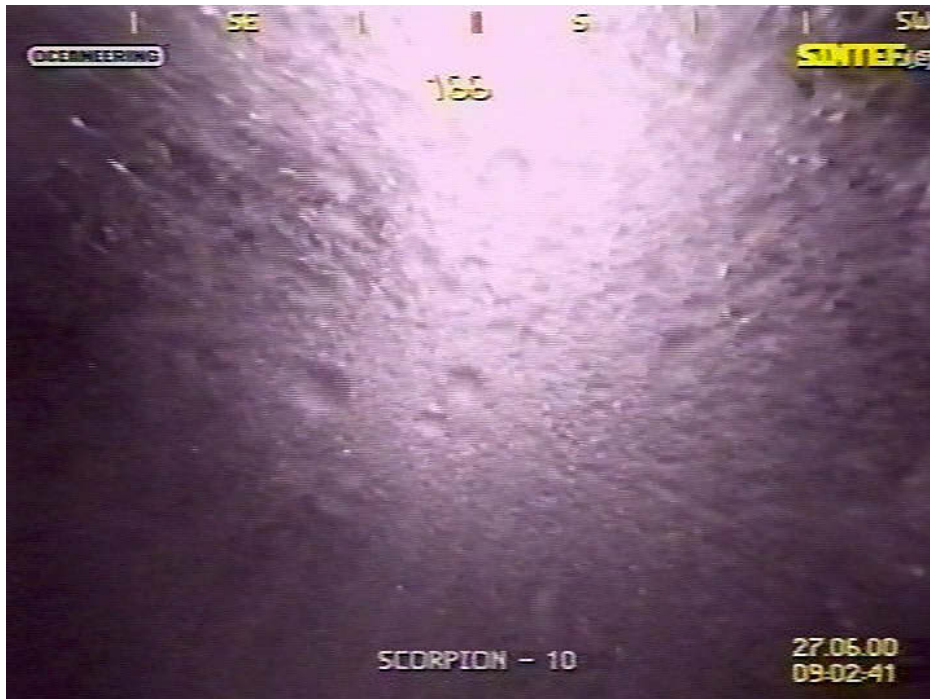
Figure 12.3. Picture identity 09-02-41. Diesel and methane release. In this particular case, it is possible to distinguish between the gas bubbles and the diesel droplets. The diesel droplets are more "glassy" and moves more slowly than the gas bubbles. Some diesel droplets can be seen in the foreground, while the gas bubbles are concentrated at larger distances from the ROV. Another indicator for separating the diesel droplets from gas bubbles is the motion characteristics. The gas bubbles tend to "wiggle" a lot, moving back and forth while ascending. The diesel droplets stay more calmly while they are ascending. The reason for this different motion characteristic is the varying momentum (mass times velocity) between gas bubbles (low momentum) and diesel droplets (large momentum).
