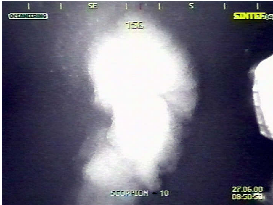
Figure 11.4. Picture identity 08-50-50. Further development of the diesel and methane plume. Undulating or meandering plume.
