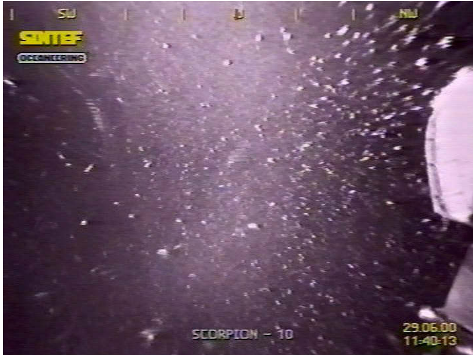
Figure 12.1. Picture identity 11-40-13. Methane release. Appearance of a gas cloud when entering into a bubble plume.
