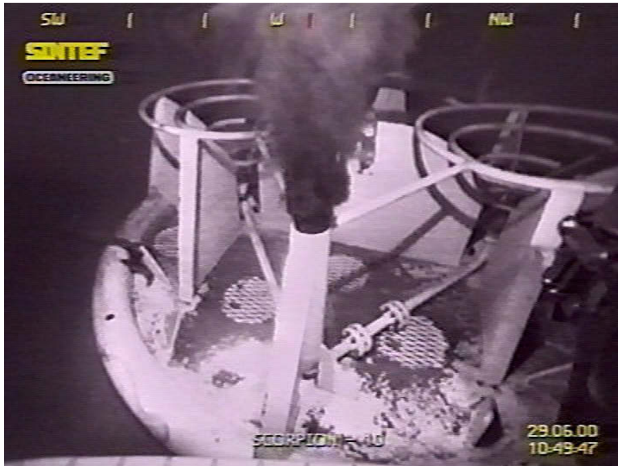
Figure 8.4. Picture identity 10-49-47. Release of dirty water the last day, prior to the methane release. The releases before this one contained the diesel and the oil release. The situation is thus similar to the one shown in Figure 8.3, except that this figure shows a more close-up picture of the release at the onset of the water release.
