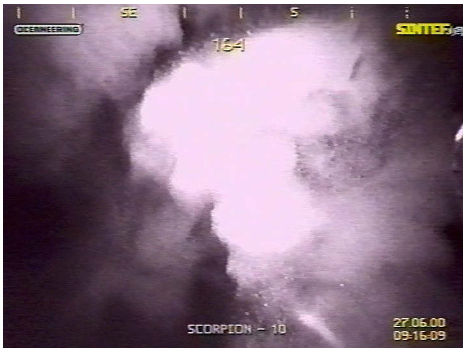
Figure 11.5. Picture identity 09-16-09. Further breakup of the plume at larger distances.
