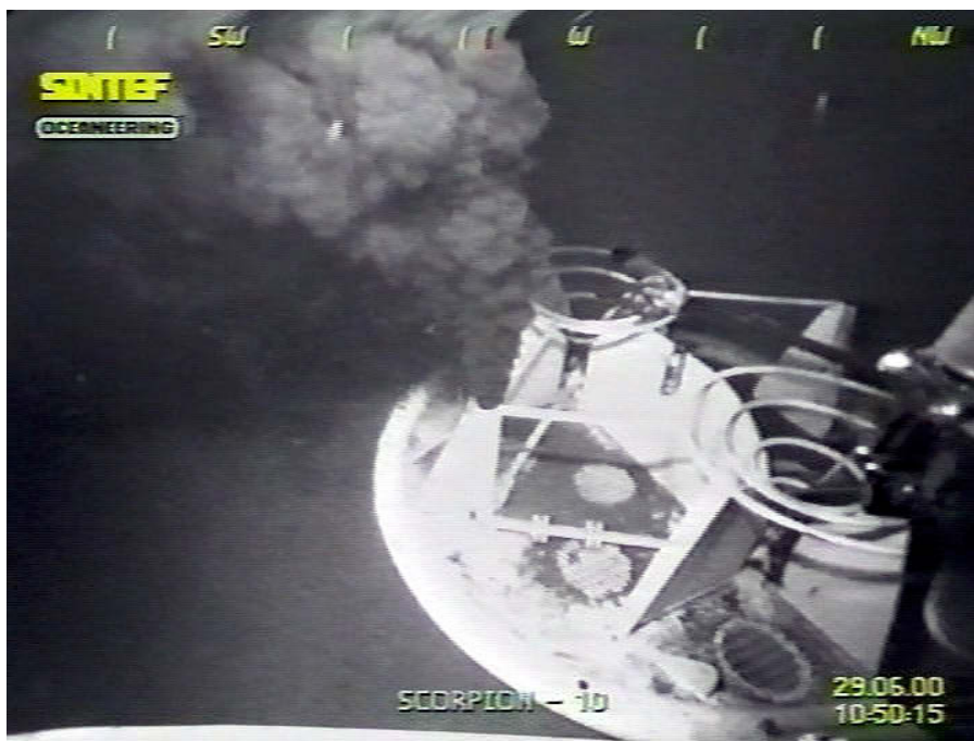
Figure 8.3. Picture identity 10-50-15. Release of dirty water the last day, prior to the methane release. The releases in the oil line before the present one contained the diesel and the oil releases. It may therefore be that the color of the water is caused by the presence of small oil and diesel particles left on the walls inside the CST. The particles are then washed out by the water flow.
