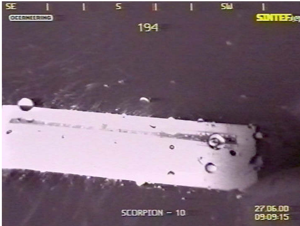
Figure 12.4. Picture identity 09-09-15. Diesel and methane release. The ruler that has been mounted is shown by the black/white camera. Also, the picture shows diesel droplets attached to the lens, which occasionally happens when the ROV moves inside the plume too close to the release point.
