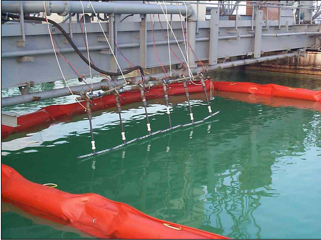
Figure 4. Oil Distribution System
