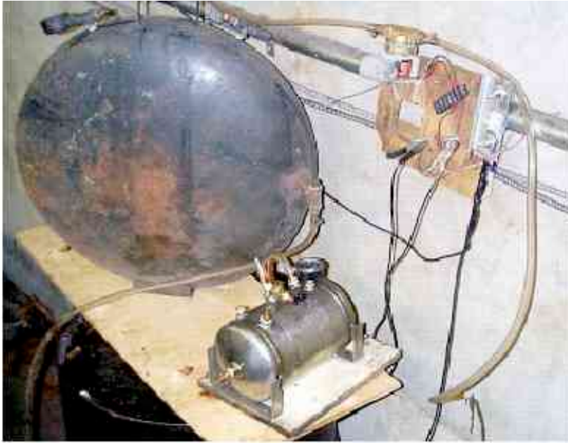
Figure 4. Dispersant Spray Pressure Tanks and Valve
