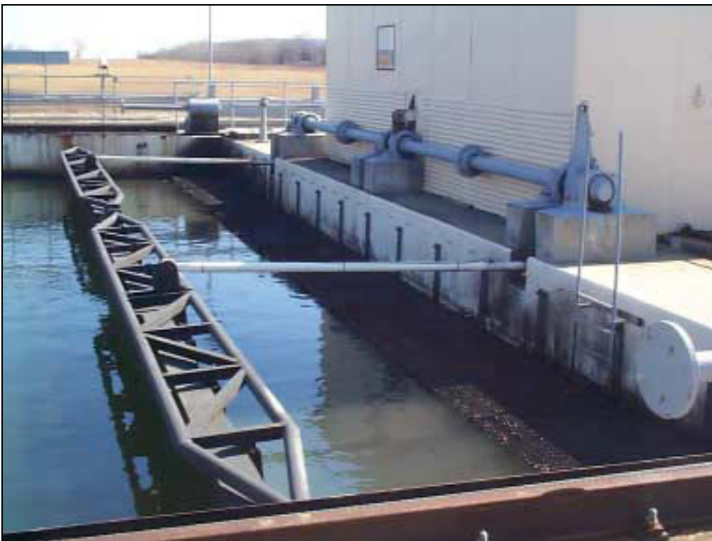
Figure 3. Ohmsett Tank Wave Paddle System
