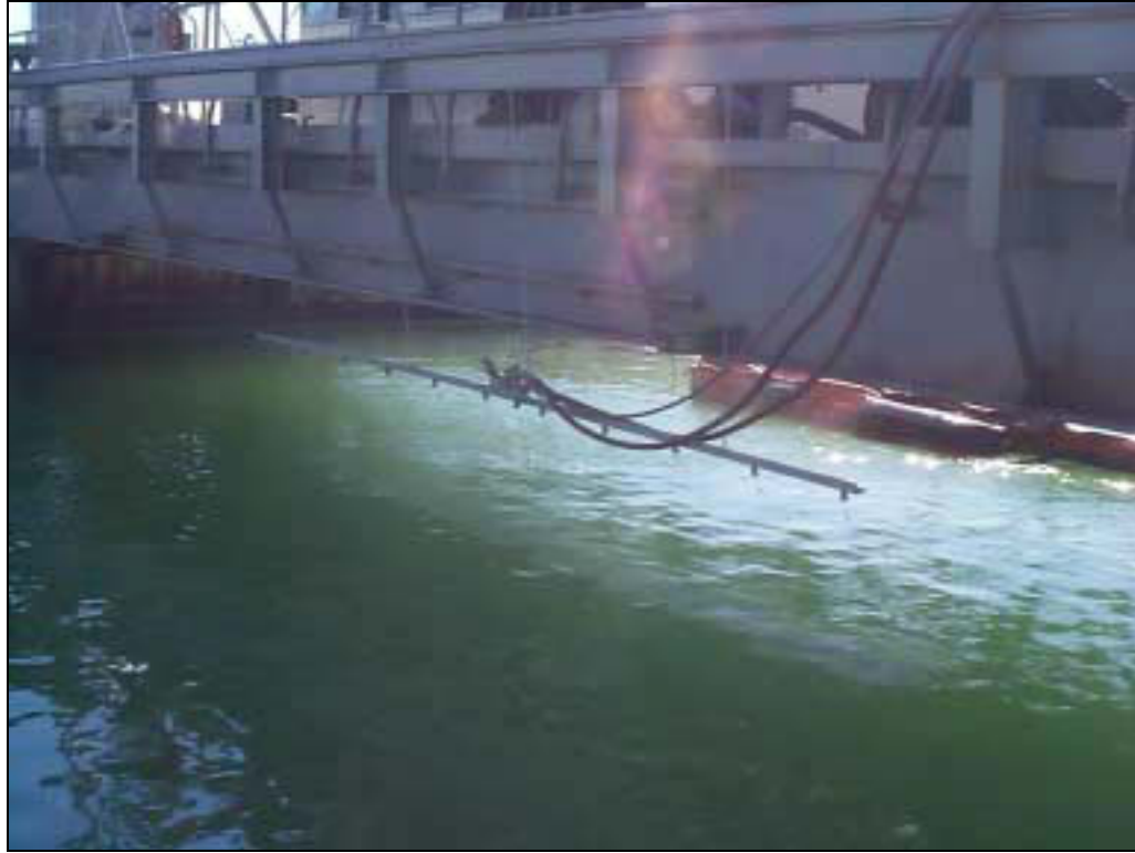
Figure 8. Dispersant Spray Bar in Operation
