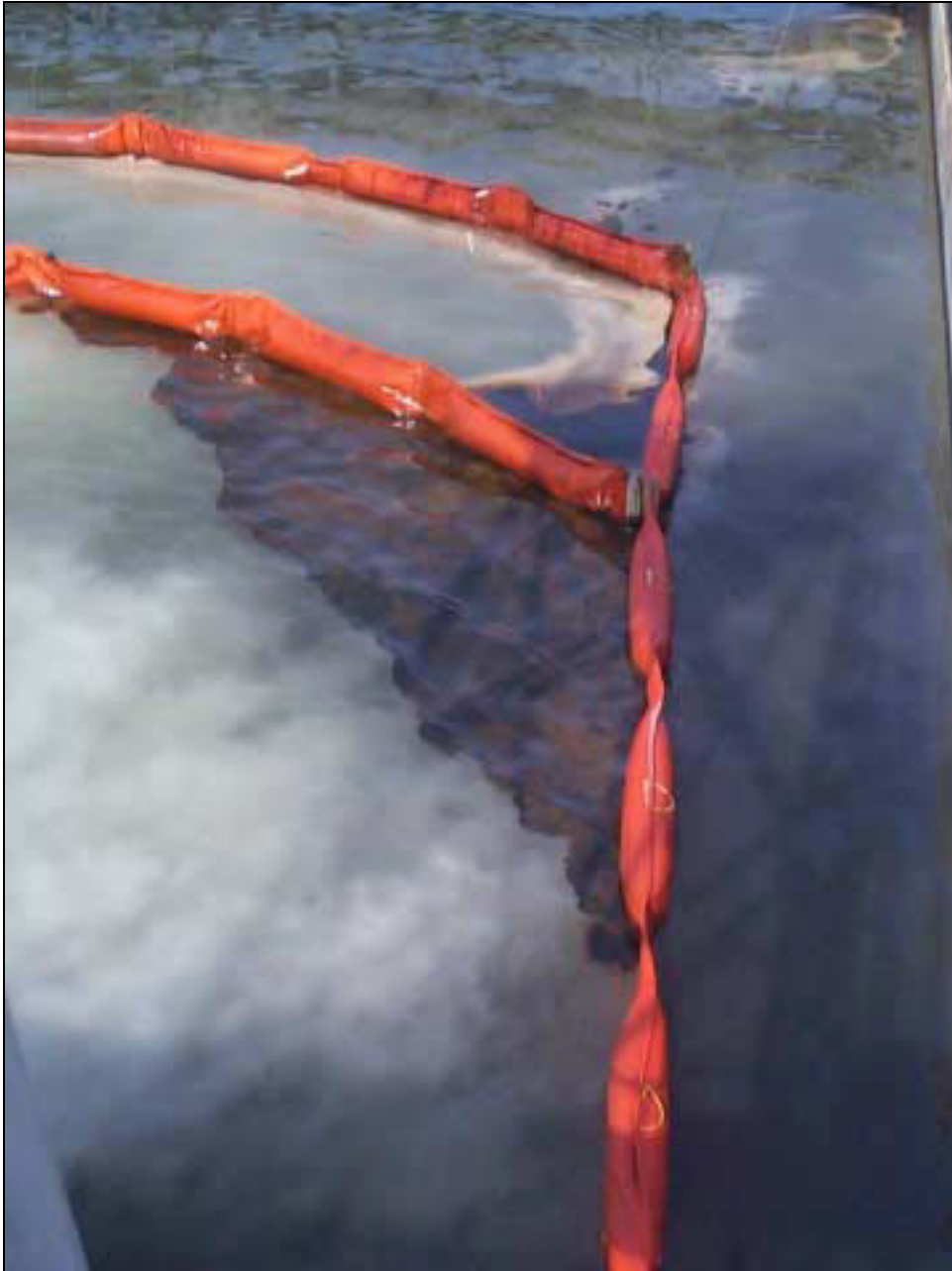
Figure 10. Oil herded to End of Double Boom for Collection
