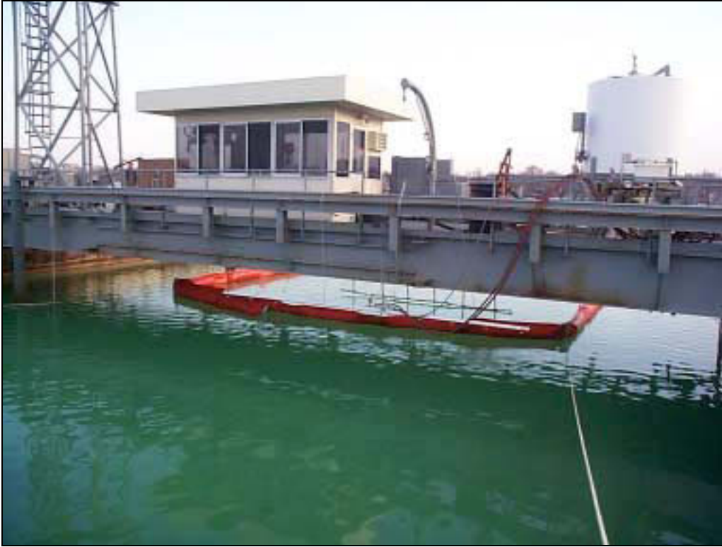
Figure 4. Main Bridge with Dispersant Spray Bar in Foreground, Oil Distribution Behind
