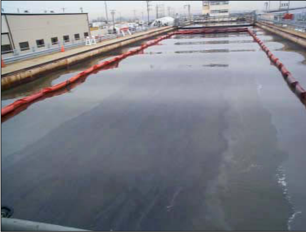
Figure 2. Ohmsett Test Tank with Oil Containment Boom
