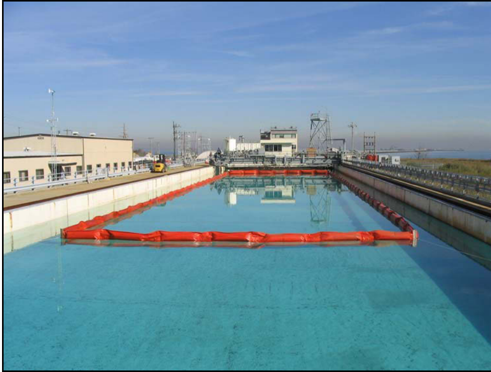
Figure 2-1: Ohmsett Test Tank with Containment Boom, October 2003.
