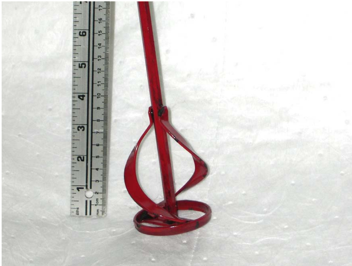
Figure 6. Paint Stirrer (PS) ... operated a two different speeds (300 and 700 rpm)
