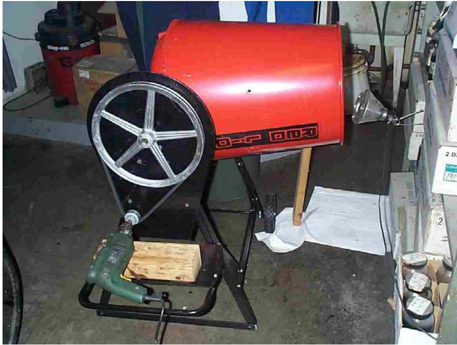
Figure 7. Cement Mixer (CM) ... operated at two speeds (20 and 30 rpm)
