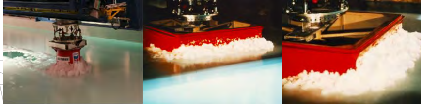
Ice rubble formation on gravity based structures (D-6, Prirazlomnoye, SSDC) and a SPAR.
