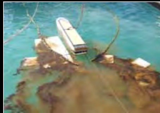
Completed basin tests using 1:25 scale workboat
