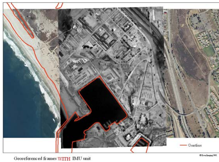
Figure 6. Auto-georeferenced imagery of San Diego coastline using only DGPS coordinate information (top) and using DGPS/IMU information (bottom).
