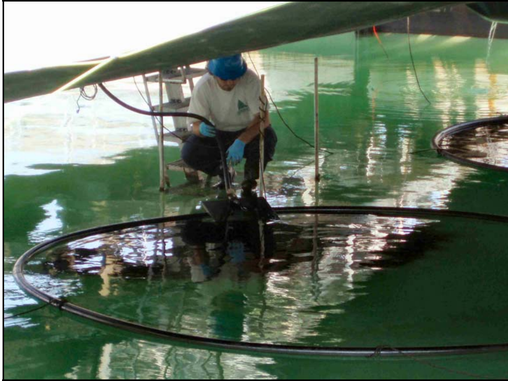
Figure 5. Oil being placed in ring
