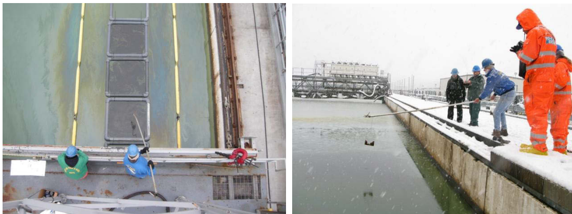
Figure 2. Crude oil samples being poured into floating containment squares in the Ohmsett tank (left) and sampling oil thickness in a patch of uncontained oil (right) during the wintertime experiments
