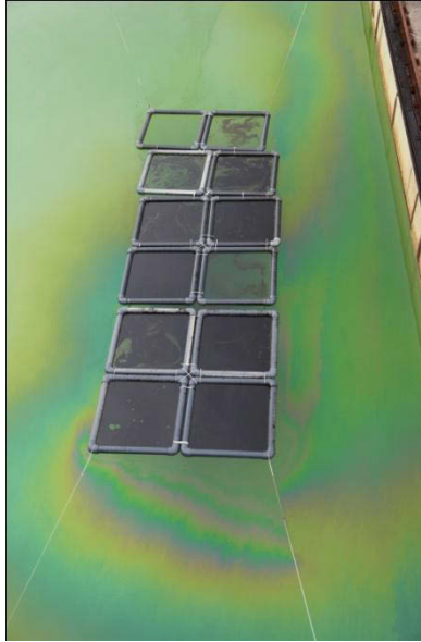
Figure 6. Floating PVC squares containing various thickness films of pure ANS crude oil emulsions and no oil for control purposes. Following each imaging experiment the squares were emptied of oil with a water jet and refilled with oil and emulsions of different thickness and oil/water ratios.
