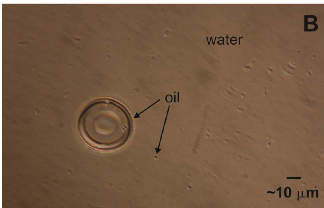
Figure 28. Clarified actual MC252 emulsion (A) and the aqueous solution resolved from this emulsion (B) under centrifugation (no Corexit or modified Corexit present).
