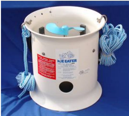
Figure 1. Ice-Eater Water Current Device Used to Generate Water Flow Barrier at Ends of Tank
