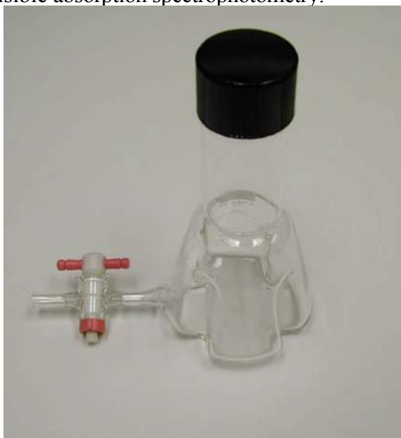
Figure 1. Photograph of the baffled trypsinizing flask.
