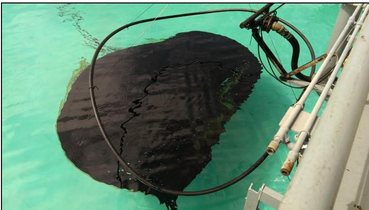
Figure 4-3 Oil Containment Ring Lifted Prior to Dispersant Application
