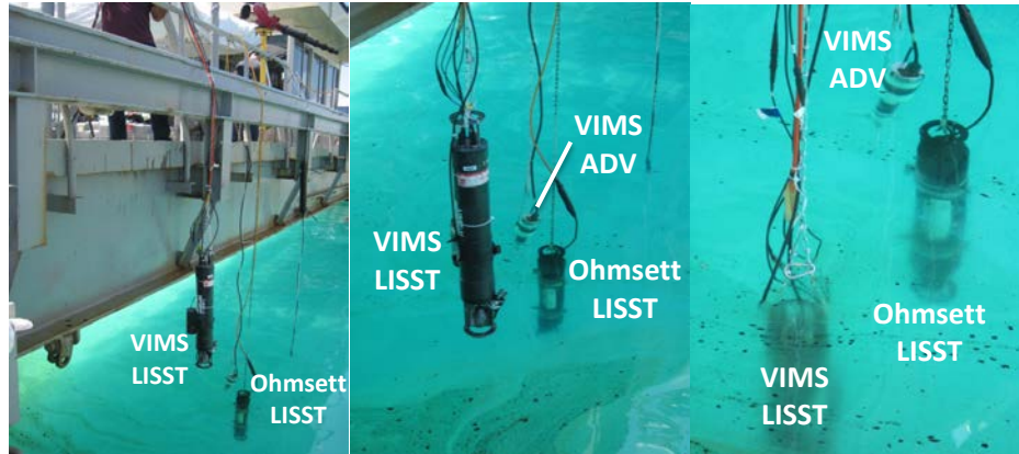
Figure 20 These photographs show the VIMS LISST as it is being deployed over the railing of the bridge along with the Ohmsett LISST. The center and right photographs show the two LISSTs along with the VIMS ADV.
