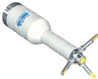
Figure 19. ADV used at Ohmsett. The transducers have yellow faces. The center transducer emits the sound and the outer three transducers receive the sound waves scattered from particulates in the water column.
