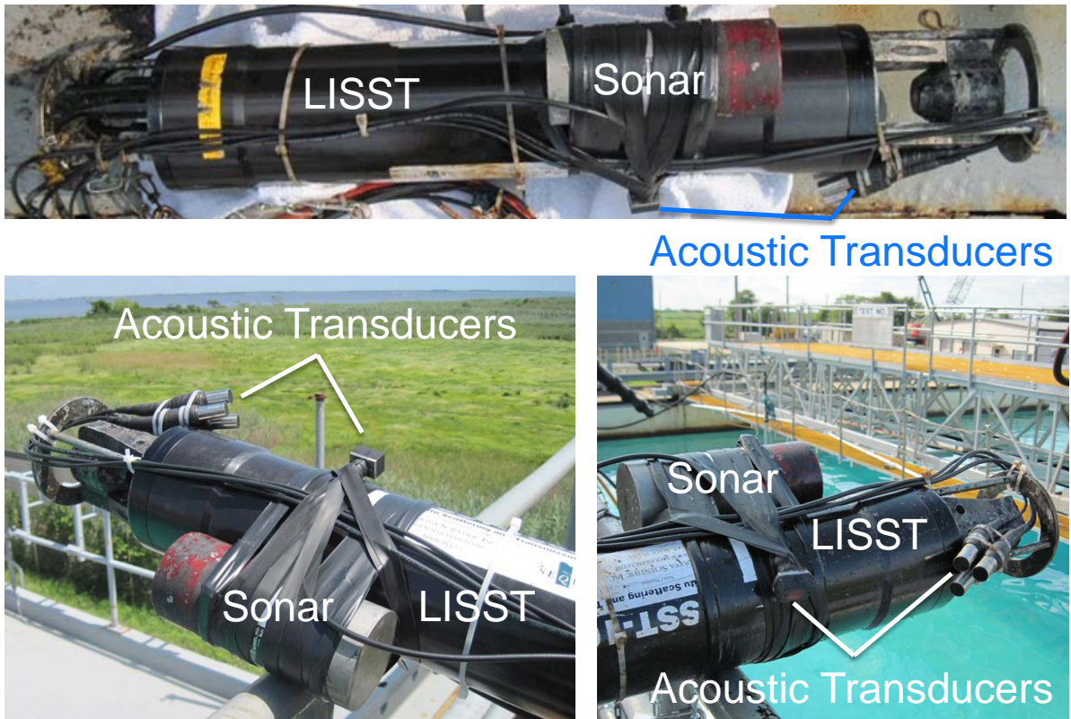
Figure 18 The configuration of the LISST, Sonar and acoustic transducers prior to deployment.
