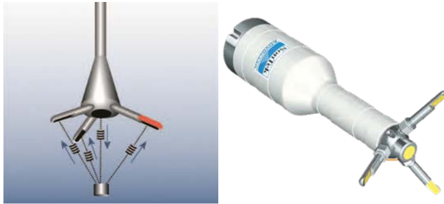
Figure 29. Images of the Sontek ADV are shown with propagation of the sound waves shown at left and a photograph of the entire instrument shown at right.
