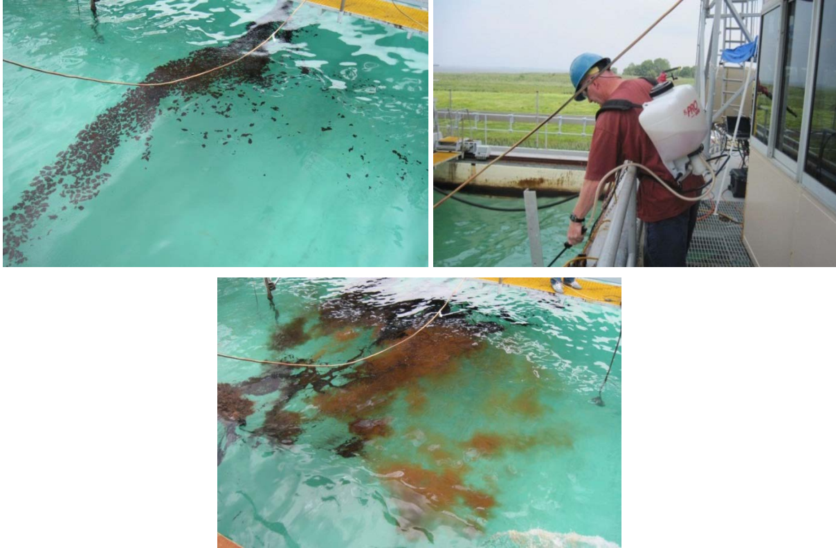
Figure 22. Photographs of one of the emulsified oils in the Ohmsett tank (top left), personnel from S.L. Ross applying dispersant using a pump sprayer (top right) and the emulsified oil after the dispersant was applied (bottom).
