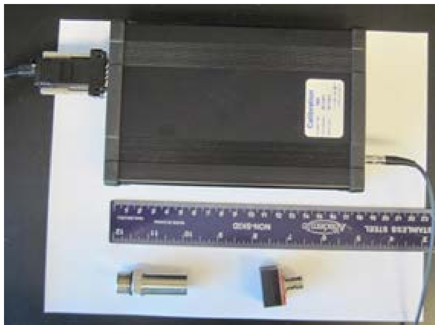
Figure 6. The precision acoustic instrument along with two acoustic transducers. The system is controlled via an Ethernet connection to the computer.
