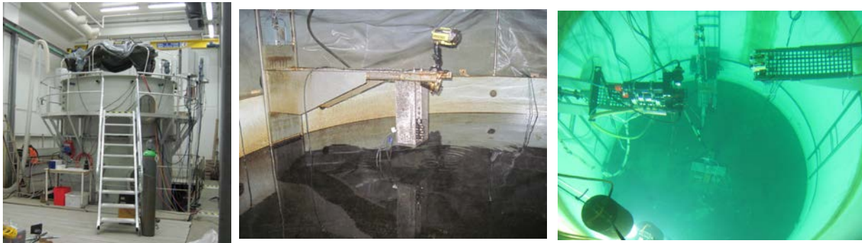
Figure 36 Photographs of the Sintef Tower tank and the installed acoustic sensors. The sensors were installed underneath the platform as shown in the center photograph. Video cameras were on top of the platform. The right photo show the sensors installed directly opposite the LISST.
