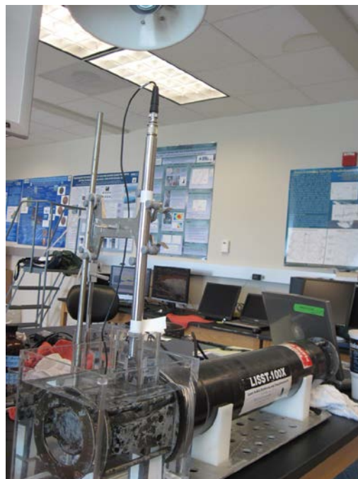
Figure 10. The acoustic test chamber for oil-dispersant mixtures. The syringe (left panel) was used to uniformly mix the suspensions. The acoustic transducer is shown pointing downward in the right panel.
