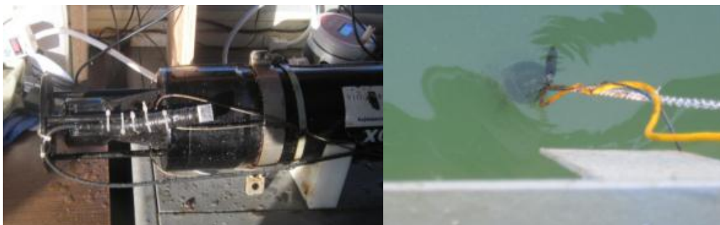
Figure 13. The ultrasonic transducer was zip tied to the LISST as shown in the left photograph and both sensors were submerged into the tank from the Tow Bridge as shown in the right hand photograph.
