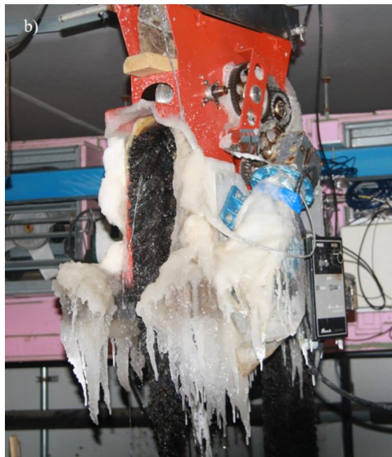
Figure 3.4. a) Ice accumulation on the rope mop at different subzero temperatures without the application of heating, b) Ice accumulation on the VAB skimmer and case at -28 °C after 1 hour testing.
