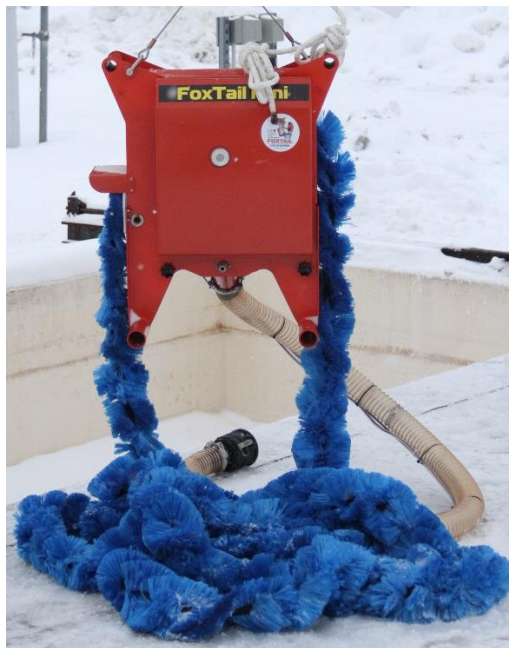
Figure 3.1. FoxTail Mini vertical adhesion belt oil skimmer used in this project.
