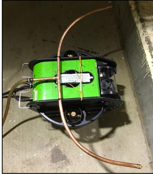
Figure 2.4. Remotely Operated Vehicle (ROV) with air applicator attached.
