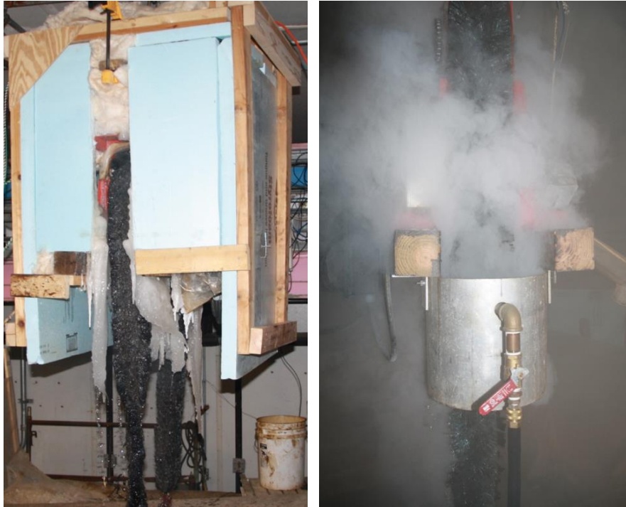
Figure 3.3 Image of insulated box with heat pads on VAB skimmer ( left ) and image of steam collar on VAB skimmer ( right ).
