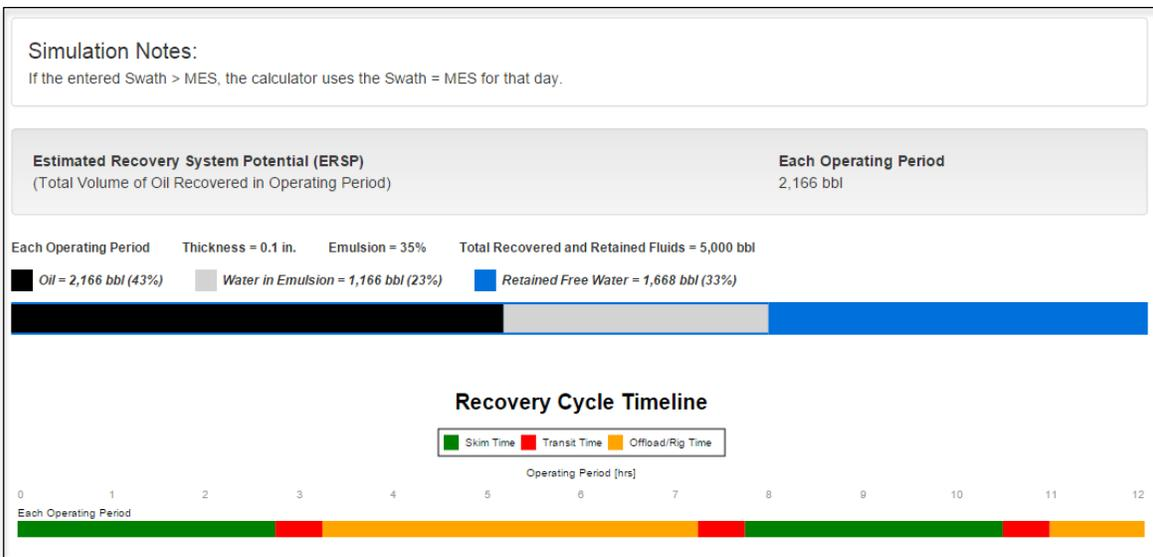
Figure 11. ERSP Graphical Outputs for Manatee Continuous Spill
