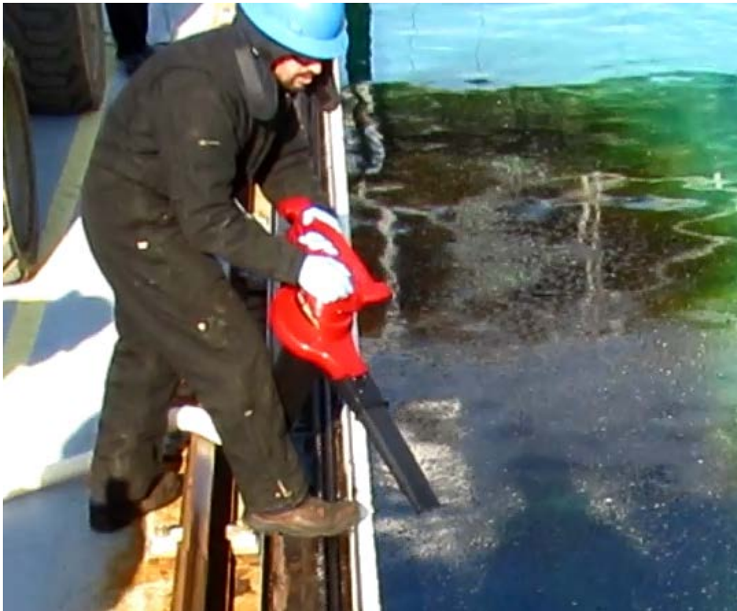
Figure 23. Dispensing i-Petrogel flakes onto water surface by a blower (Test 15).
