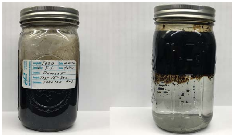
Figure 26. Recovered oil/i-Petrogel adducts (left) by skimmer and (right) scoop after 1 month.
