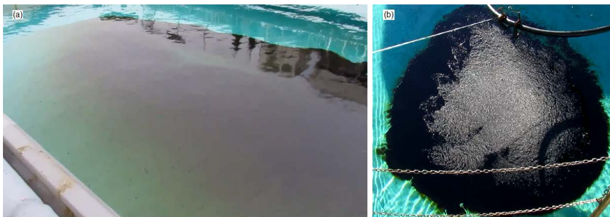
Figure 20. 2-Gallon of ANS oil was released from the O-ring and freely spreading on water surface (a) without (Test 2) and (b) with i-Petrogel (Test 3).
