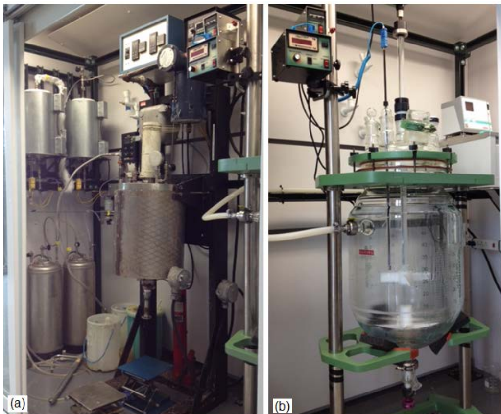
Figure 13. (a) a 20-liter high pressure polymerization system for polymerization reactions and (b) a new 50-liter reactor with control accessories.
