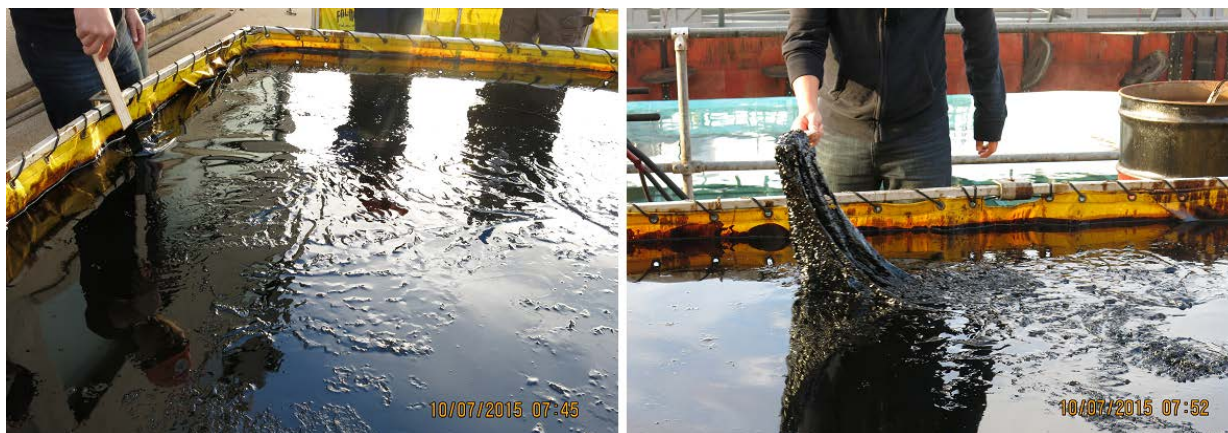
Figure 16. (a) The sheet-like ANS oil/i-Petrogel (3/1) adduct, (b) recovery of ANS oil/i-Petrogel sheet by a simple stick.
