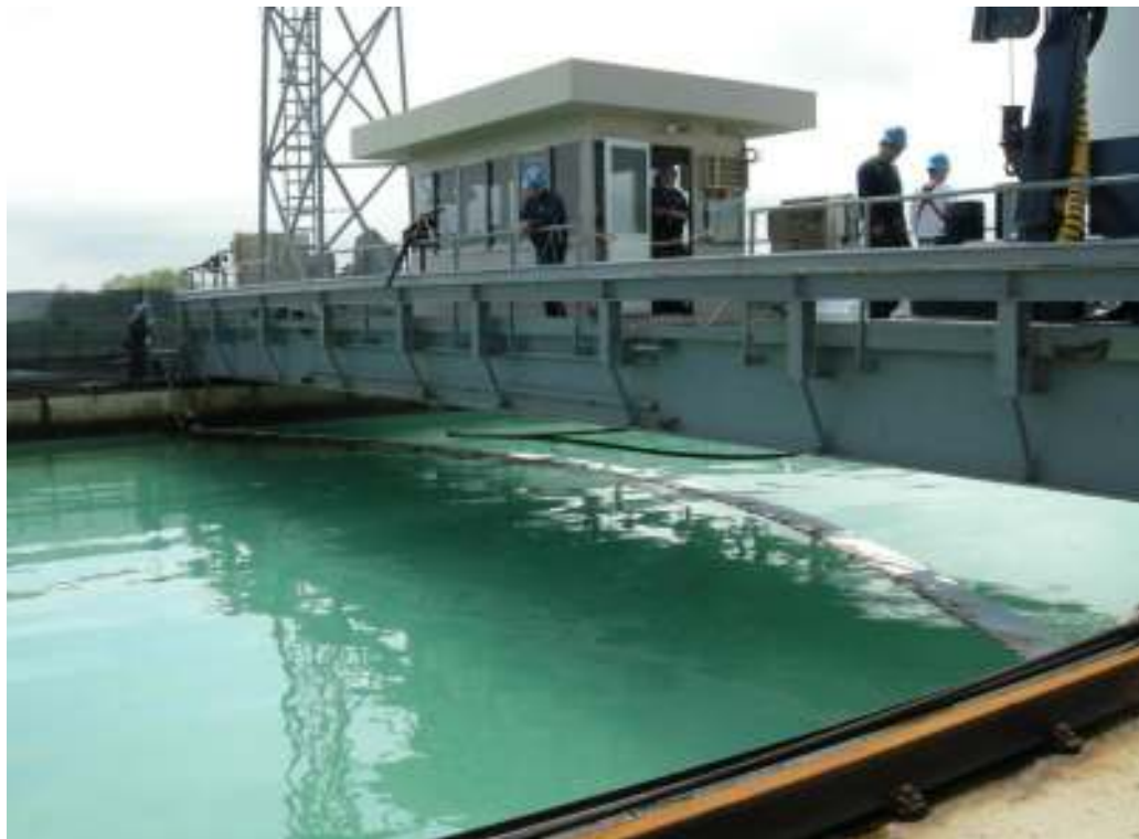
Figure 14. Cleaning water surface in test area with sorbent sweep attached to Main Bridge.
