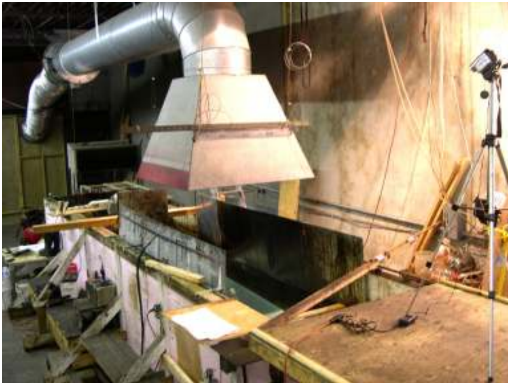
Figure 5. Wind/wave tank set up for burn experiments with heat shields and exhaust hood.
