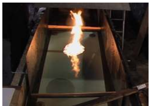
Figure 5. Herded slick burning in wind/wave tank
