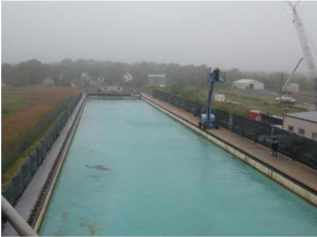
Figure 13. Ohmsett tank during herder persistence testing showing wind screens and person lift.
