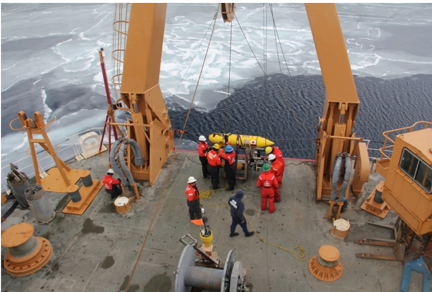
Figure 3.2.1 A-frame on stern of the Healy viewed from adjacent to the vehicle conning station. This was used to deploy the AUV as the port crane reportedly was not working properly and the starboard crane was used for other operations during the exercise. Nilas (thin grey ice < 10 cm thick) and broken ice were frequently present off the stern so that the AUV was often deployed and recovered amongst ice.
