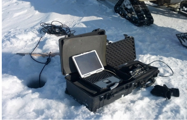
Figure 3.4.1 Laptop (left) and acoustic modem (right) with ice hole for transducer in background.
