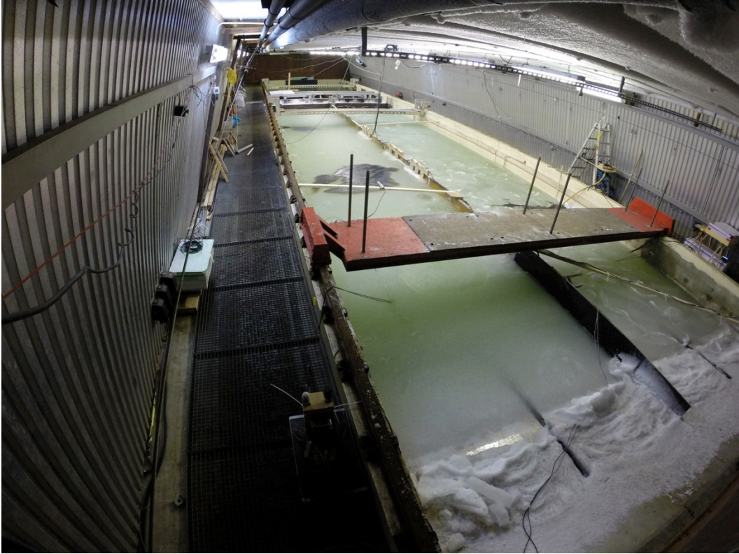
Figure 4.3.1 The AETB facility at HSVA, Hamburg, Germany. Toward the back is the wave-maker. The basin was divided into three tanks. Beyond the wave-maker was the quiescent tank (tank 1). Tank 2 (at left) was used to produce frazil and white nilas. Tank 3 (at right) was used to produce pancake ice. The instruments were deployed on a trolley that ran along rails on the bottom of the tank. The trolley was lowered from the movable bridge across the tanks and pulled back and forth toward the “beach” in the foreground where the wave energy was dissipated. Spilled oil can be seen in the center of tank 2.
