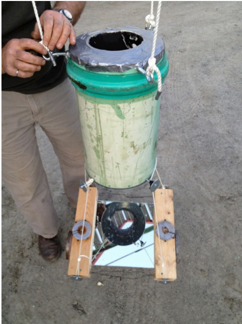
Figure 4.2.2 Set-up for the laser fluorescence installation. An insulated PVC tube with a mirror beneath was use to keep a clear optical path from above the ice (left). Laser system viewed from behind (below).
