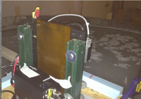
Figure 4.2.2 Set-up for the laser fluorescence installation. An insulated PVC tube with a mirror beneath was use to keep a clear optical path from above the ice (left). Laser system viewed from behind (below).
