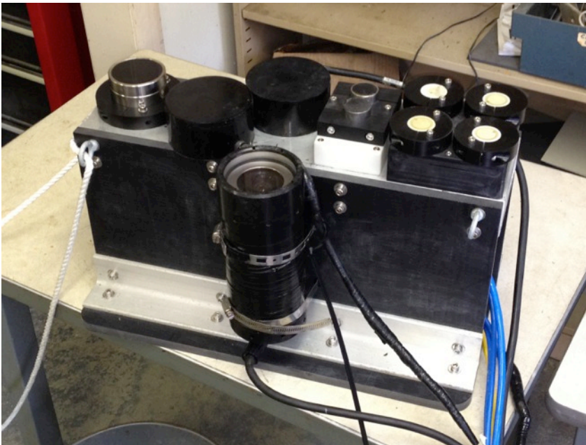
Figure 4.7 The sonar transducers mounted at the bottom of the test tank. From left to right: Marine electronics 1.1 MHz profiler, two 160 kHz Airmar transducers for the broadband system, two 500 kHz Airmar transducers for the broadband system, and four Aquascat transducers (there 1 MHz (two connected) and one 5 MHz). A Prosilica low-light camera is mounted in an underwater housing on the side of the instrument platform.
