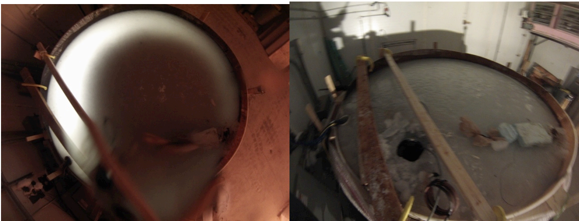
Figure 6.1.1 Photographs of the ice tank with the ice and encapsulated oil from above, illuminated from below in the dark (left), and in daylight from above with no underwater illumination (right).
