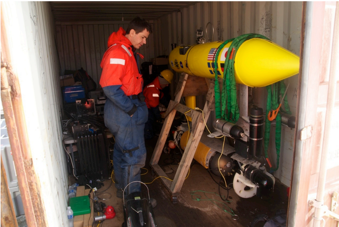
Figure 3.1.2. The Jaguar AUV in the storage container on the deck of the Hollyhock. The vehicle was pushed out of the container on the wooden A-frame trolley, where it was hooked to the ship's crane for deployment.
