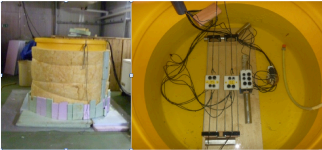
Figure 4.3.9. A 1.4 m diameter insulated tank was used to perform broadband measurements of oil under congelation ice at HSVA (left). The six ‘time series’ transducers were centered horizontally and located at the center of the tank. The four pairs of transducers for spatial measurements were deployed on two rail systems allowing the transducers to be pulled horizontally to span a range of approximately 90 cm (right). Various pipes through the ice were used for cables runs, to release hydrostatic pressure, and to move the carts.
