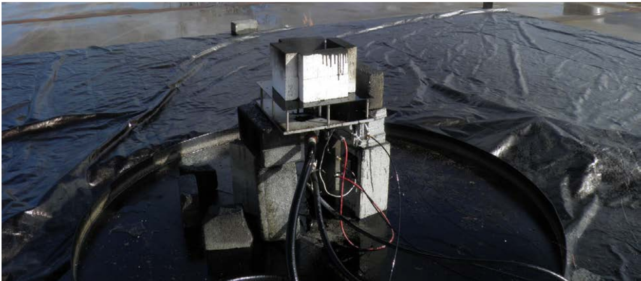
Fig. 12-Burner surrounded by fire bricks during unsteady combustion
