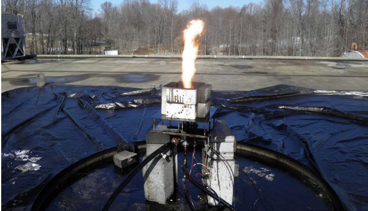
Fig. 13-Burner mounted on pool fire catch basin and tarp to catch un-burned oil droplets: nozzle diameter = 7.04 mm, oil flow rate = 800 mL/min, and ALR = 0.5
