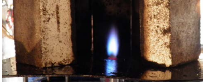
Fig. 13-Ignition torch, tuned to eject luminous reacting flame
