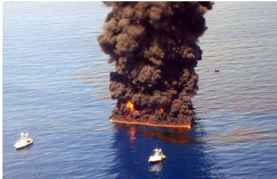
A containment boom is being carried between two boats to facilitate and control in situ burning [9].
