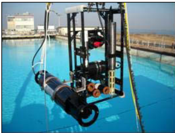
Figure 19. LISST attached to WINDOW sensor cage.
