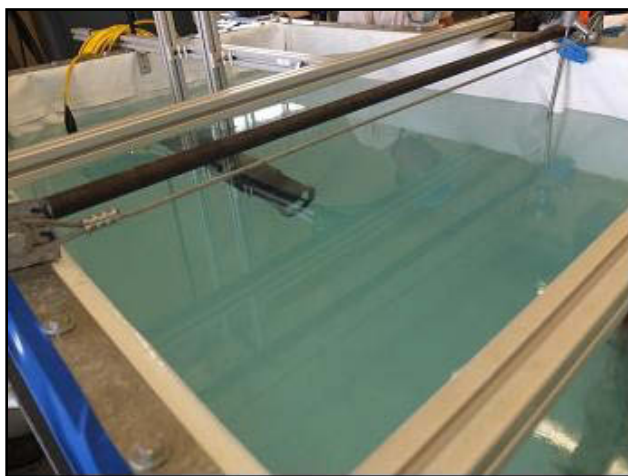
Figure A-4. LISST particle size analyzer in its support frame.
