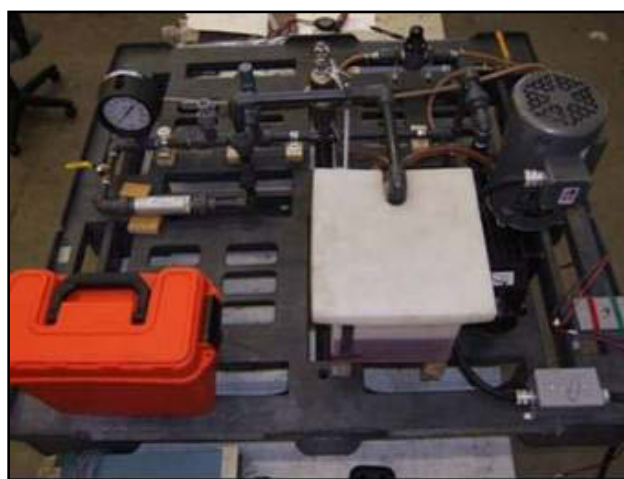
Figure 3. Oil dispensing system.
