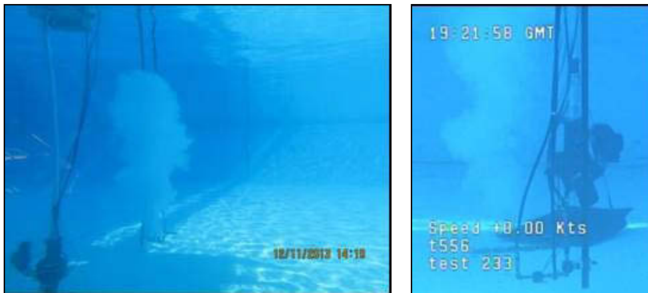
Figure 14. Release of diesel with dispersant, sonar and nozzles 2 ft from bottom.
