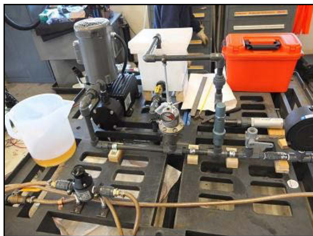
Figure A-2. Oil delivery pump system.
