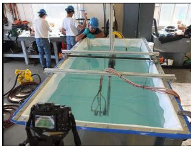
Figure A-3. Modular tank with nozzle apparatus in place.
