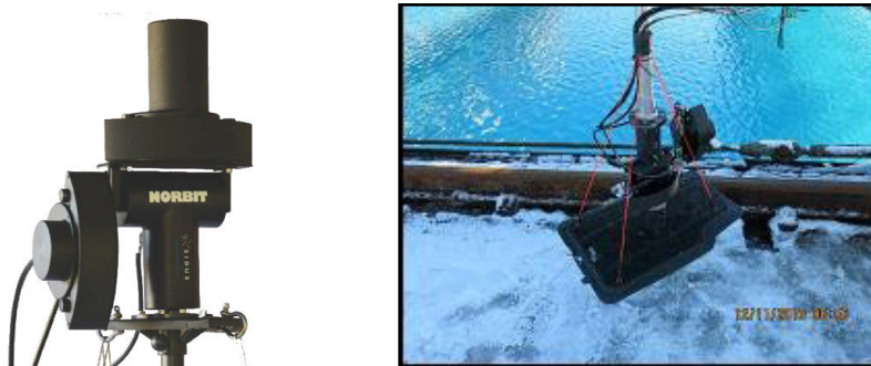
Figure 9. WBMS system with two sonars (left) and anechoic mat (right).
