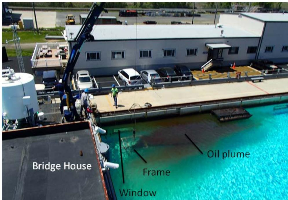
Figure 25. Testing of dispersant application for subsurface releases of oil and gas in the Ohmsett tank.
