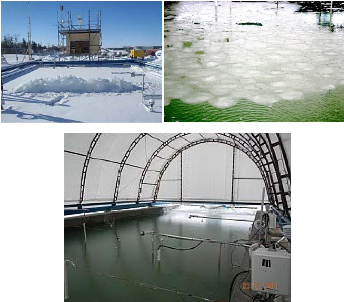
Figure 30. The outdoor saltwater pond in various stages of ice coverage and with the movable roof over the tank.
