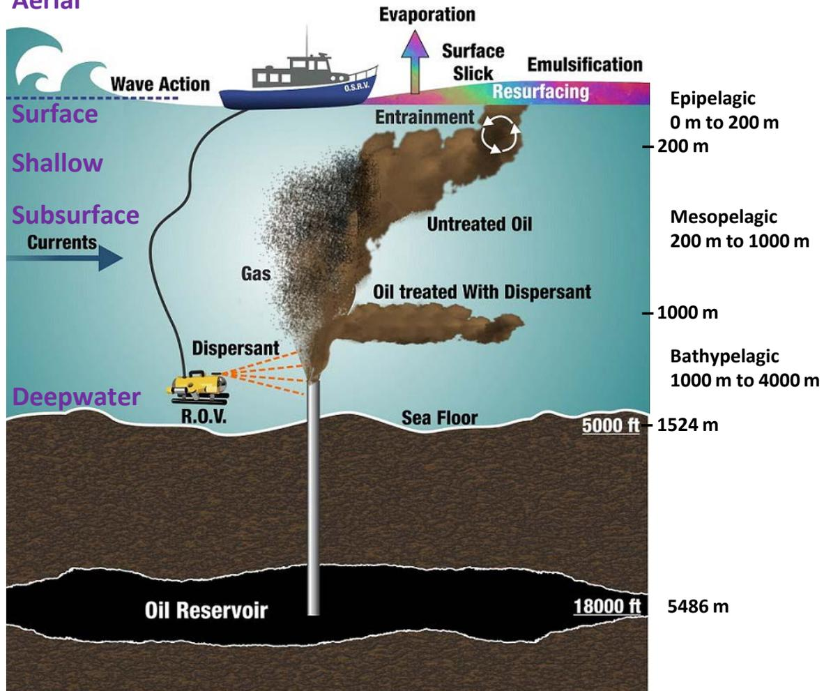
Figure 14. Operational spill environments, cross-referenced to oceanic depth zones.
