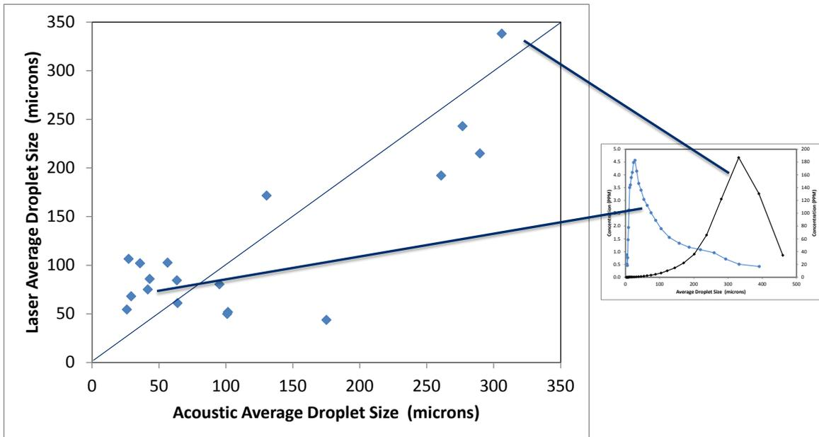
Figure 4. Proof of concept data for acoustic measurements of mean oil droplet size during TRL 3 research.
