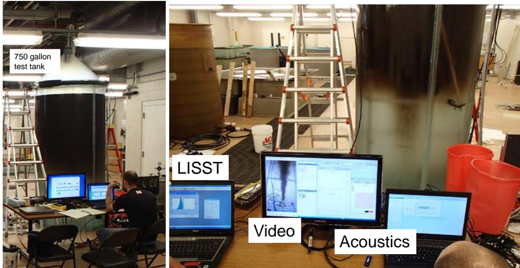
Figure 38. Testing of subsurface releases of oil and gas at the VIMS Seawater Research Laboratory.
