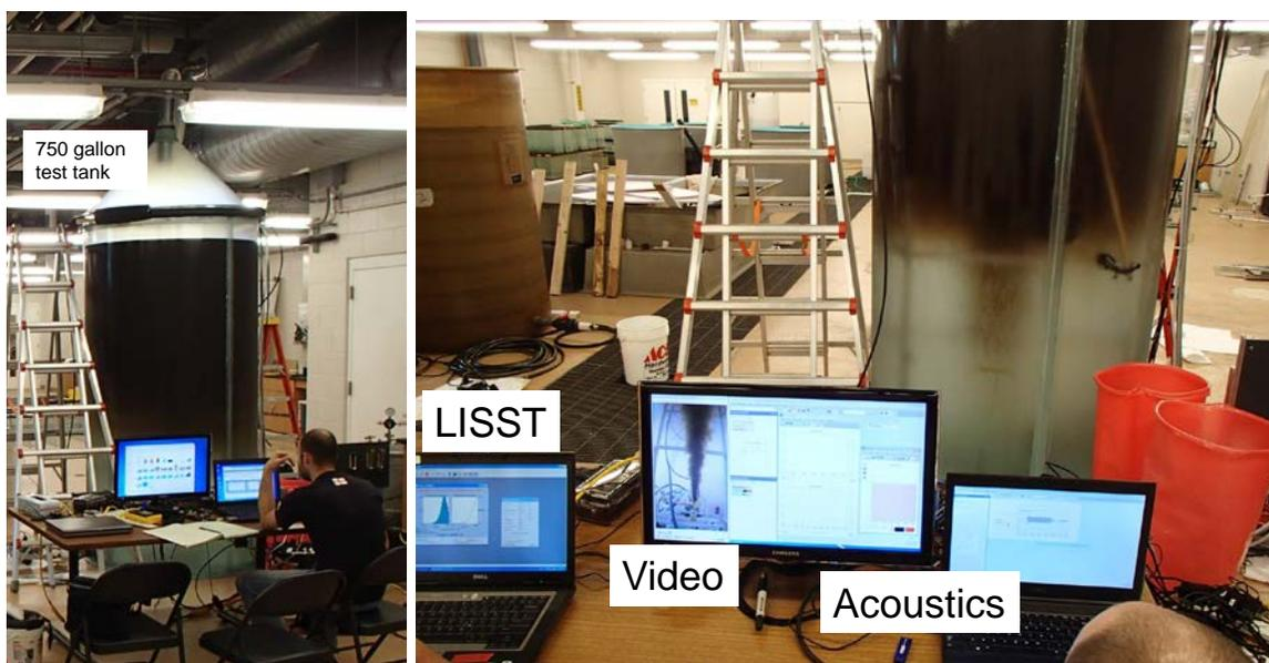
Figure 3. Subsurface releases of oil and dispersant to produce proof of concept data and achieve TRL 3.
