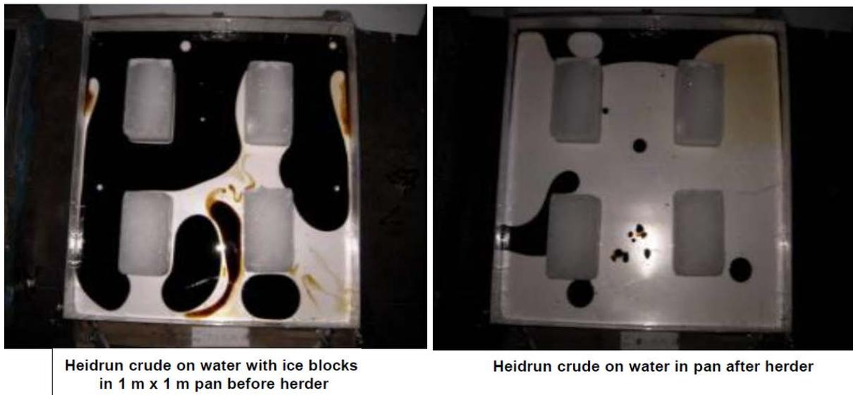
Figure 8. Small-scale lab testing of herding agents.
