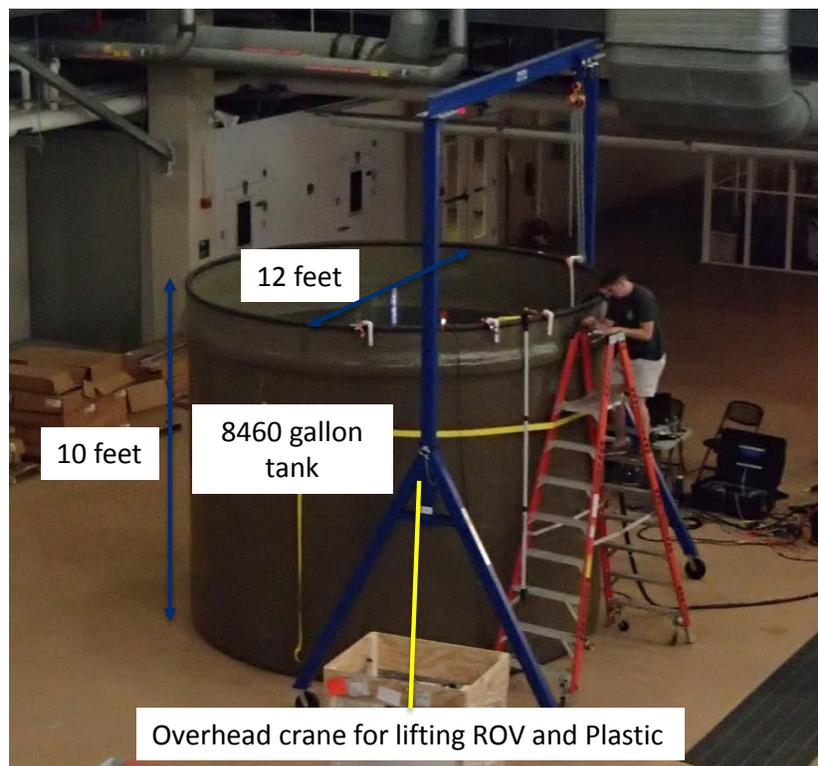
Figure 37. A large tank for oil testing installed at in the VIMS Seawater Research Laboratory.
