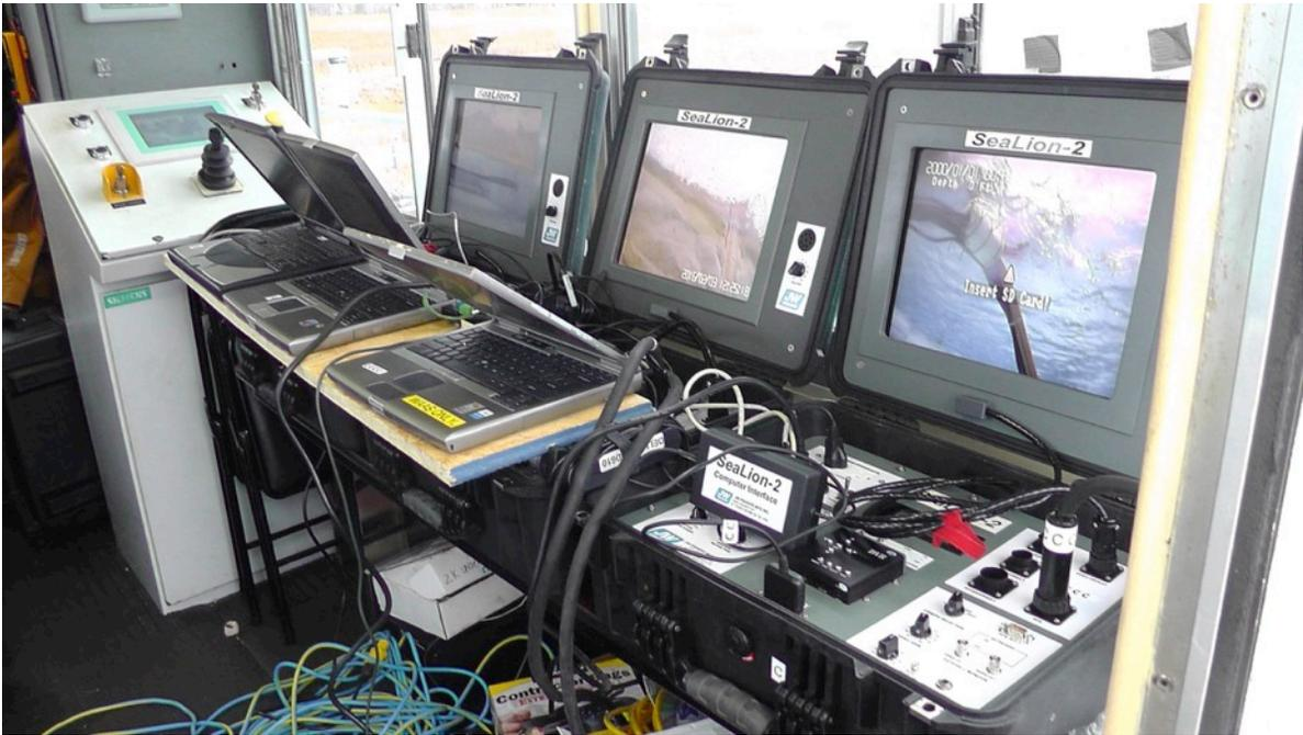
*Figure 17: ROV controllers located on table in the Main bridge.*
