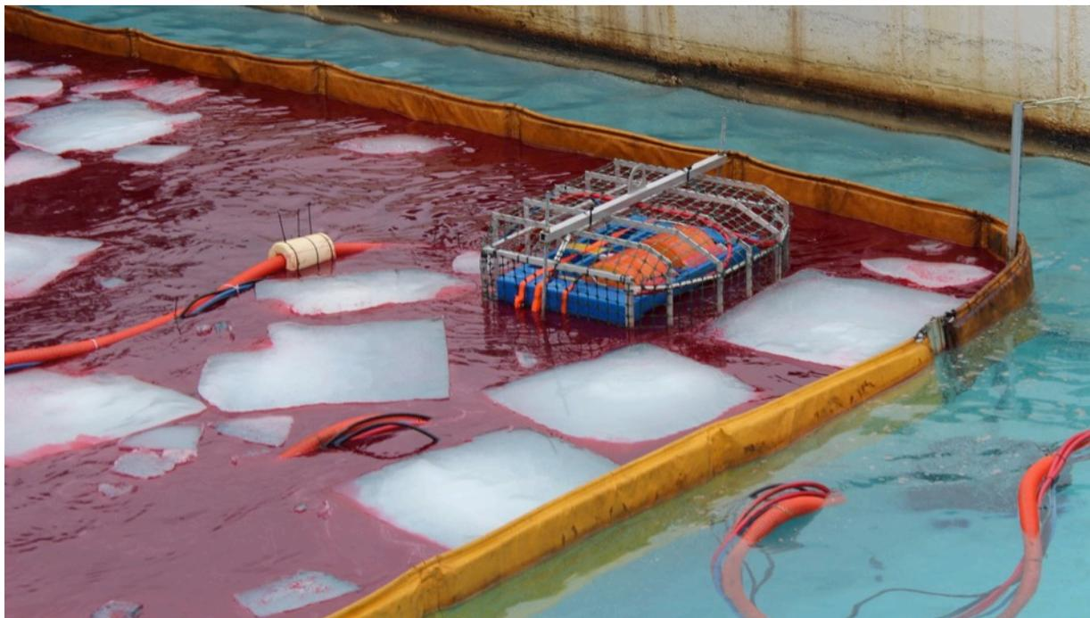
*Figure 27: ICEHORSE with ice jammed against the boom.*
