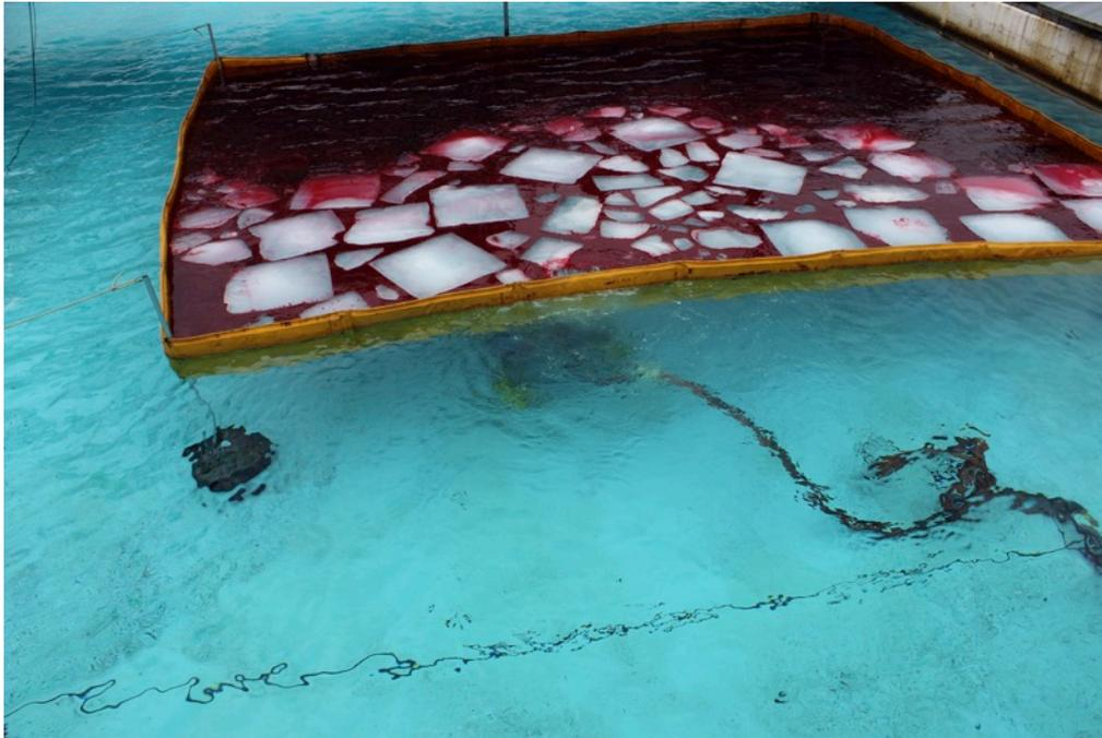
*Figure 24 Test area with 30% ice coverage with oil; note that ice is all drifted into about half of the test area.*
