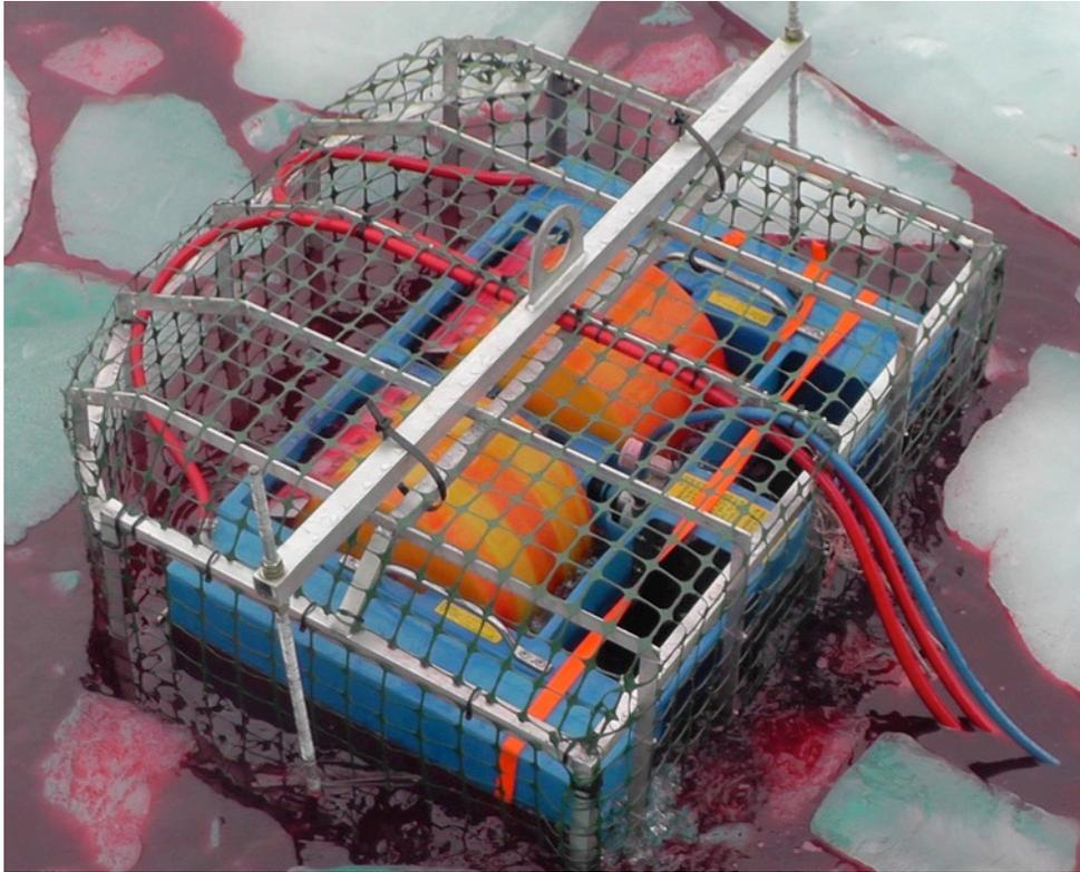
**Figure 30: ICEHORSE in operation not effectively picking up oil - drum NOT fully coated, the drum speed is too fast.**
