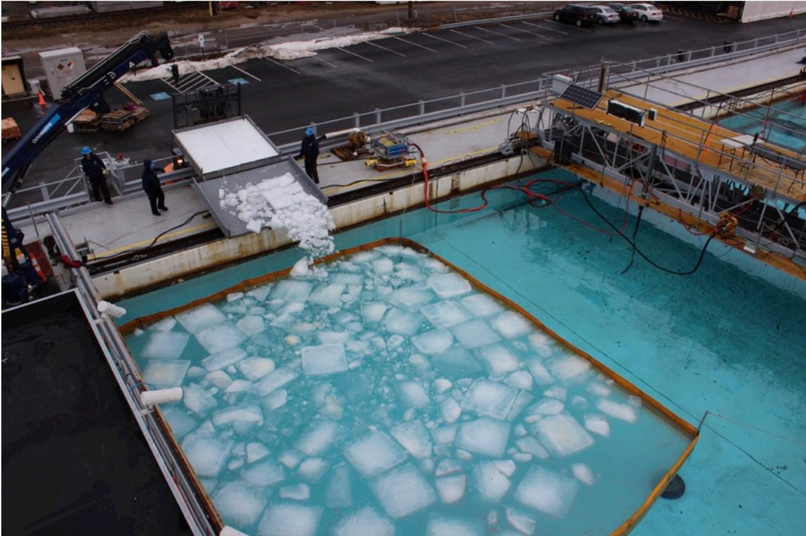
**Figure 14:** Test Area as set up at Ohmsett; Auxiliary bridge is to the right, Main bridge to the left, yellow boomed area is the test area. Shown here with ice being loaded for the 70% ice concentration.
