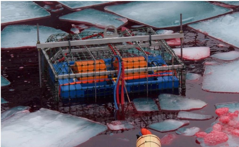
*Figure 29: ICEHORSE in operation - drum fully coated with oil indicating that it is picking up oil well - the drum speed is good.*
