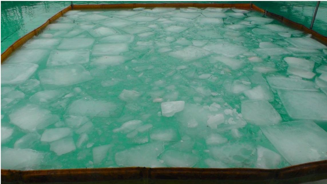
*Figure 25 Test area with 70% ice coverage with no oil, note even distribution of ice and range of ice sizes.*
