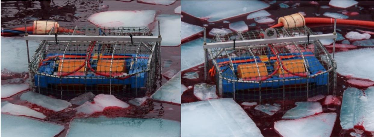
*Figure 28: ICEHORSE ice cage and mesh were effective at keeping ice out.*
