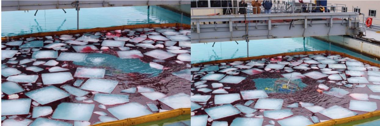
*Figure 26: ICEHORSE surfacing into oil and ice (70% ice coverage).*
