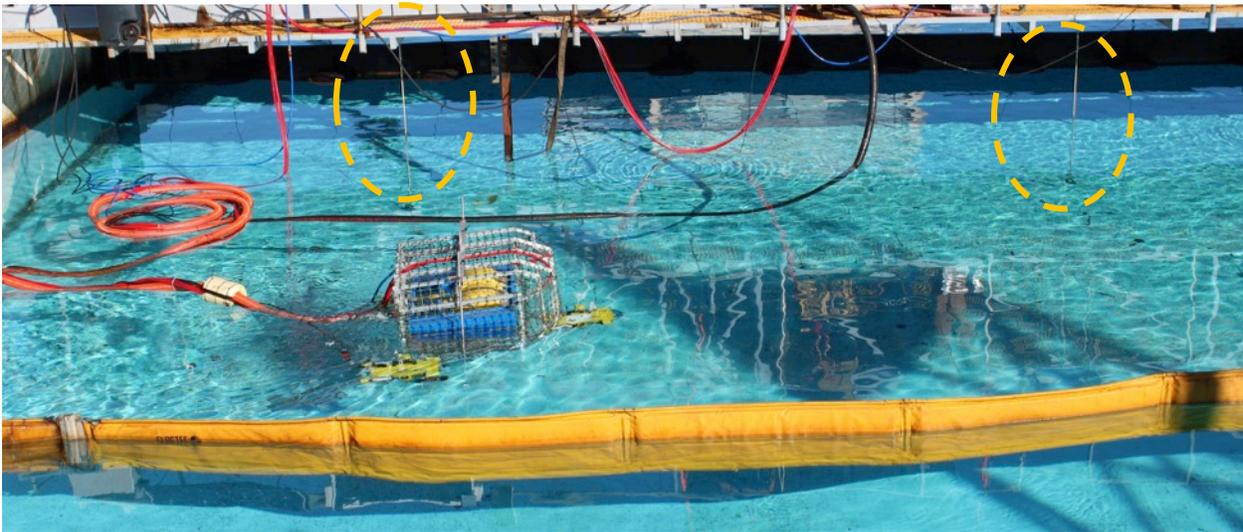
*Figure 20: ICEHORSE time trial on surface; notice slight upward pitch when accelerating. The start and stop markers (lines hanging down from Auxiliary bridge) are circled in orange.*
