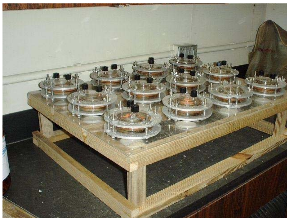
Figure 3.5 Rack System for Holding Multiple Chambers
