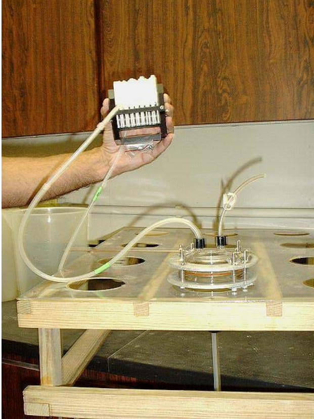
Figure 3.8 Tubing Set-up for a Single Chamber
