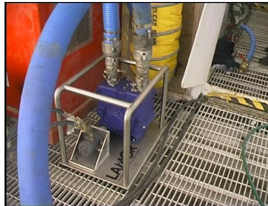
LAMOR unit, peristaltic pump for recovered product.
