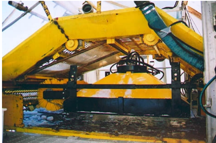
Figure 3.13 LAMOR recovery unit installed in the Lifting Grated Belt, Prudhoe Bay.
