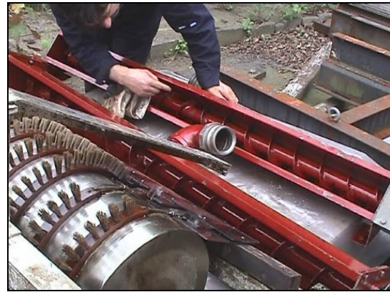
Brush Drum and troughs with screw augers. Note that the two augers operate in different directions when moving product to the outlet at the middle of the troughs.
