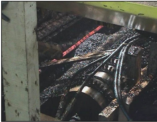
Brush Drum operating in oil and ice. The screw auger is piling up recovered ice and oil at the middle of the trough (the conveyor pump is not running).
