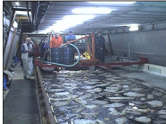
Ice conditions after some time of operation. Ready for the next test, two open top containers for recovered product.
