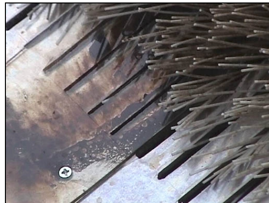
LORI brush unit. The front comb/scrapper has very wide openings. A small lexan (transparent) section of more narrow comb was installed to see the difference.
