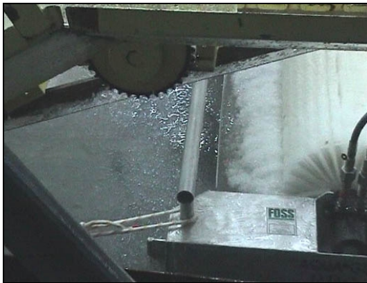
Modified Aquaguard RBS-10 inside LGB, testing the ice processing capability.
