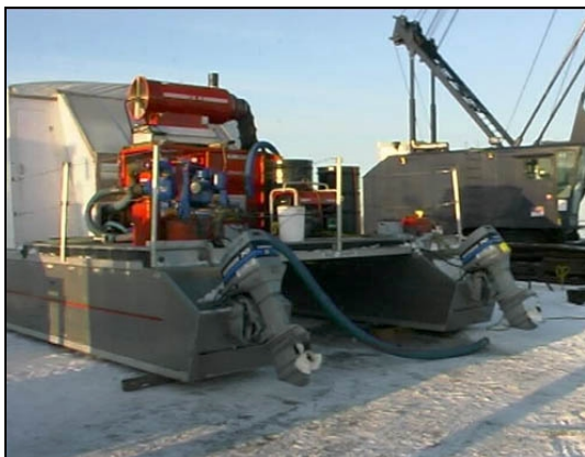
Rear of the work platform with outboards and auxiliary equipment on the working deck.
