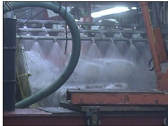
Flushing oil off ice. The spray from adjacent nozzles are overlapping, and nozzles in different spraybars are staggered.
