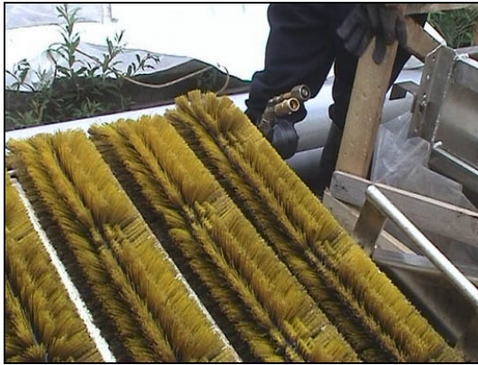
LORI brush pack after operation in ice and oil, sections of bristles have been cut away to give room for ice pieces.
