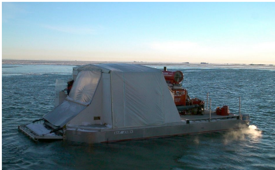
Figure 3.1 Work platform with modified shape of the superstructure at the bow.
