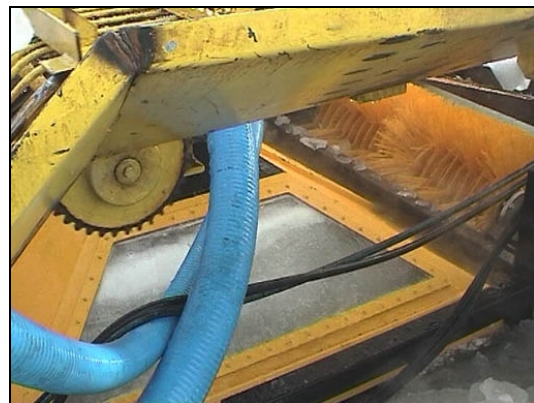
LAMOR unit operating inside Lifting Grated Belt. This "bell" has a window on one side to observe the level inside.
