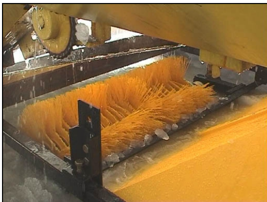
LAMOR unit operating inside Lifting Grated Belt. The cylindrical brush moves ice and oil into the "bell". Some bristles have been removed to improve ice processing.
