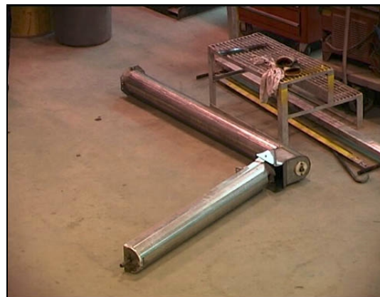
LORI recovery unit, horizontal and vertical screw augers connected prior to installation.
