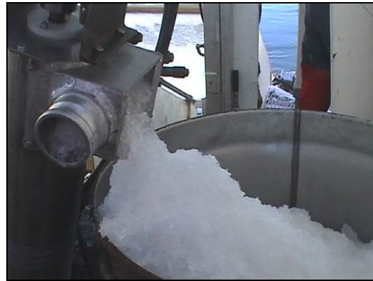
LORI recovery unit, the recovered product is falling from the entrance of the vertical screw auger into the open top container.
