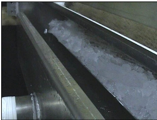
LORI brush unit, rear trough full of fairly dry ice that is not moving towards the outlet, very hard to transfer with a pump.
