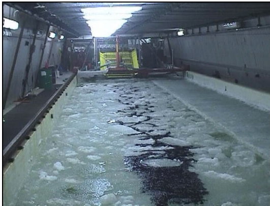
Ice conditions in the HSVA test tank immediately after the first oil has been deployed. We see a lot of small/slush ice. About 2 m of fast ice is left on the righthand side of the tank.
