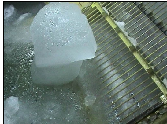
Recovery unit (Aquaguard RBS-10) not able to process the ice fast enough, resulting in small ice building up inside the grating of the Lifting Grated Belt.
