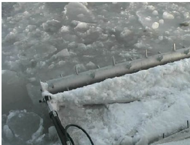
Figure 3.2 Ice feeder operating in broken ice. Snow covers the frame with the aluminum plate.
