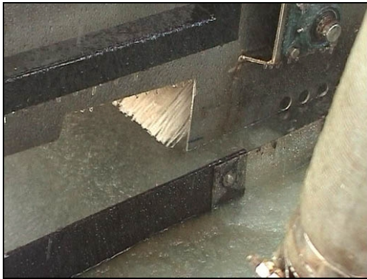
LORI recovery unit, we see the waterline of the inlet with bristles.
