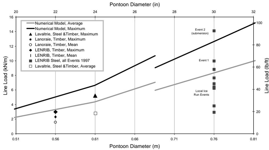
**Figure 5.6: The Effect of Pontoon Diameter on a Pontoon’s Ice Retention Capacity**
