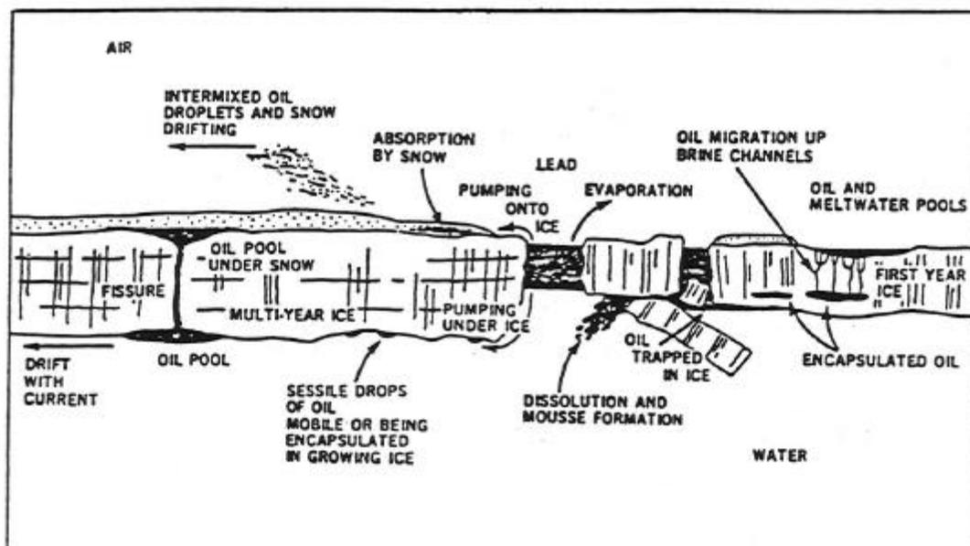
**Figure 1.1: Oil Behavior and Fate in Broken Ice (after Bobra and Fingas, 1986)**
