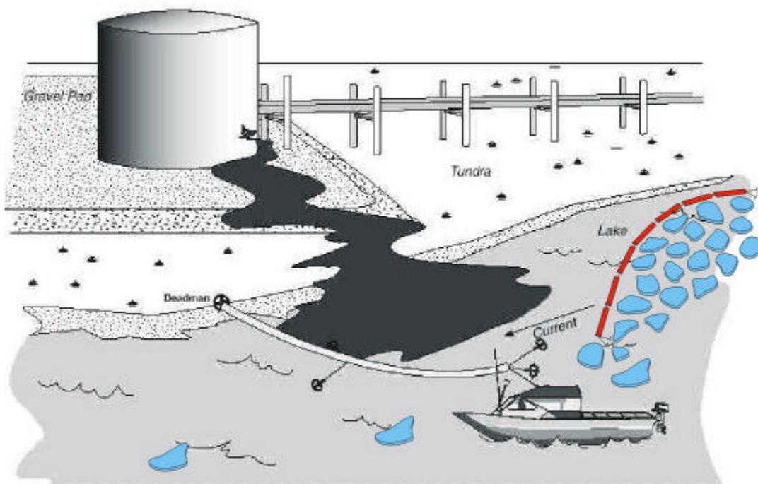
**Figure 3.7: Continuous Spill from a Reservoir**
