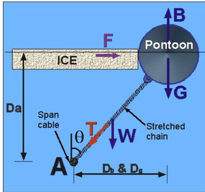
**Figure 5.7: The Ice Action on the Pontoon before Submergence**
