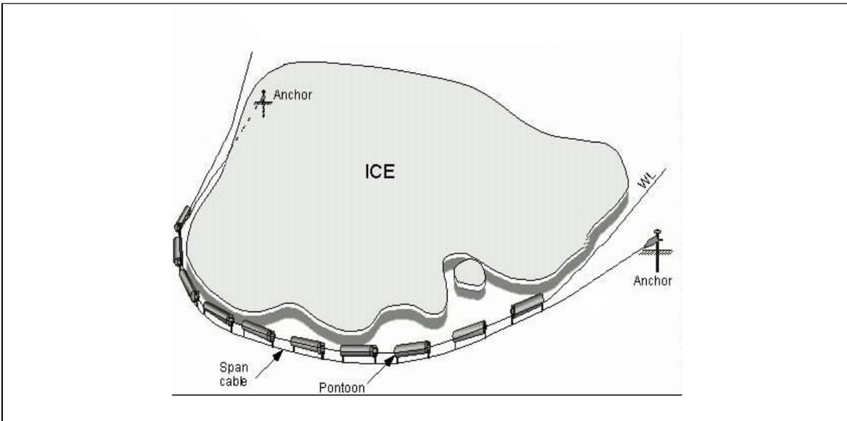
**Figure 2.2: Ice Boom Schematic**
