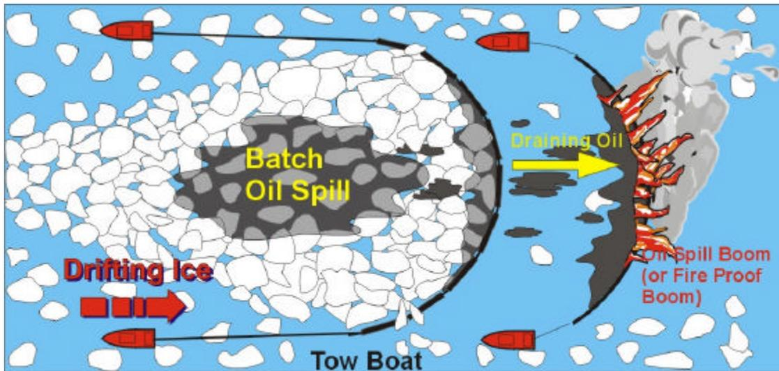
**Figure 3.3: Scenario 2a: A Batch Spill from a Tanker**
