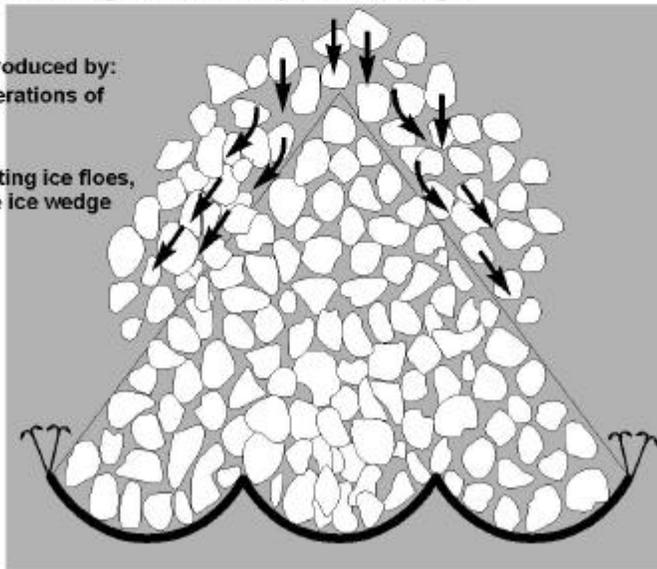
**Figure 4.4: Ice Accumulation and Loading Process in High Pack Ice Concentrations (7-9/10ths)**
