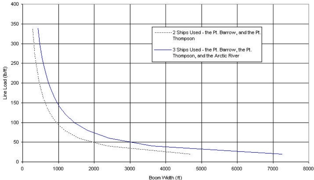
**Figure 6.2: Operating Limits for the Largest Vessels on the North Slope**
