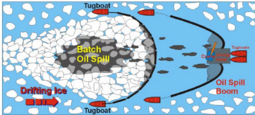
**Figure 3.4: Scenario 2b: A Batch Spill from a Tanker**
