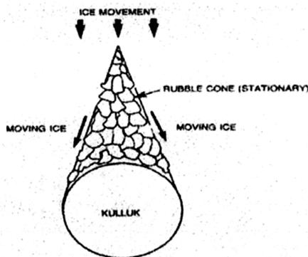
**Figure 5.21** The upper photo provides a representative example of poor ice clearance in “tight” pack ice conditions around the Kulluk. In this situation, the managed ice fragments are not clearing well, and a “rubble wedge” can be seen updrift of the Kulluk. The lower figure is a schematic illustration of this situation.
