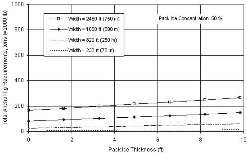
**Figure 4.16: Total Anchoring Requirements for a Pack Ice Concentration of 50% With No Pressure**
