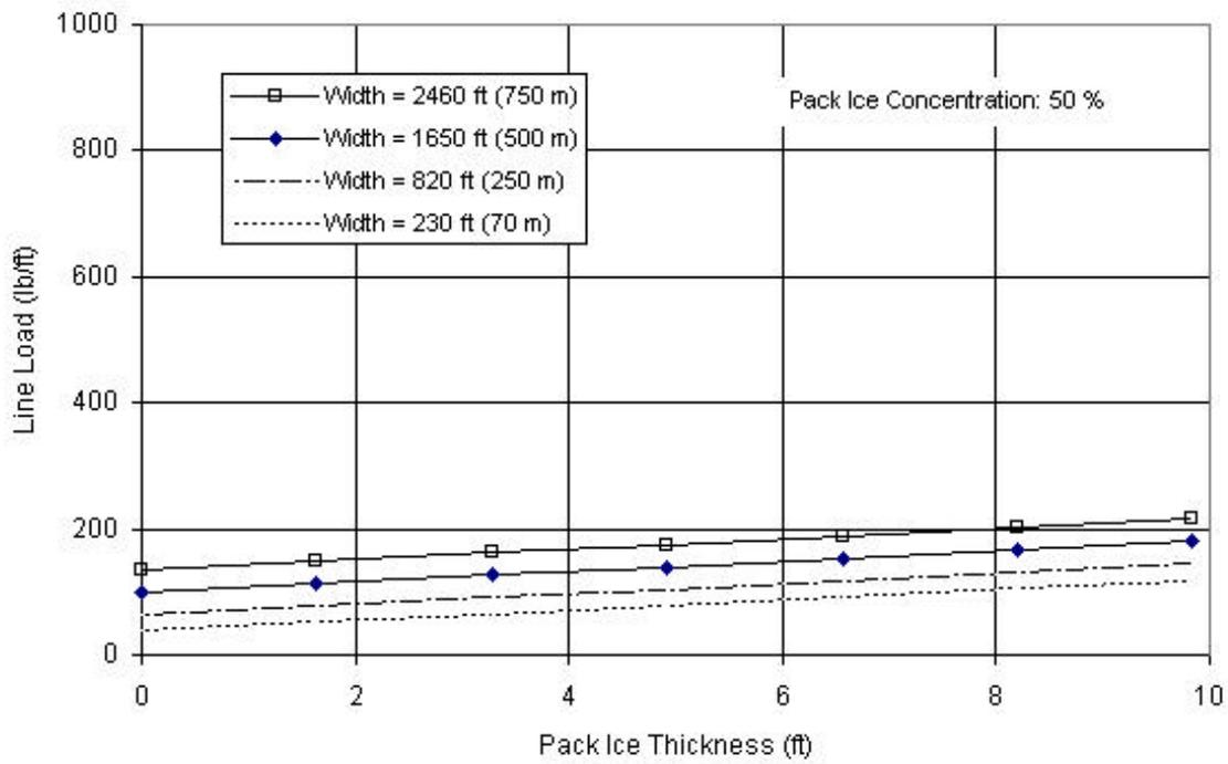
**Figure 4.13: Line Loads for a Pack Ice Concentration of 50% with No Pressure**
