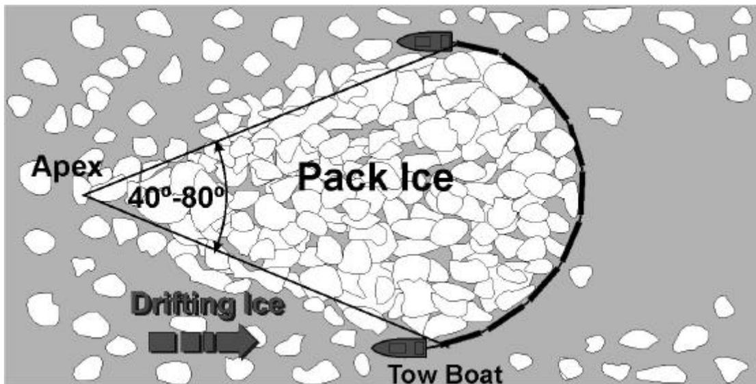
**Figure 4.1: “Dead Wedge” Formed Upstream of a Boom in an Open Sea**
