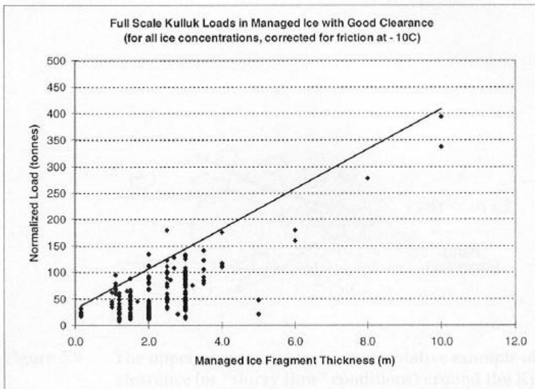
**Figure 4.9: Ice Loads on the Kulluk in Managed Ice Conditions with Good Ice Clearance and No Pressure**
