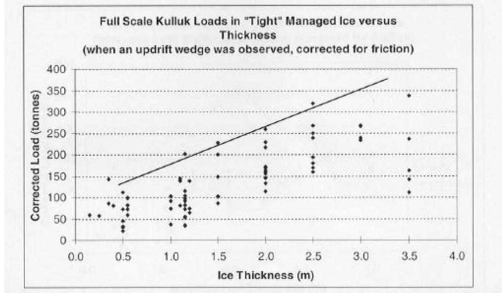
**Figure 4.10: Ice Loads on the Kulluk in Tight Managed Ice Conditions with Poor Ice Clearance and No Pressure**
