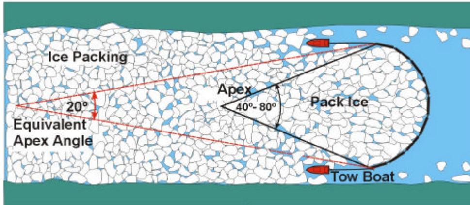
**Figure 4.2: “Dead Wedge” Formed Upstream of a Boom in a Channel**
