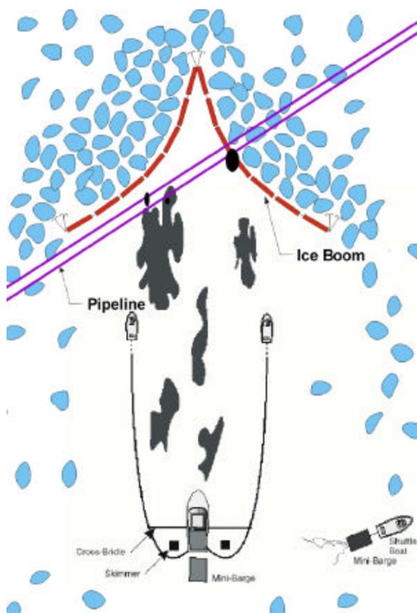
**Figure 3.6: Scenario 3: Continuous Spill from a Punctured Offshore Pipeline**
