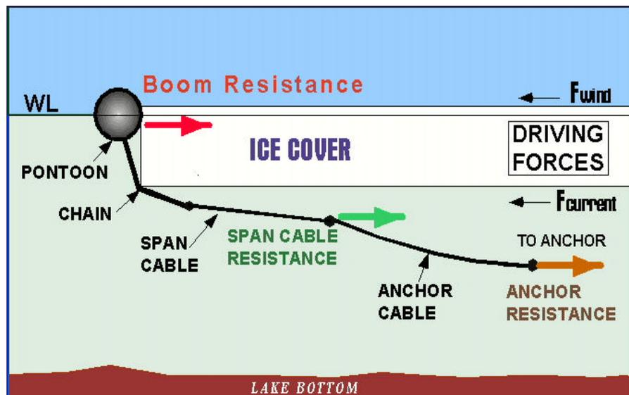
**Figure 5.5: Schematic of Forces Acting on the Boom**
