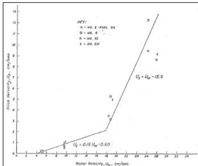
**Figure 3.5: Oil Slick Velocity Versus The Current Velocity (after Cox et al, 1980)**
