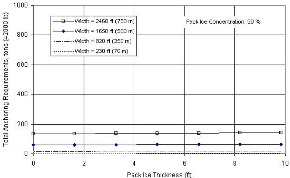
**Figure 4.15: Total Anchoring Requirements for a Pack Ice Concentration of 30% With No Pressure**
