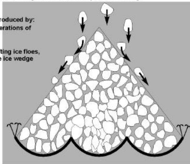
**Figure 4.3 Ice Accumulation and Loading Process in Pack Ice Concentrations up to about 8/10ths**
