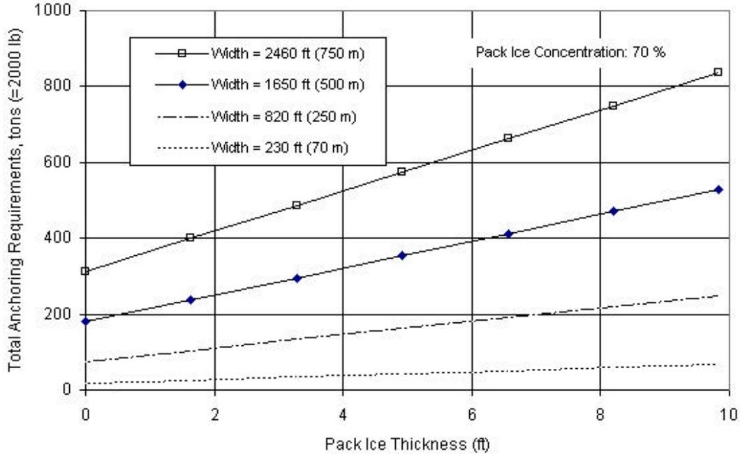
**Figure 4.17: Total Anchoring Requirements for a Pack Ice Concentration of 70% With No Pressure**
