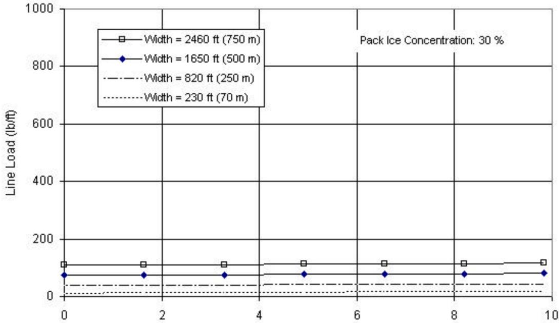
**Figure 4.12: Line Loads for a Pack Ice Concentration of 30% with No Pressure**
