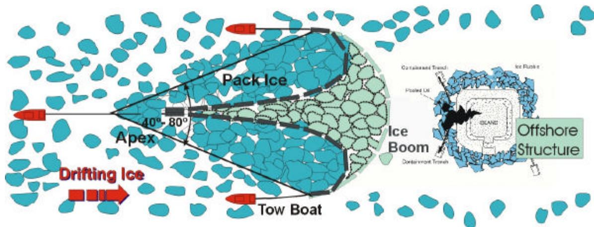
**Figure 5.1: The Deployment of an Ice Boom in two Configurations (i.e., Chevron and Catenary), Upstream of an Oil-Spill from an Offshore Structure**
