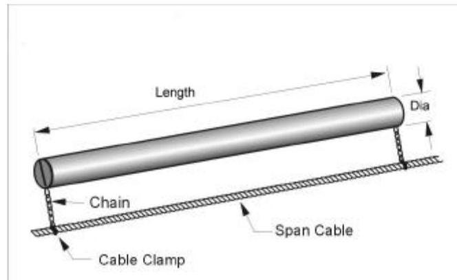
**Figure 5.3: Pontoon Attached to the Span Cable to Allow Ice Over-Run when the Ice Load Exceeds the Boom's Ice Retention Capacity**
