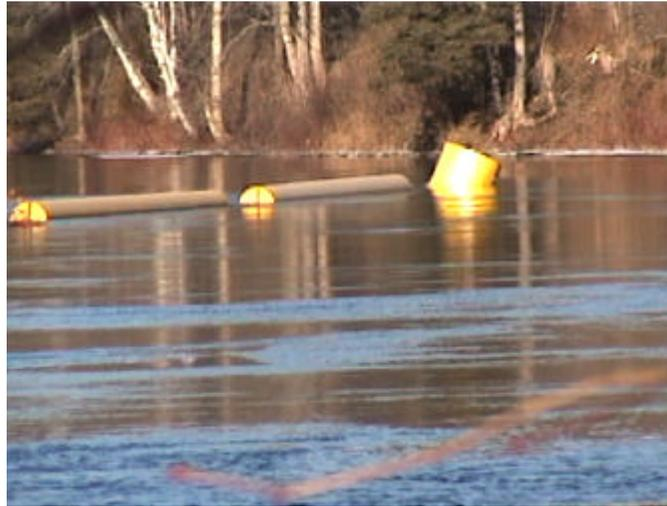
**Figure 5.4: Buoy Used to Connect the Tugboat or the Anchor to the Boom**
