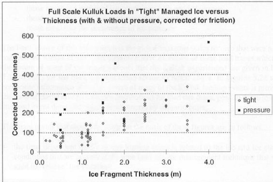
**Figure 4.11: Effect of Pressure on the Loads Exerted on the Kulluk**
