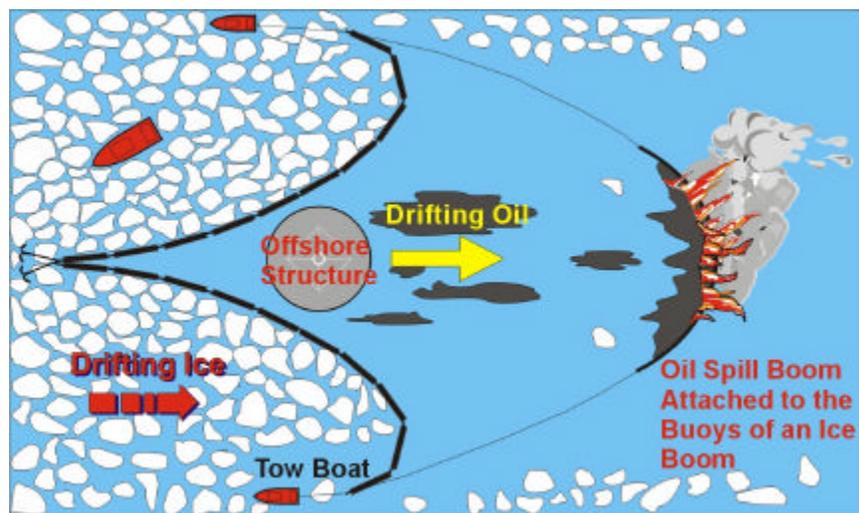
**Figure 5.2: Boom Maneuvering and Attachment of an Oil Spill Boom to an Ice Boom.**
