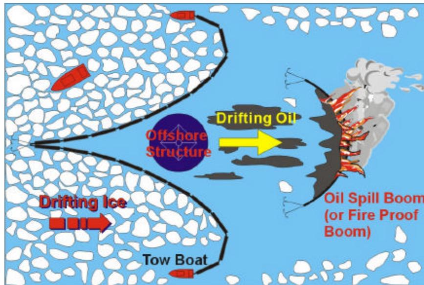
**Figure 3.2: Scenario 1b: Oil-Spill From An Offshore Structure**
