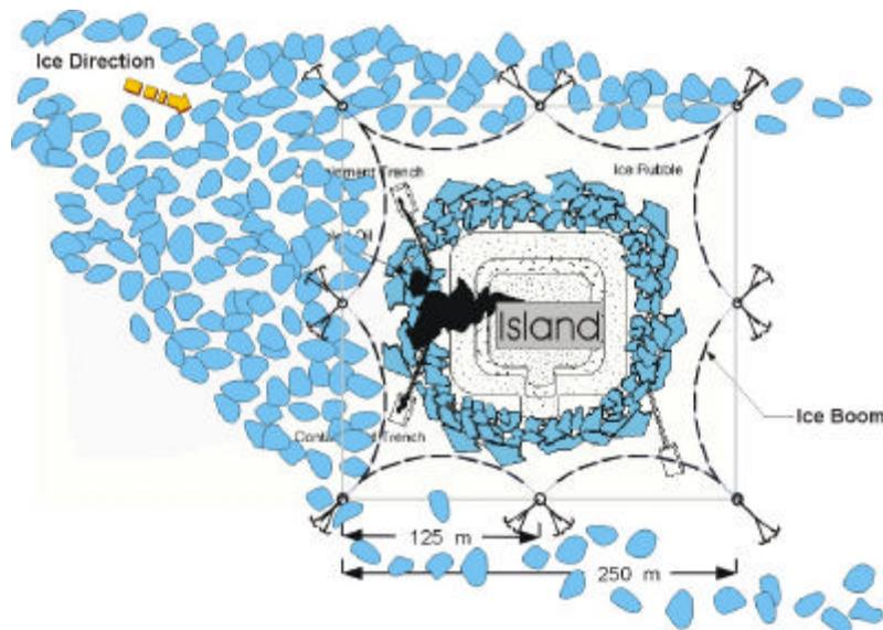
**Figure 5.8: Fixed Boom Installation**
