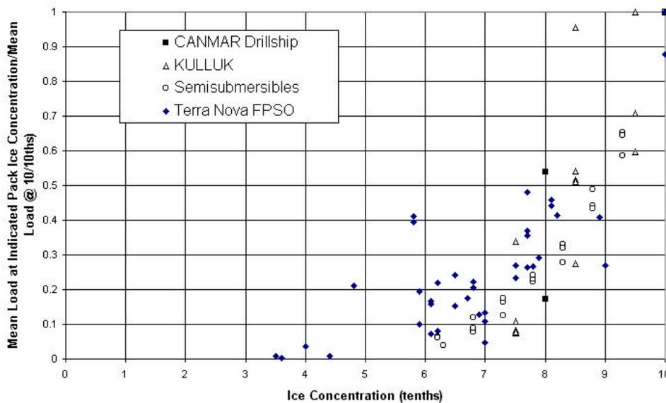
**Figure 4.8: Effect of Pack Ice Concentration on Pack Ice Loads**
