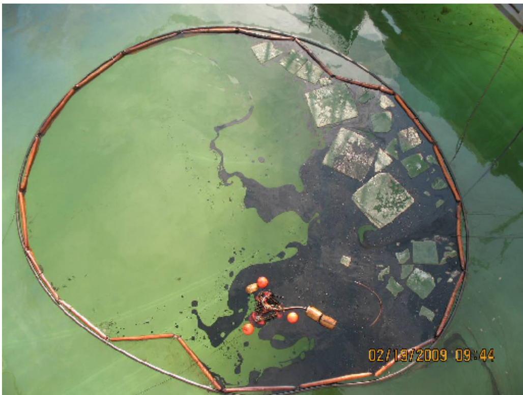
Figure 10: Photograph of same disc skimmer test from man lift after herder applied to slick.
