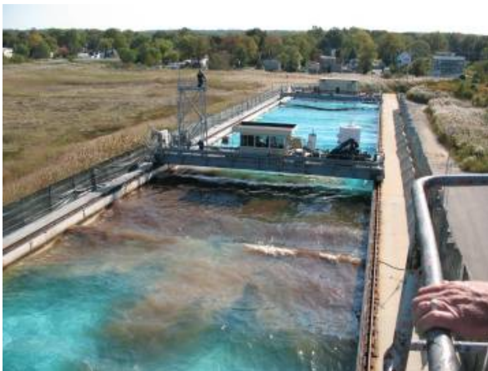
Figure 25. Main Bridge towing LISST and C3 through dispersed oil cloud.
