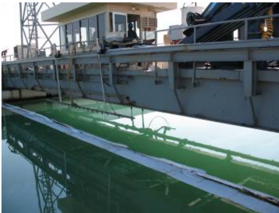
Figure 18. Dispersant spray bar mounted on trolley on north side of Main Bridge. Note sorbent sweep below Bridge.
