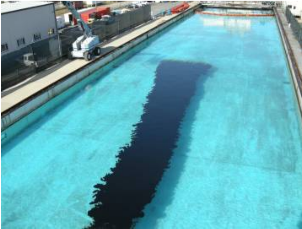
Figure 20. Slick spreading before herder application
