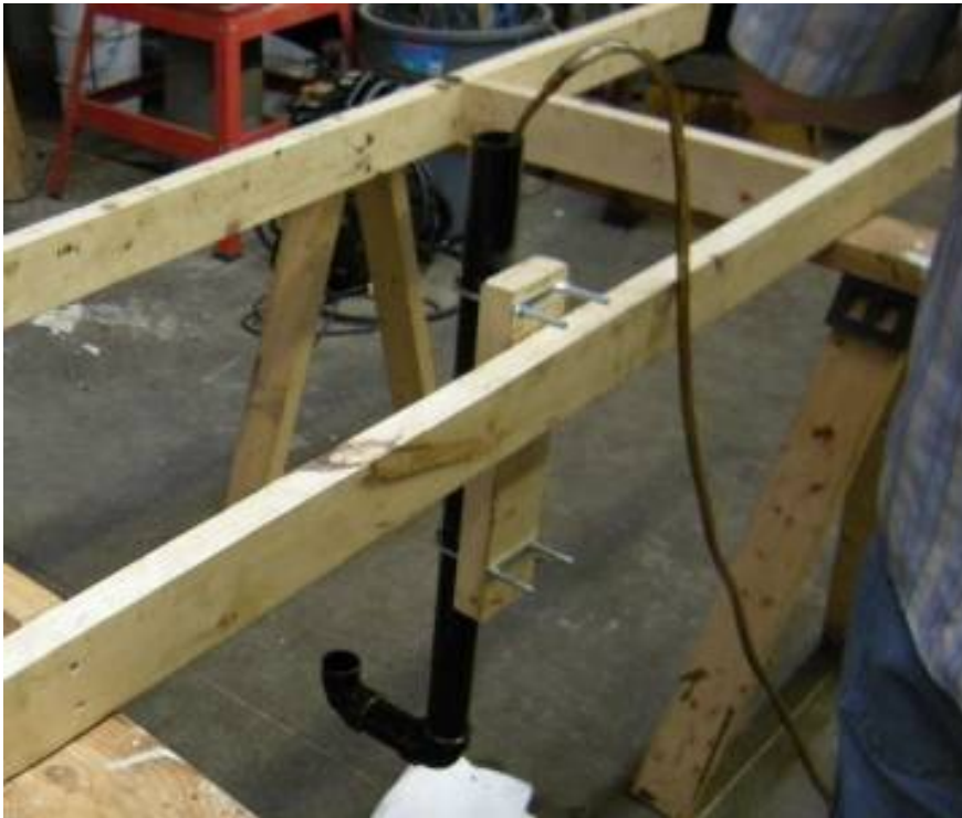
Figure 3: Surrogate weir skimmer used in tests.
