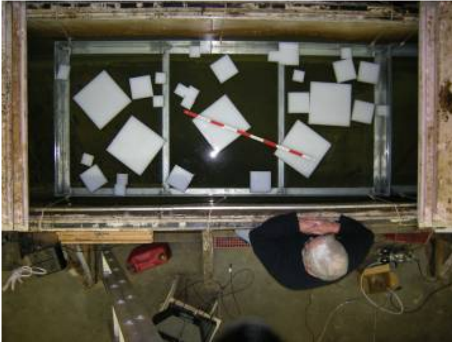
Figure 2: Test section in SL Ross wind/wave tank containing artificial ice floes made from 1''-thick LDPE.
