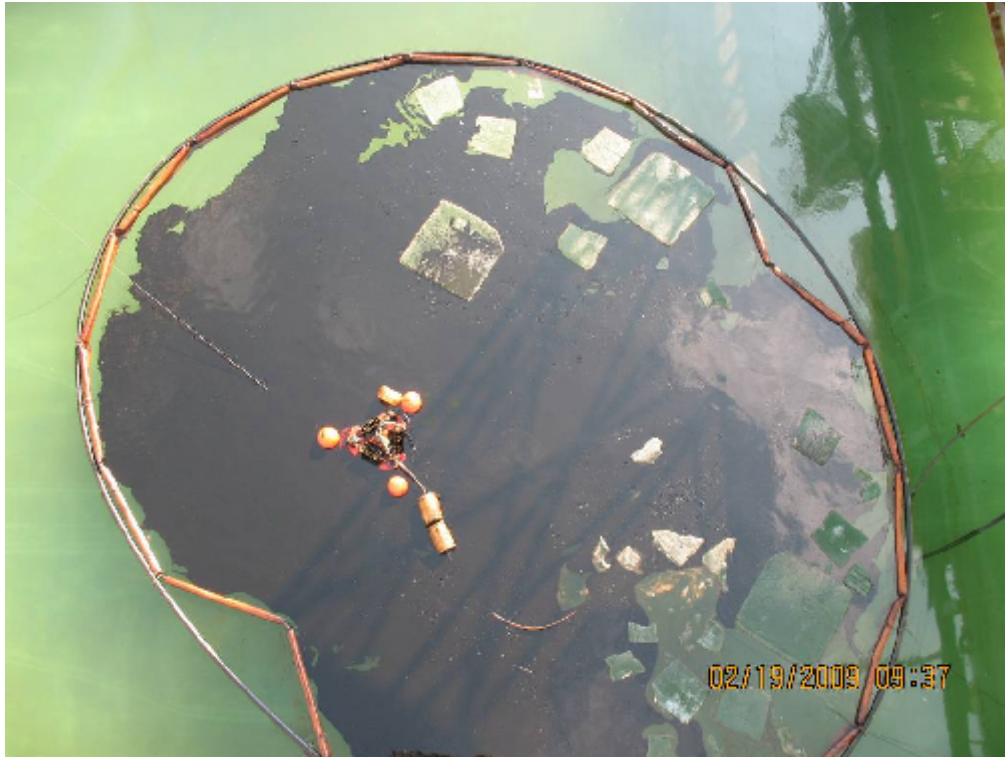
Figure 9: Photograph of disc skimmer test with 10% ice from man lift prior to herder.
