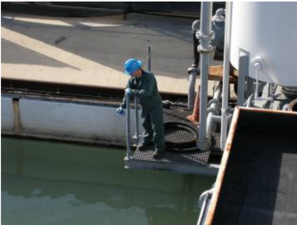
Figure 21. Applying herder from handheld spray bottle.
