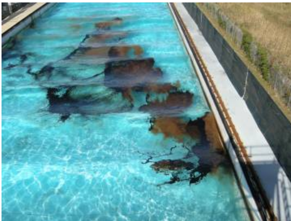
Figure 24. Dispersion underway as cresting waves create small droplets.
