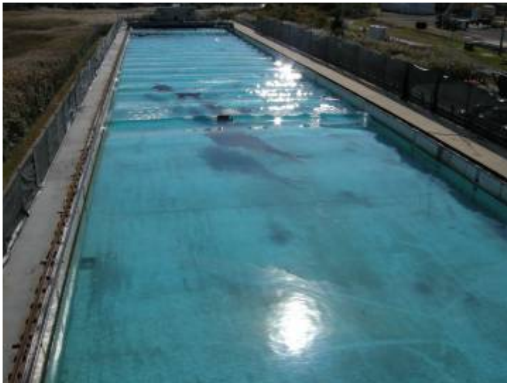
Figure 23. Waves just hitting herded slick after dispersant applied.
