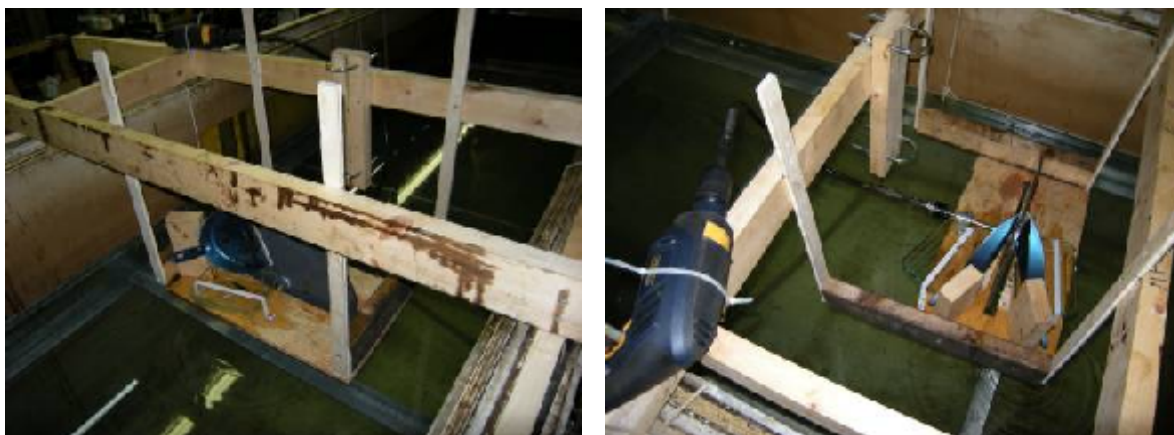
Figure 4: Mock disc skimmer used in tests.
