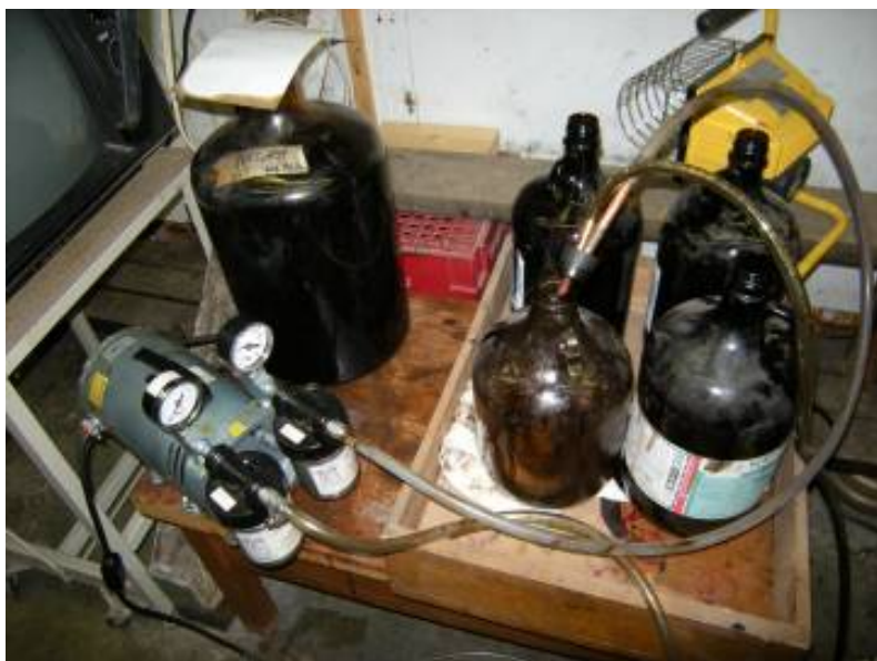
Figure 6: Vacuum pump and glass bottles used to collect recovered oil from skimmers.
