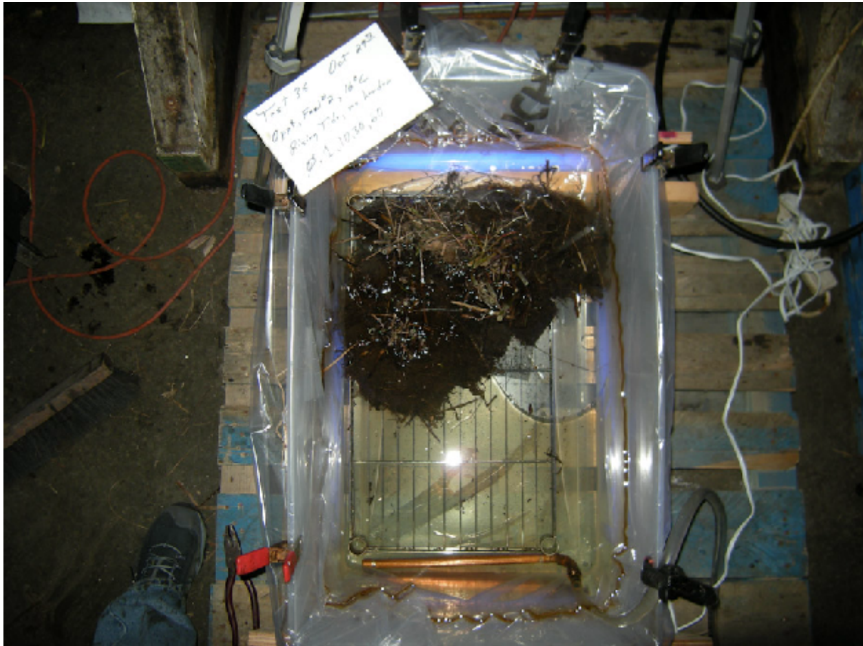
Figure 16. “Rising Tide” test apparatus. Note copper pipe water diffuser at low end and marsh plants at high end of pan.
