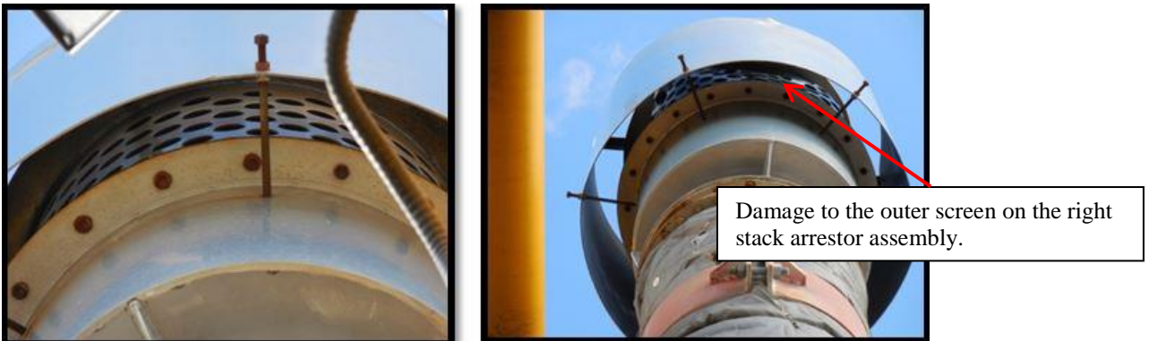
Figure 17: Comparison of Left and Right Stack Arrestor Assemblies
