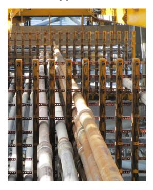
Figure 3- Looking upward from the deck. In the foreground is the lower fingerboard. Latches in closed position can be seen holding stands of pipe in place.
