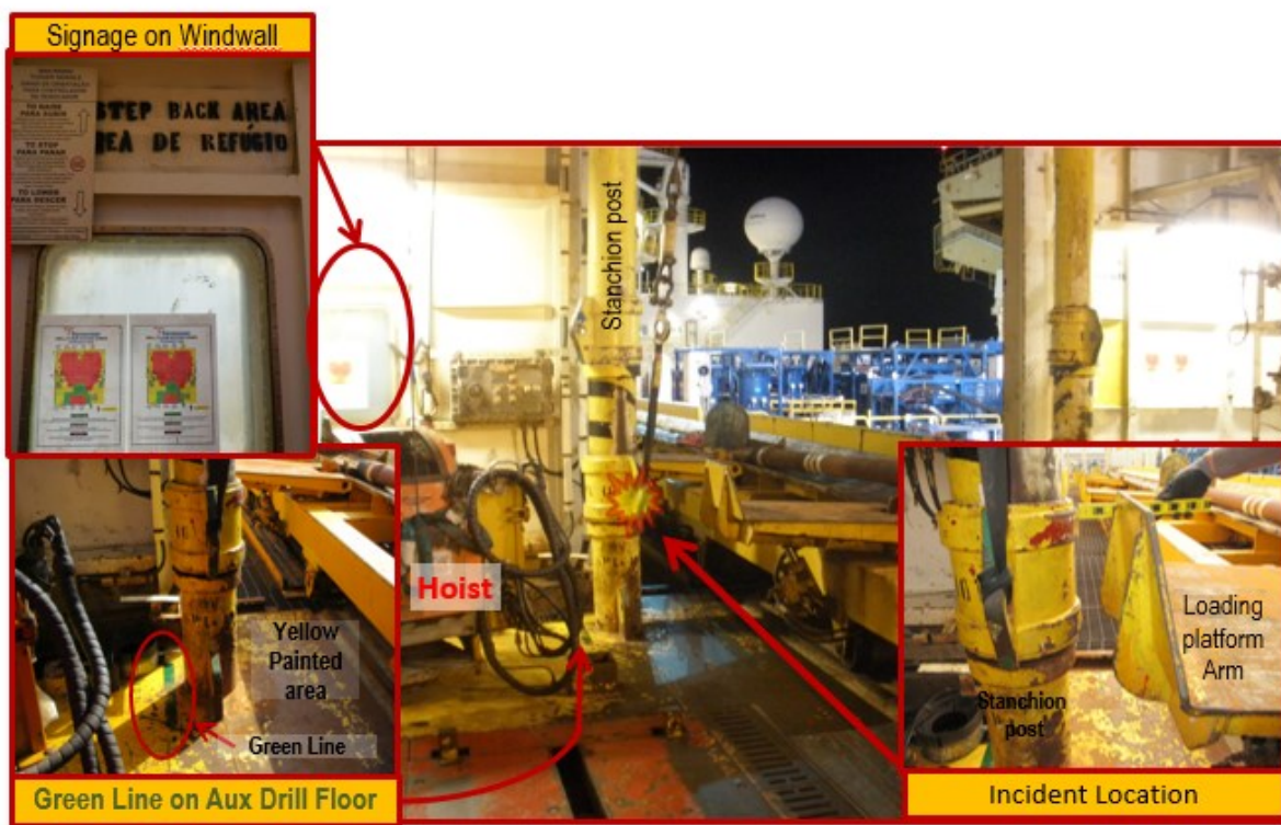
Figure 12: Auxiliary drill floor loading platform arm/ stanchion post proximity (floor hand view)
