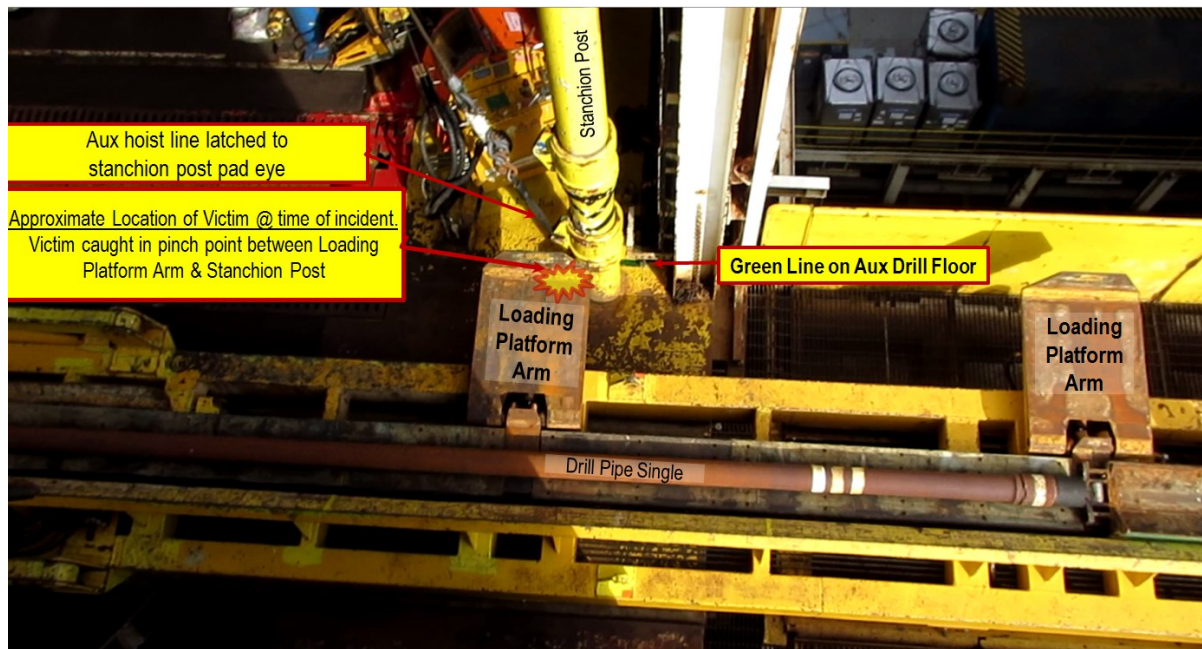
Figure 16: Auxiliary drill floor loading platform arm/ stanchion post proximity - birds-eye view #1 (BSEE photo)
