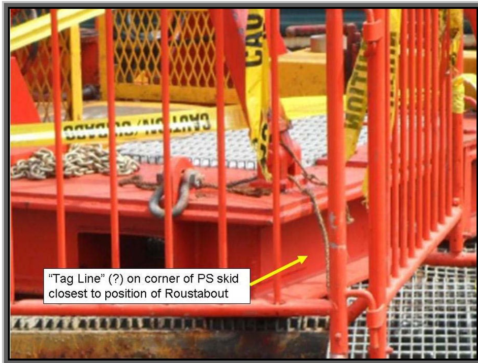
Figure 13 – Original tag lines on power swivel, Roustabout corner
