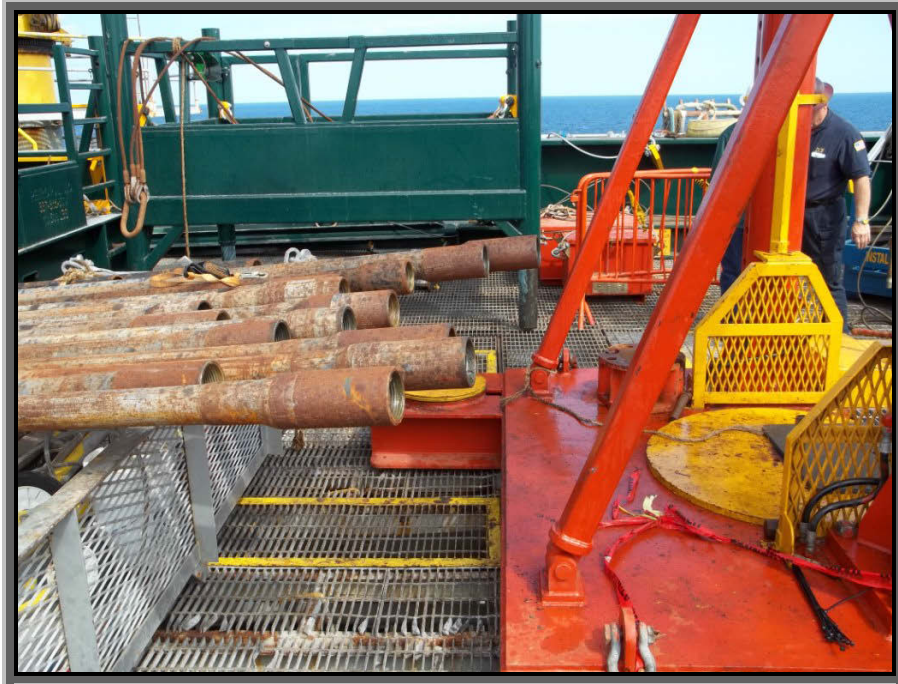
Figure 15 – Pipe in “pipe rack” overhanging PS skid
